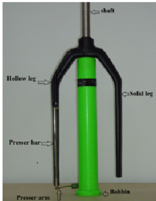
Figure 1.2: Structure of flyer (Courtesy : Inspiron Engg. Pvt. Ltd.)
