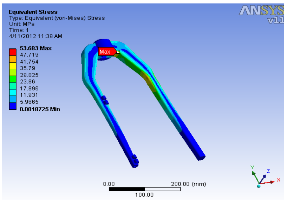
Figure 6.6: Von-Mises Stress on optimized balanced model of flyer
