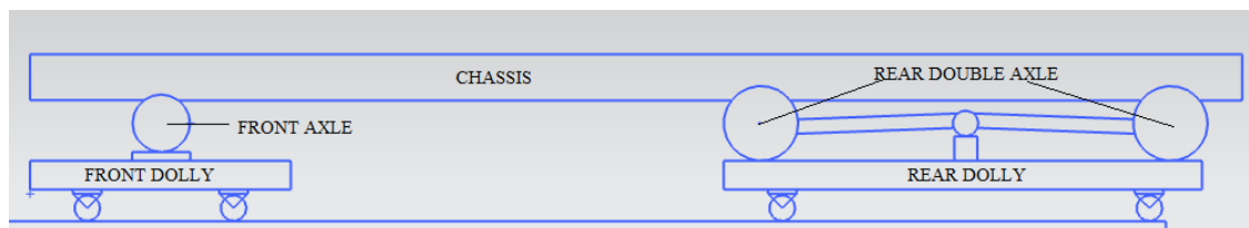
Figure 3.1: Arrangement of the Axles on the Front and Rear Dolly
