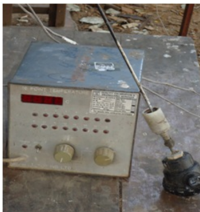
Figure 3.1: 12-point digital Temperature indicator with thermocouple.
