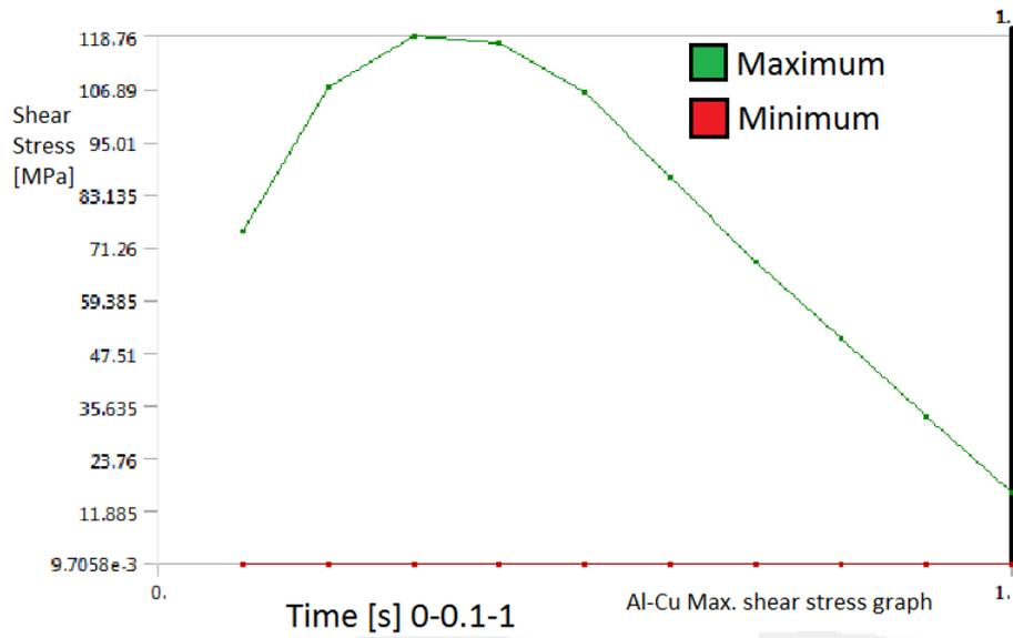
Figure 5.21: Transient shear stress graph for lathe bed of Al-Cu alloy
