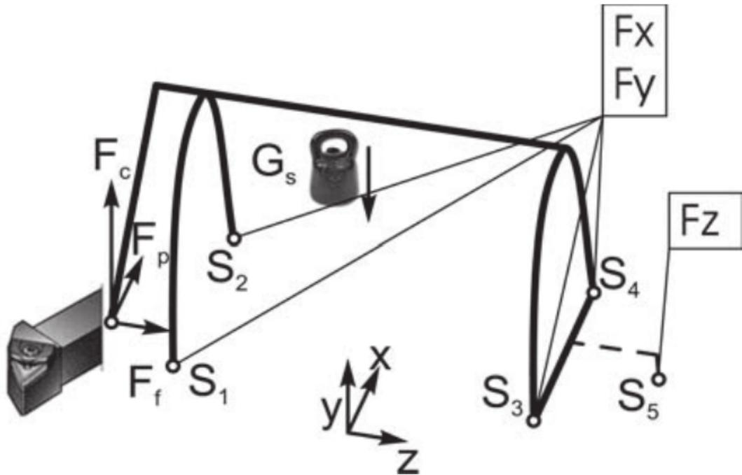
Figure 2.3: A diagram to determine reaction forces and moments of the slide[2]
