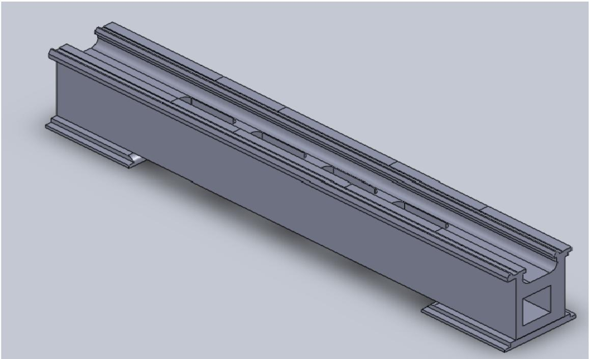
Figure 4.14: New optimized redesigned lathe bed structure
