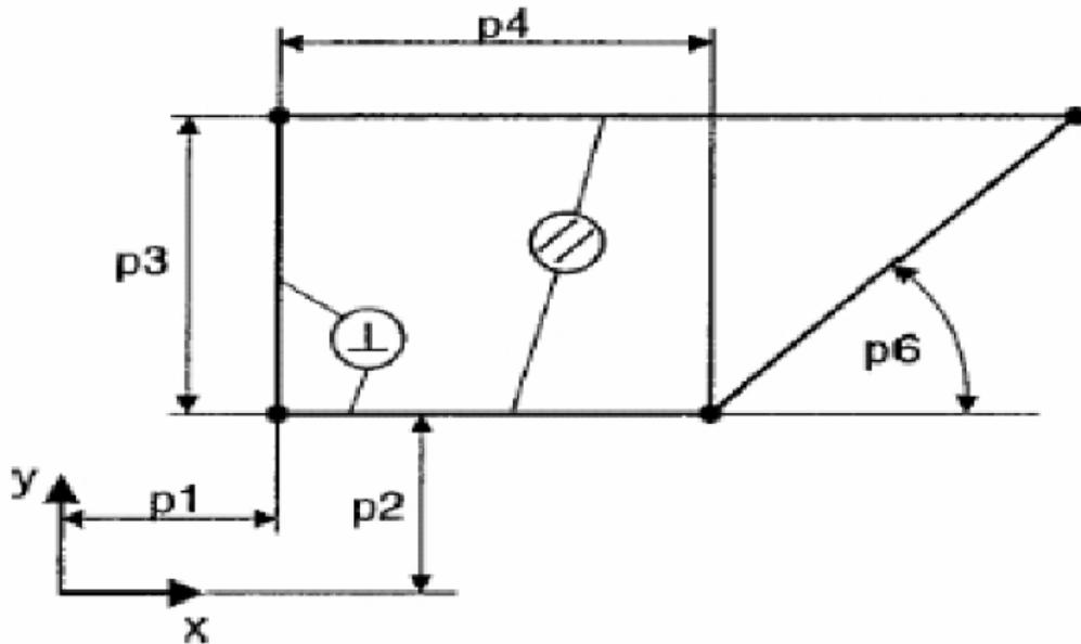
Figure 4.2: Defining Geometry by Parameters
