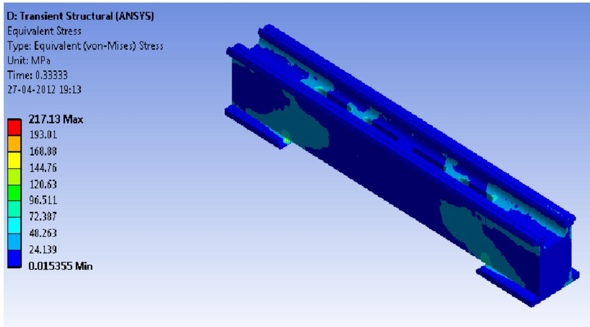
Figure 5.9: Present von-Mises transient stress
