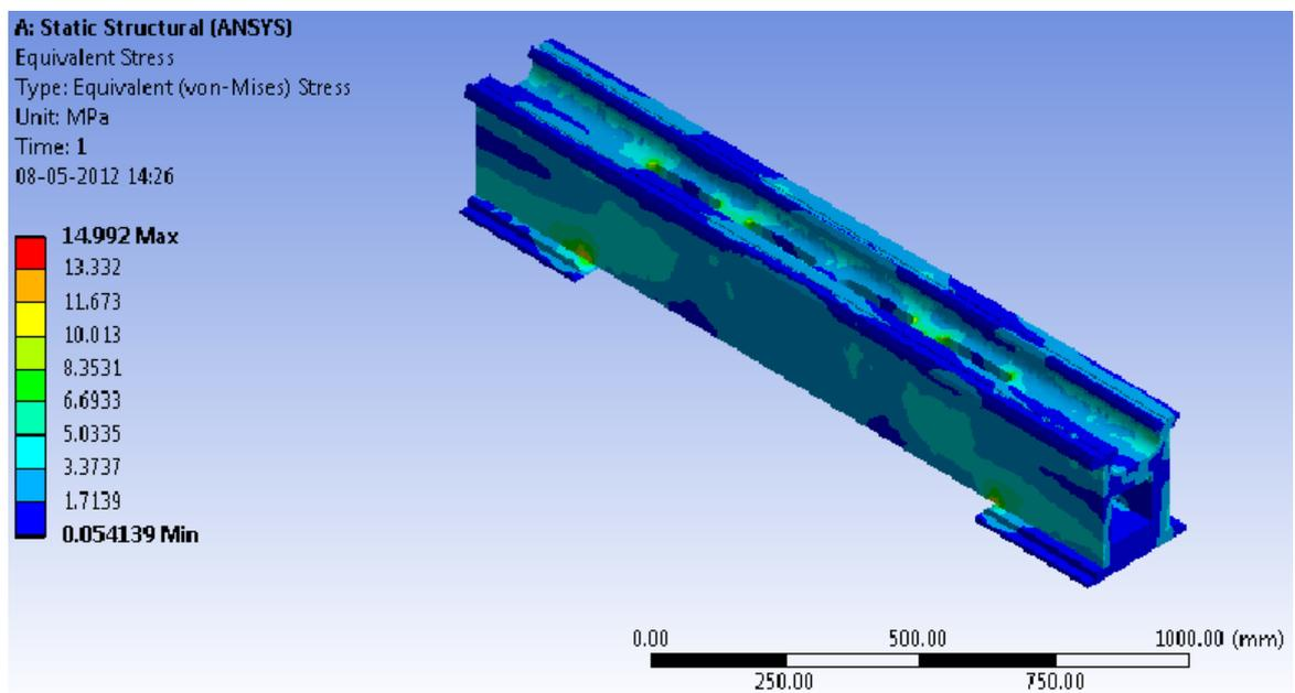
Figure 5.4: Proposed optimized von-Mises static stress
