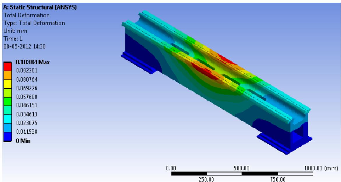
Figure 5.8: Proposed optimized static deformation
