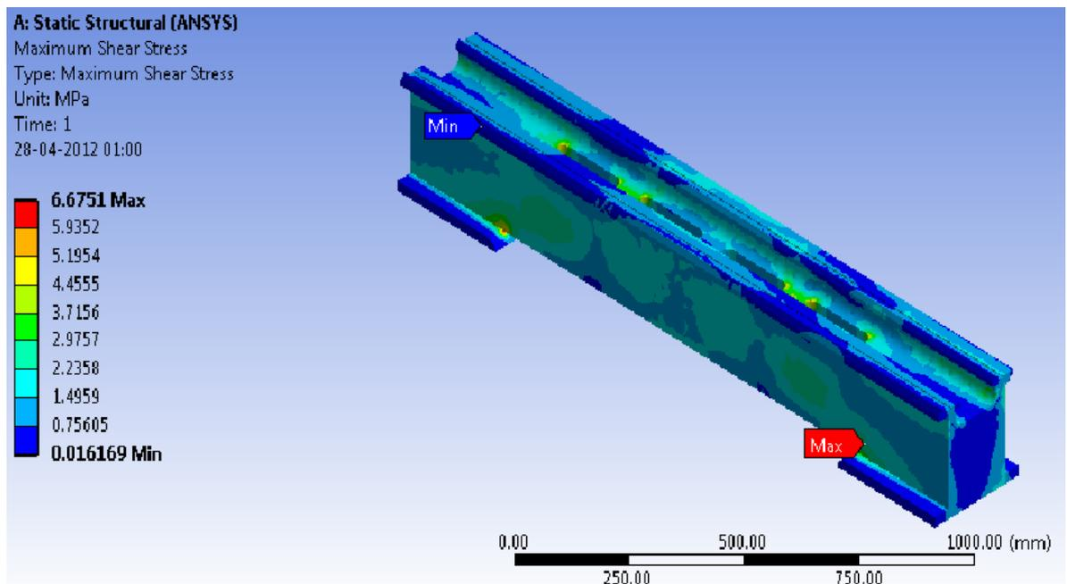
Figure 5.16: Proposed material static shear stress
