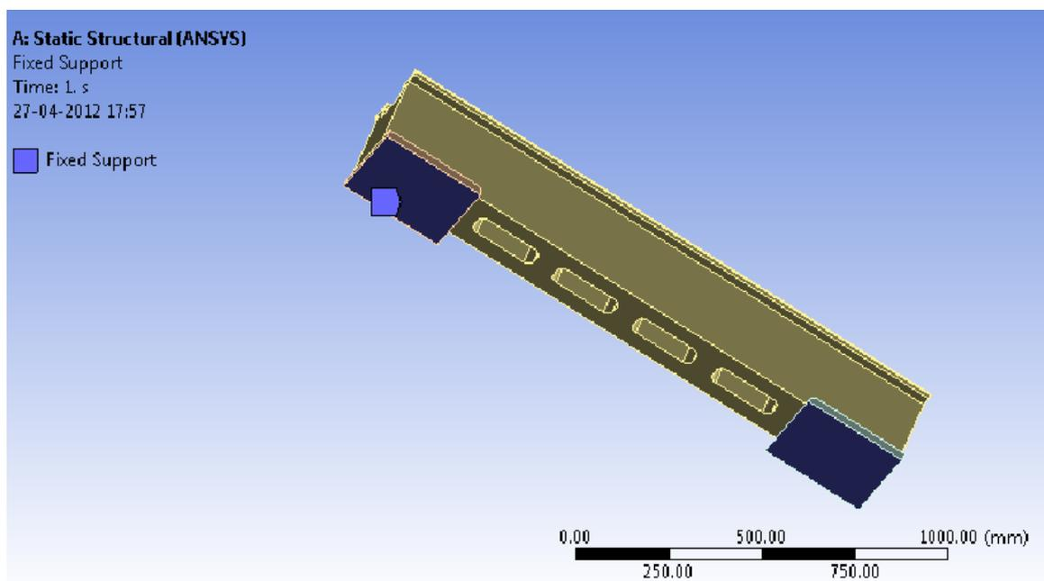
Figure 4.8: Boundary condition applied to support of lathe bed
