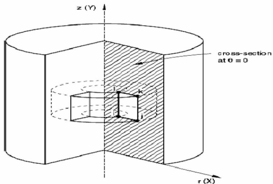
Figure 4.4: Axis symmetric element
