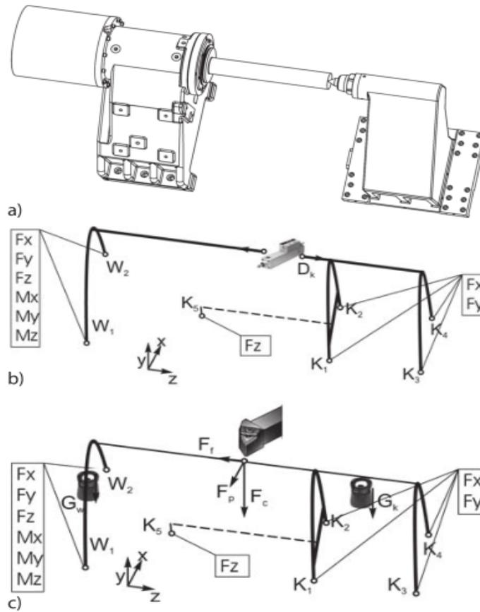
Figure 2.4: A diagram to determine headstock and tailstock force and moment reactions[2]
