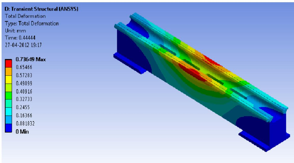
Figure 5.13: Present transient deformation
