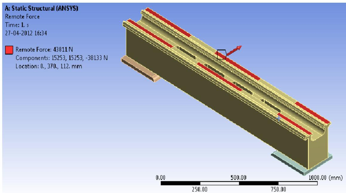
Figure 4.7: Different forces on lathe bed for static analysis
