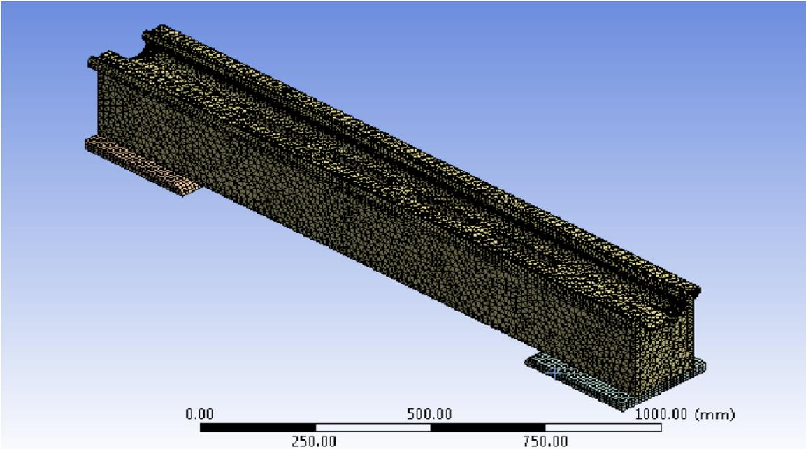
Figure 4.6: Meshed model of lathe bed
