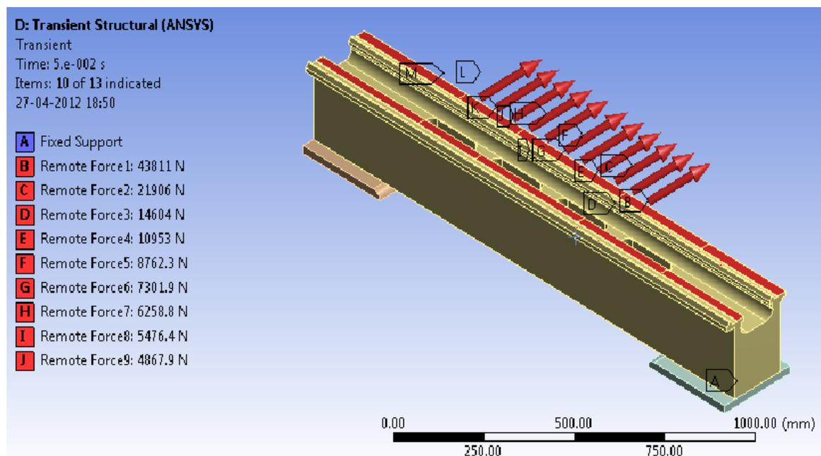
Figure 4.13: Different forces acting on lathe bed for dynamic analysis
