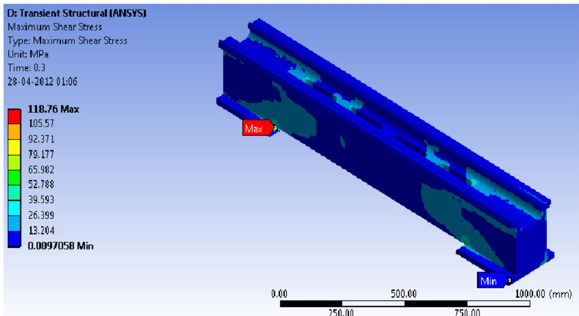
Figure 5.20: Transient shear stress for lathe bed of Al-Cu alloy
