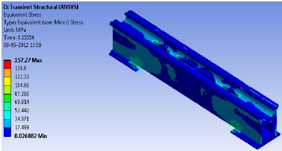
Figure 5.10: Proposed optimized von-Mises transient stress
