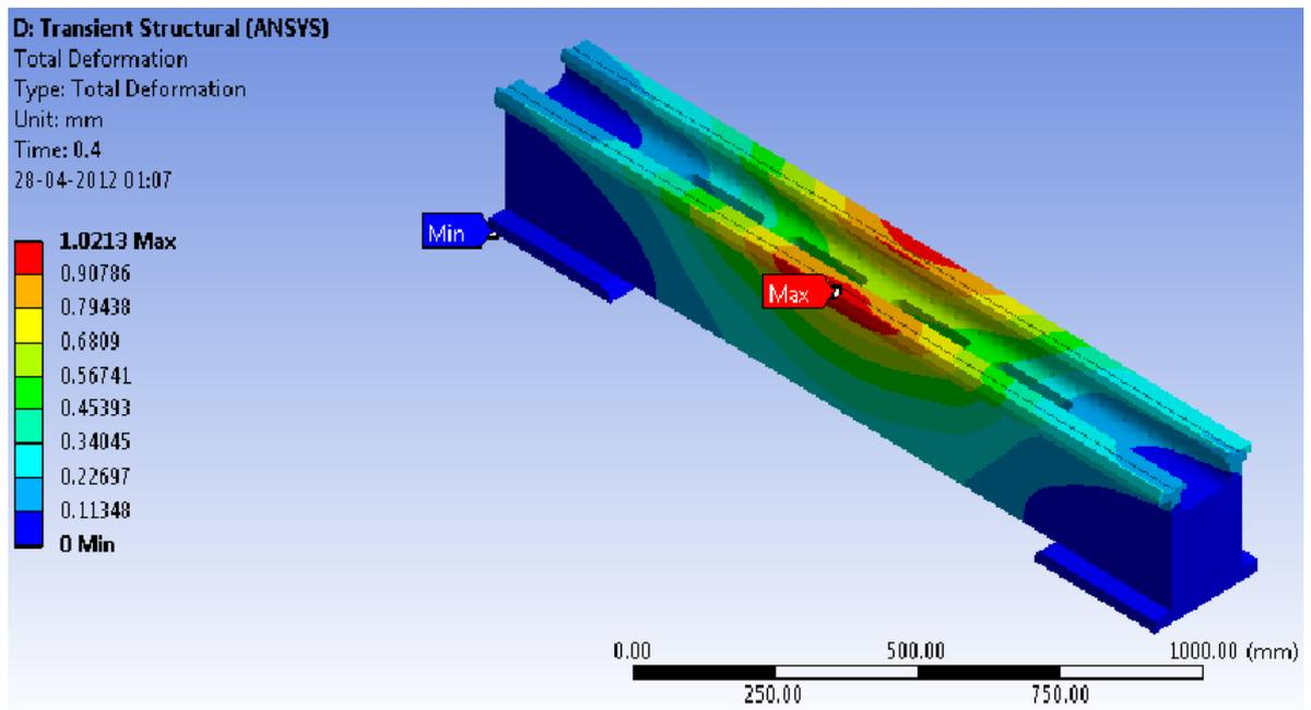
Figure 5.22: Transient deformation for lathe bed of Al-Cu alloy
