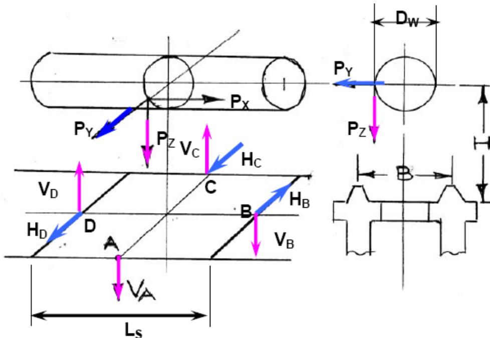
Figure 3.2: Forces acting on lathe bed due to saddle through cutting force[7]
