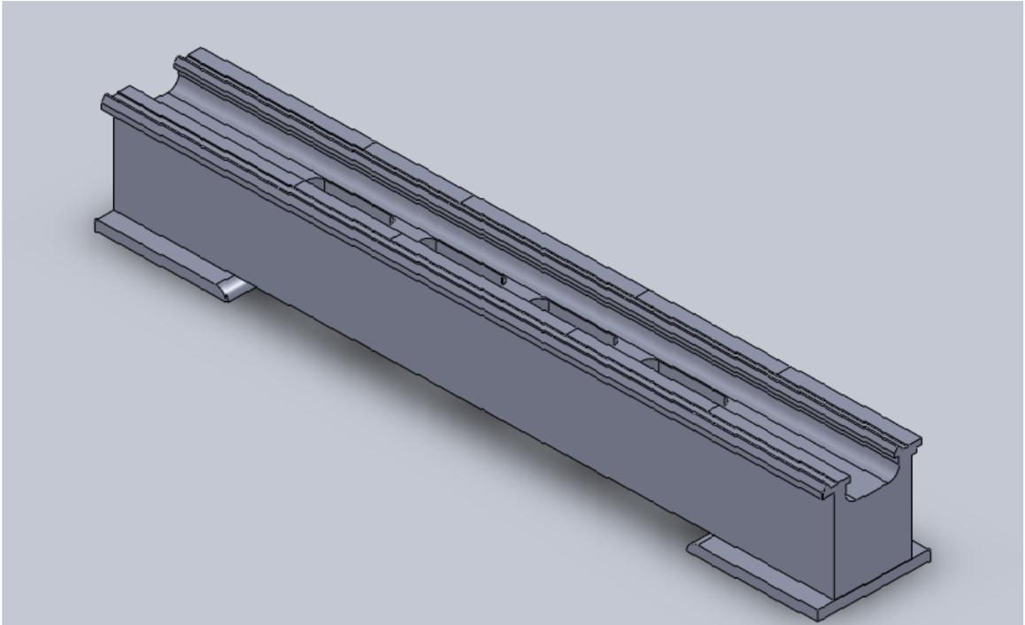
Figure 4.3: Solid modeling of lathe bed
