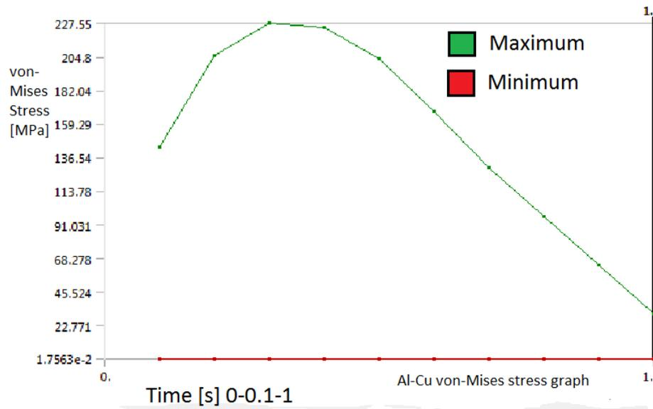
Figure 5.19: Transient von-Mises stress graph for lathe bed of Al-Cu alloy
