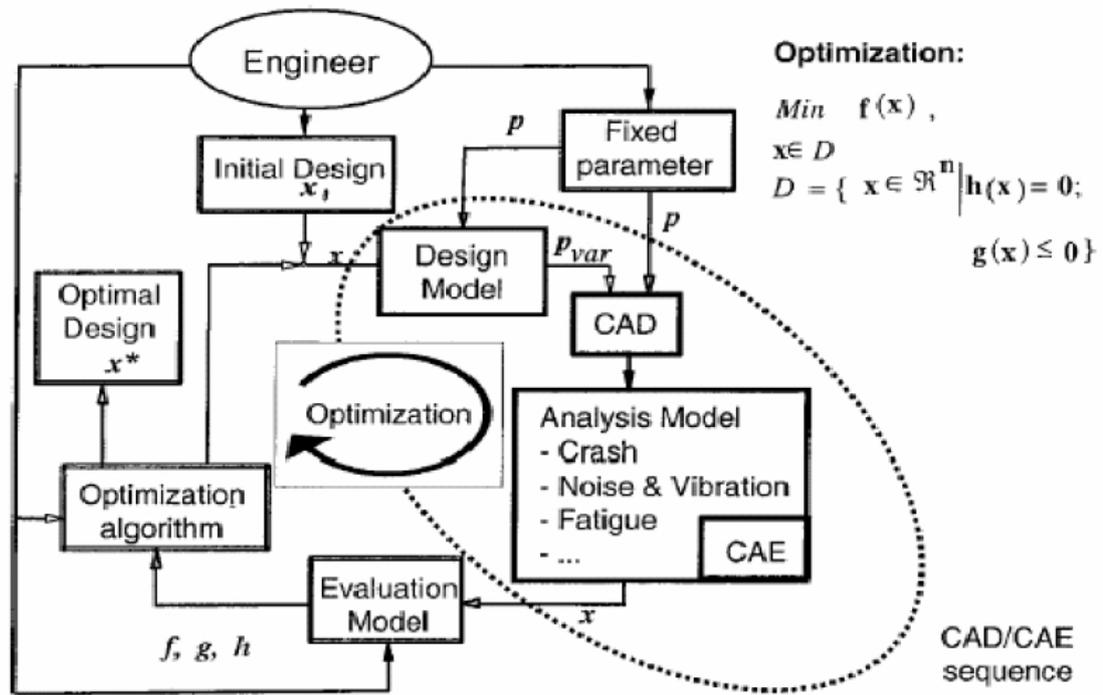
Figure 4.1: CAD/CAE sequence within the optimization process
