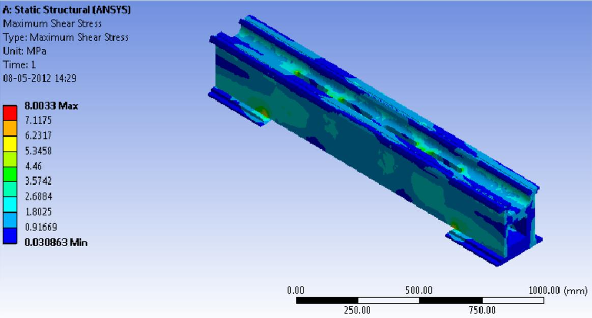
Figure 5.6: Proposed optimized shear static stress
