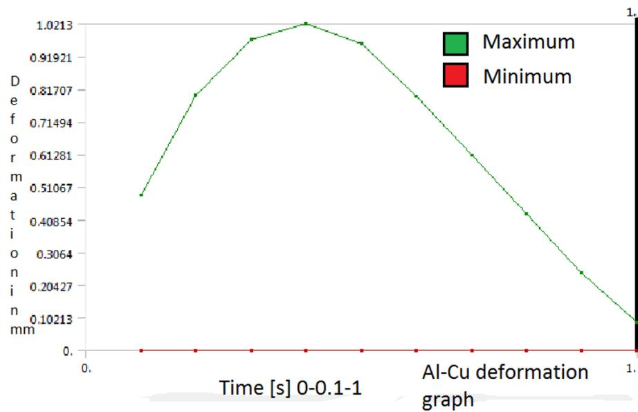
Figure 5.23: Transient deformation graph for lathe bed of Al-Cu alloy
