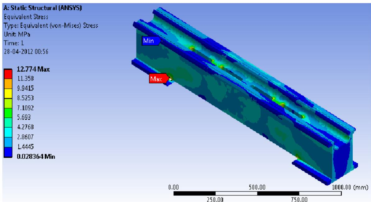
Figure 5.15: Proposed material static von-Mises stress
