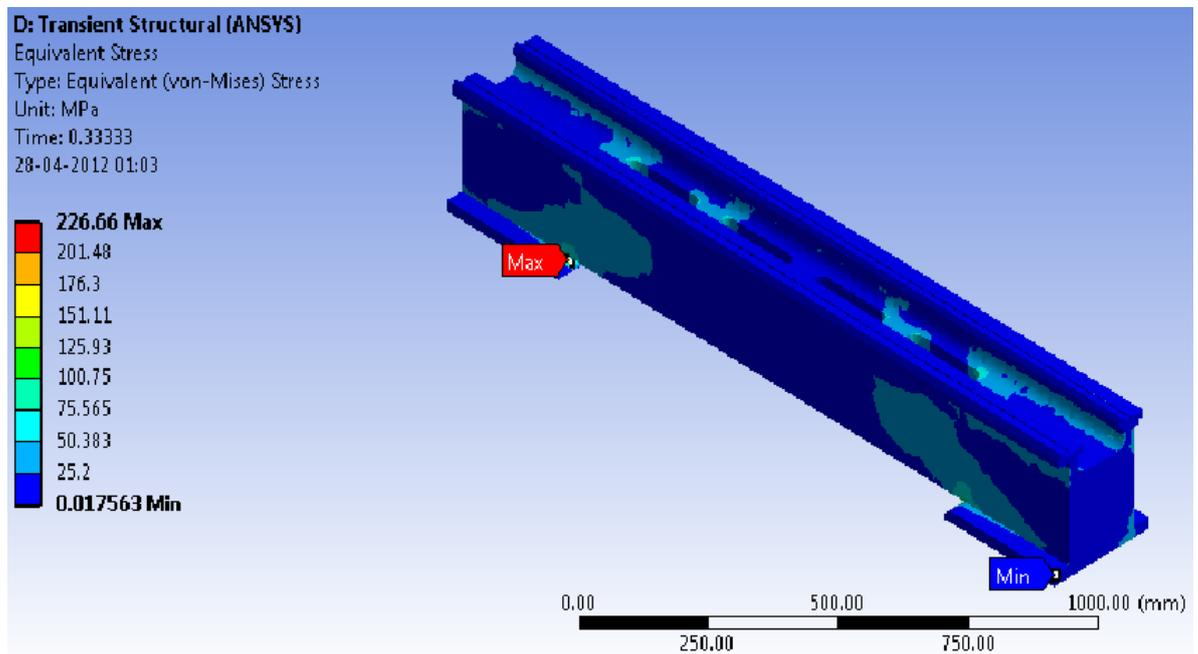
Figure 5.18: Transient von-Mises stress for lathe bed of Al-Cu alloy
