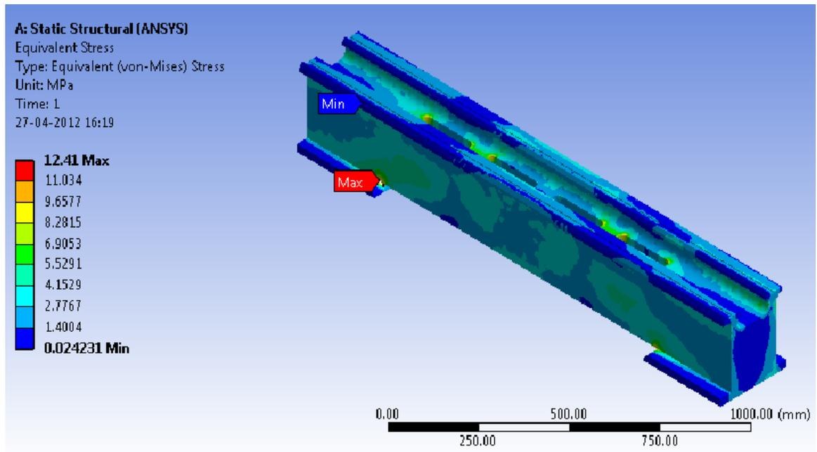
Figure 5.3: Present von-Mises static stress
