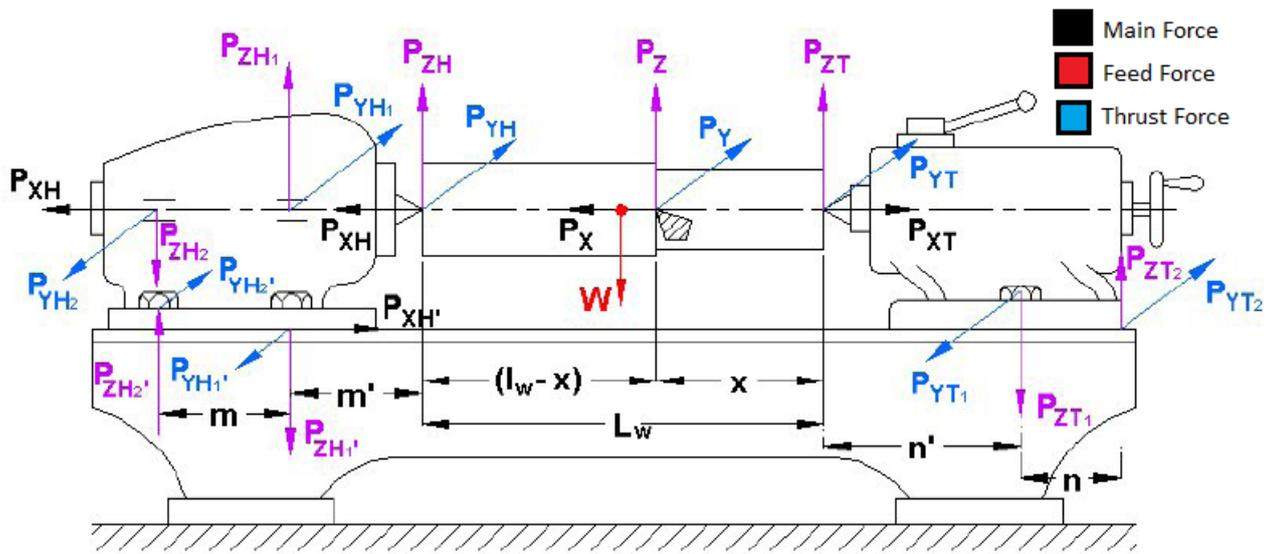
Figure 3.1: Forces acting on lathe[7]
