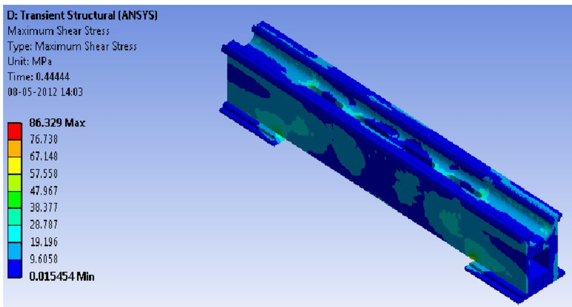
Figure 5.12: Proposed optimized shear transient stress
