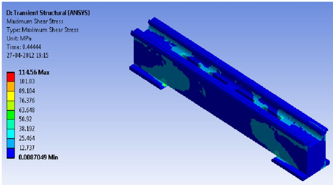
Figure 5.11: Present shear transient stress
