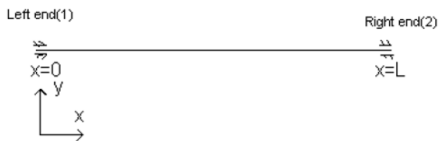
Figure 3.2: Intermediate span of tube(pinned-pinned)
