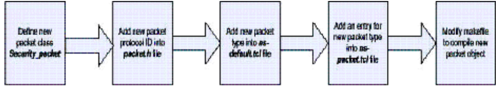
Figure 6.1: Flow chart of adding new protocol to NS-2
