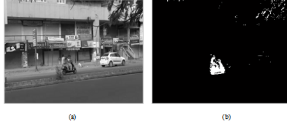
Figure 7.6: Result of background subtraction (a) video frame containing stationary and moving object both, (b) thresholded image
