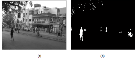
Figure 7.3: Result of background subtraction (a) video frame in which car has moved out, (b) thresholded image
