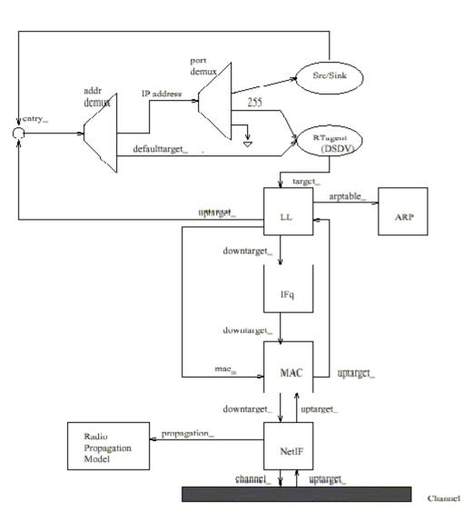
Figure 3.2: Model of Basic Wireless mobile node[7]
