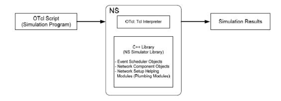
Figure 3.1: Basic Structure Of Ns-2[7]
