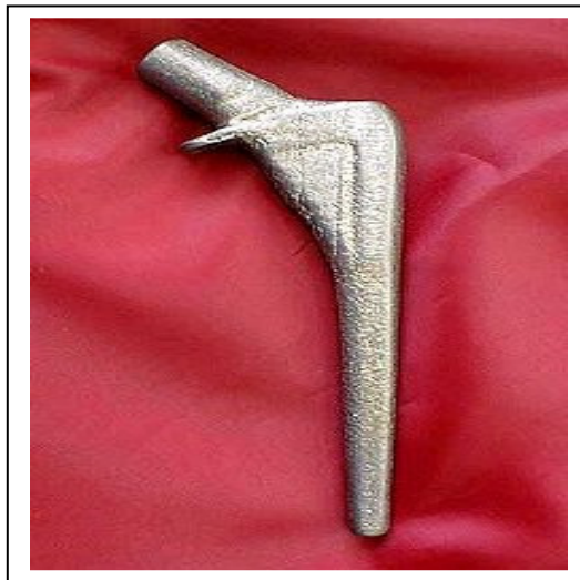
Fig 5: Titanium hip implant made by Laser Engineered Net Shaping
