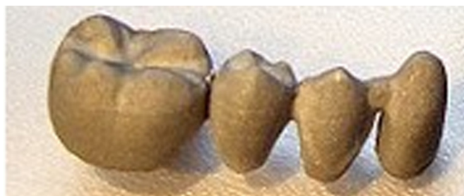
Fig.4 –bridge by DMLS
