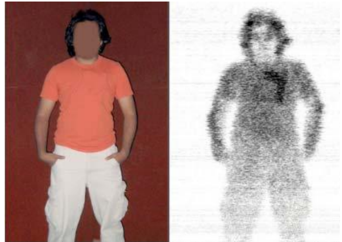
Figure 4. THz reflection image of a person carrying a gun[9]
