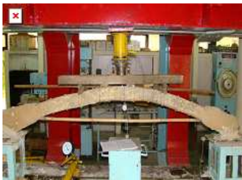
(b) Bamboo concrete composite infill parabolic tied arch: Centre Half Loading
