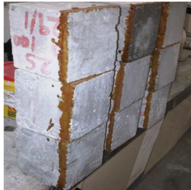
Figure 3.15: Sealed specimens prepared for sorptivity test
