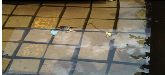
Figure 3.11: Tank of chloride solution with concrete specimens
