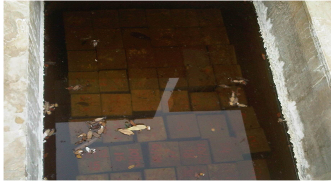
Figure 3.9: Tank of sulfate solution with concrete specimens
