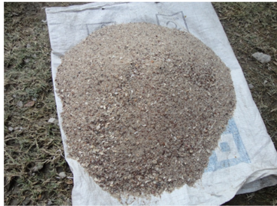
Figure 1.1: Dredged marine sand
