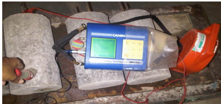
Figure 3.24: Half-cell potentiometer test on RC specimens
