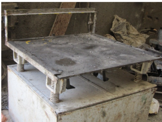
Figure 3.3: Table vibrator for compacting concrete mix
