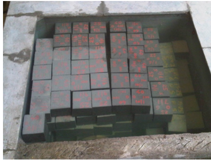
Figure 3.4: Curing of plain concrete specimens
