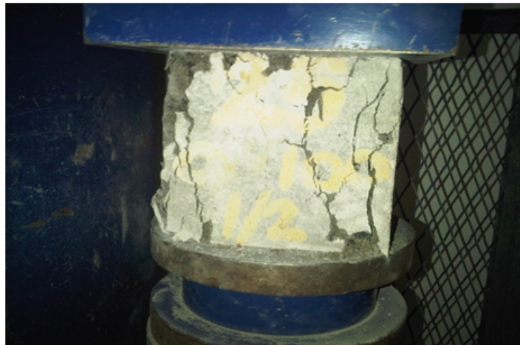
Figure 3.6: Plain concrete cube in compression testing machine
