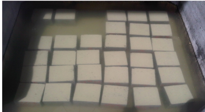
Figure 3.18: Concrete specimens in water tank for water absorption test
