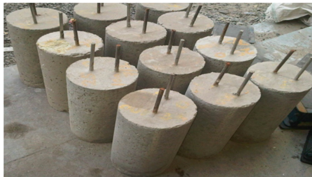
Figure 3.20: Specimens for accelerated corrosion test
