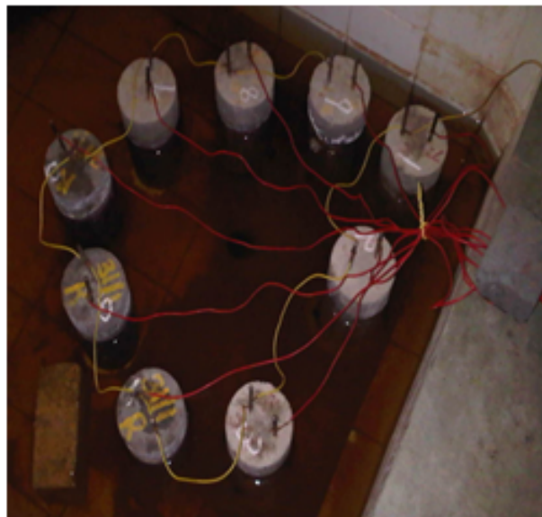
Figure 4.12: RC specimens after initiation of corrosion in the reinforcement
