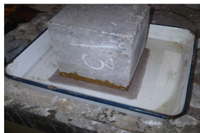
Figure 3.16: Sealed cube on bunch of filter papers for sorptivity test
