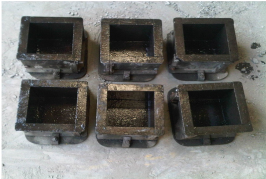
Figure 3.1: Moulds for concrete specimens
