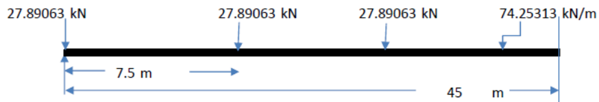
Figure 4.22: Final DL Loading on Girder
