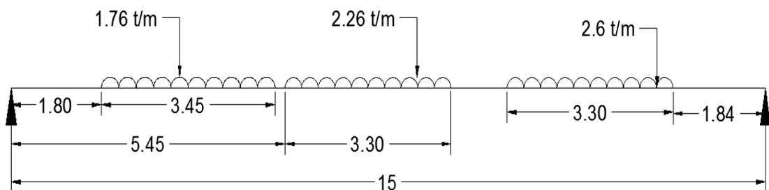
Figure 4.12: Effective UDL for maximum forces
