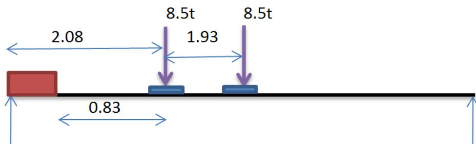
Figure 4.4: Transverse placement of 17t(Q) Axles
