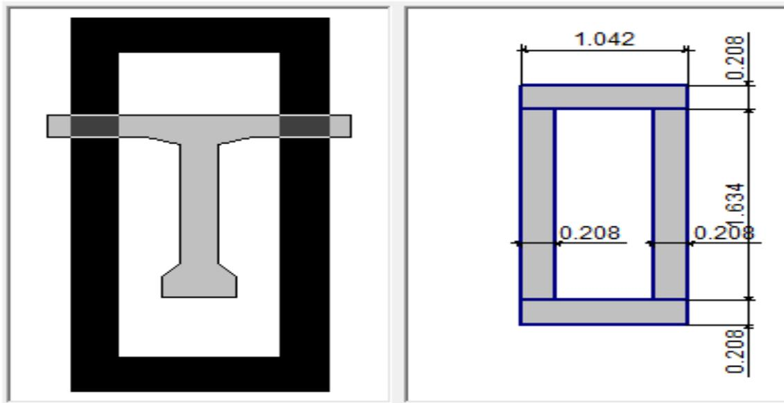
Figure 5.6: Equivalent hollow section
