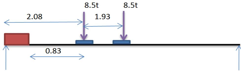
Figure 4.8: Transverse placement of 17t(B) Axles
