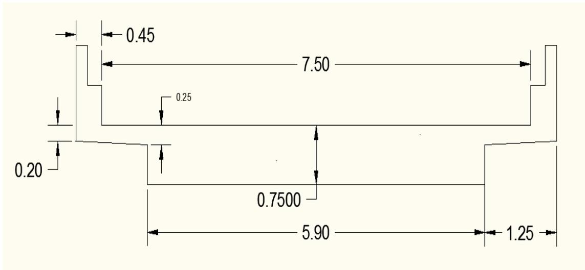
Figure 4.2: Cross section of solid deck slab
