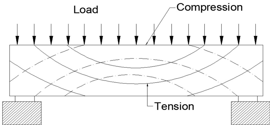
Figure 3.3: Principle stresses in a beam
