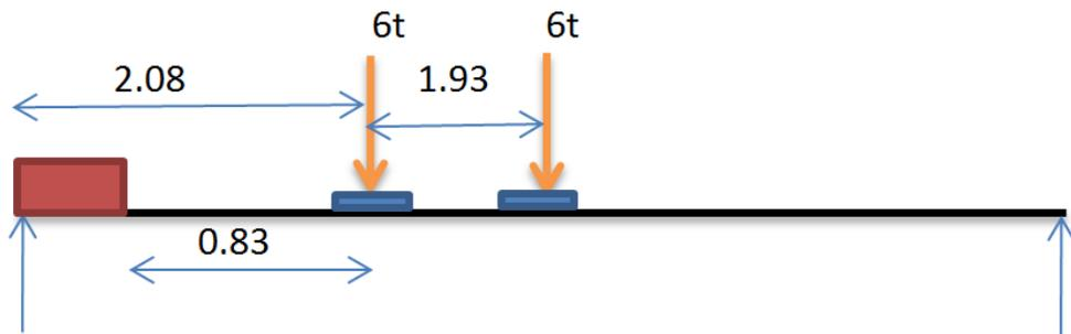
Figure 4.6: Transverse placement of 12t(R) Axles
