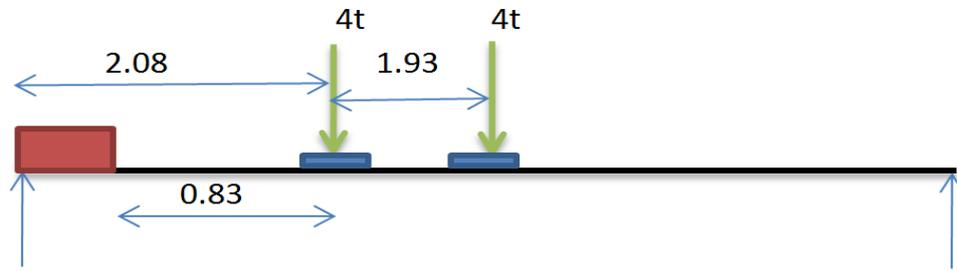
Figure 4.11: Transverse placement of 8t(D) Axles
