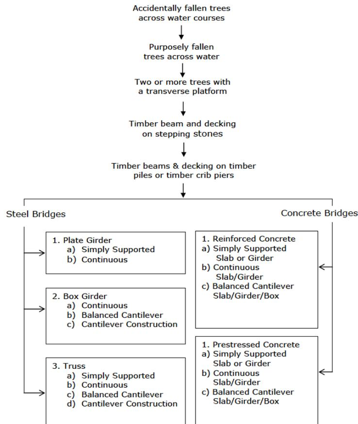
Figure 1.1: Development of various bridges from ancient times to the modern age
