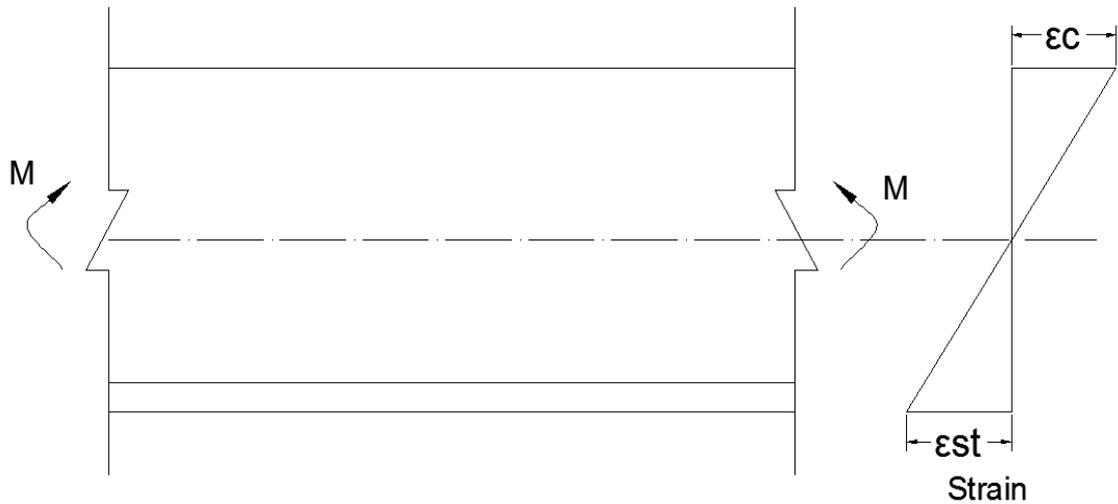
Figure 3.6: Bending of a length of beam
