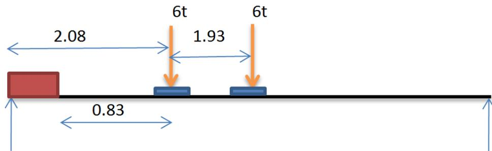
Figure 4.10: Transverse placement of 12t(C) Axles
