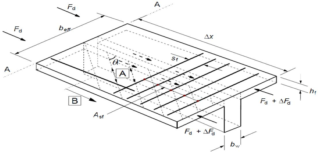
Figure 3.5: Shear between flange and web
