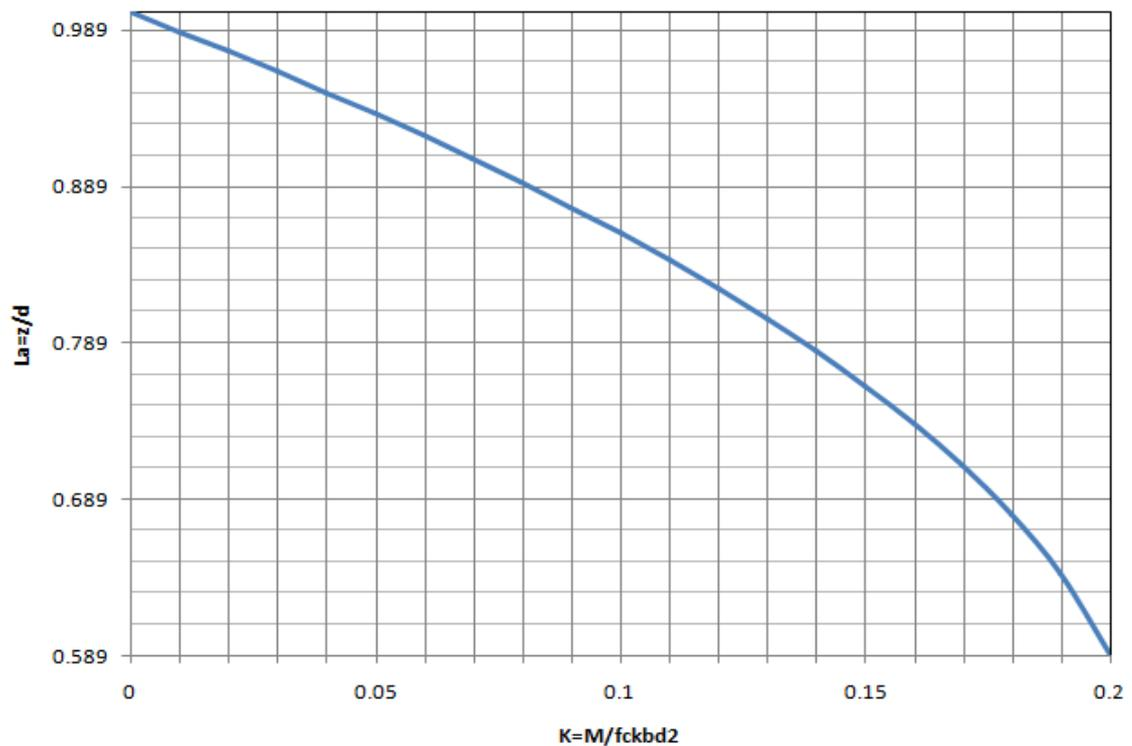
Figure 3.2: Lever-arm curve
