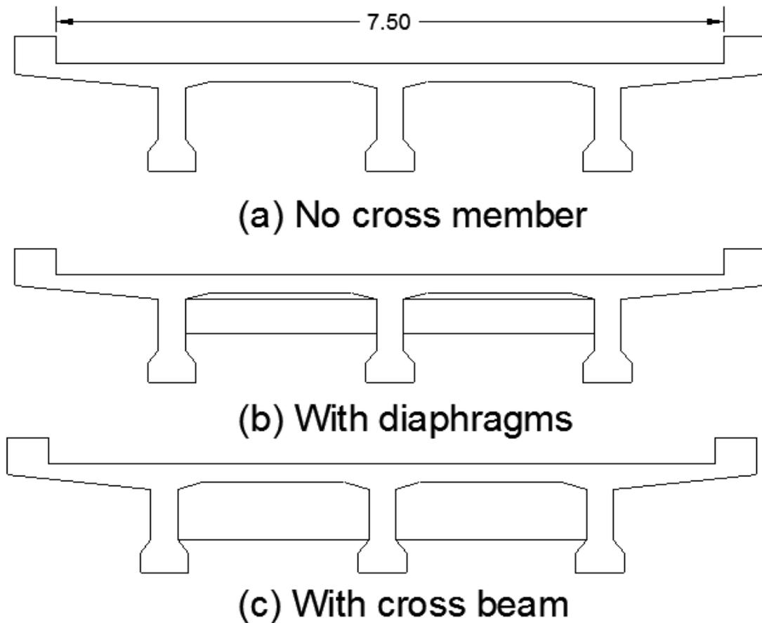
Figure 5.1: Typical cross section of T-beam bridges
