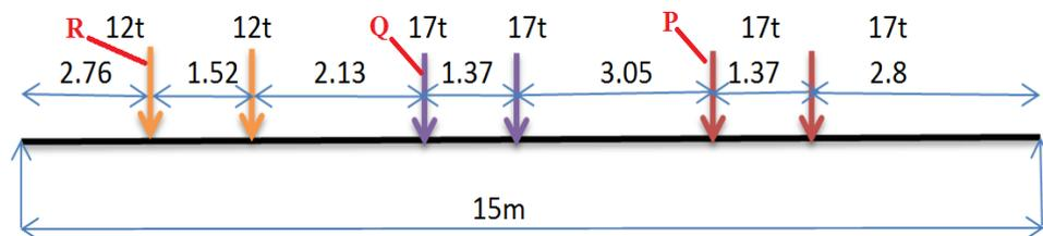
Figure 4.3: Loading for max. bending moment
