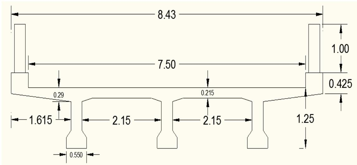
Figure 6.1: Cross section for different span
