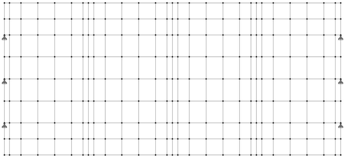
Figure 5.4: Grillage Model for 20m Span in Staad-Pro
