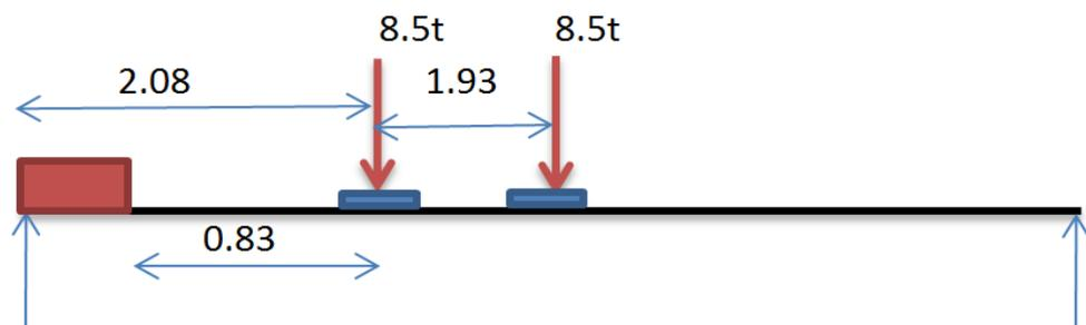
Figure 4.5: Transverse placement of 17t(P) Axles
