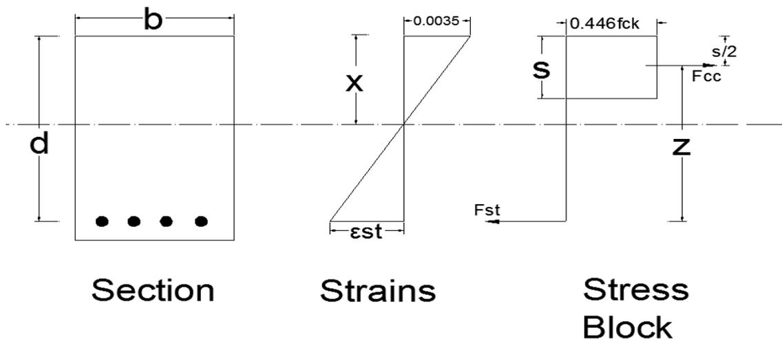
Figure 3.1: Rectangular Stress Block Diagram
