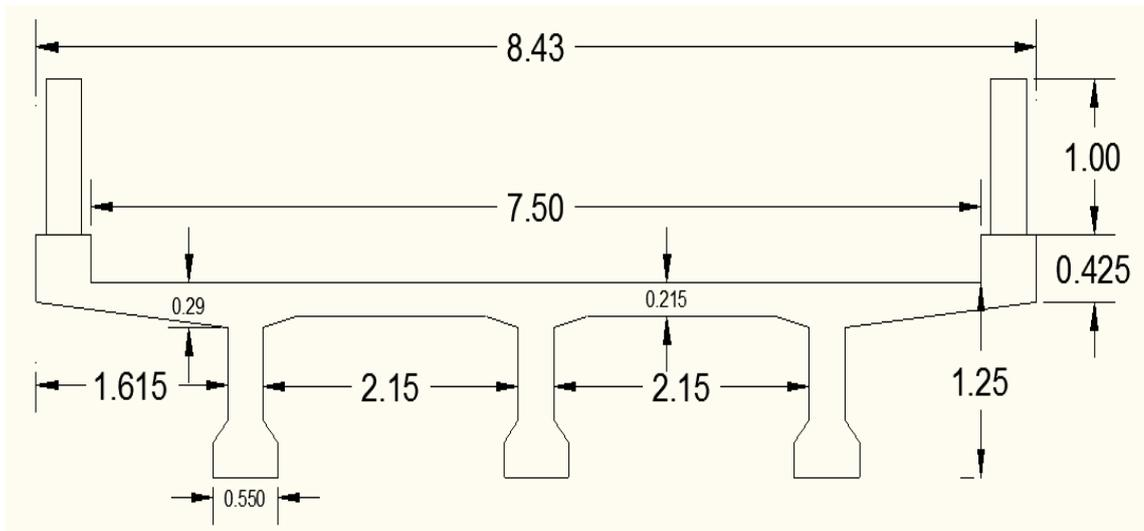
Figure 5.2: Cross section of T-beam bridge
