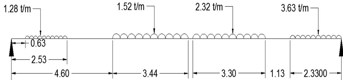
Figure 4.13: Loading for Maximum live shear force
