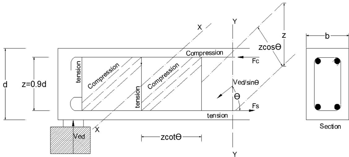
Figure 3.4: Assumed truss model for the variable strut inclined method
