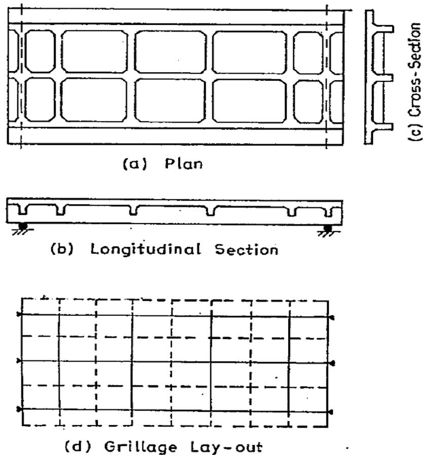
Figure 5.3: T-beam bridge and grillage lay-out
