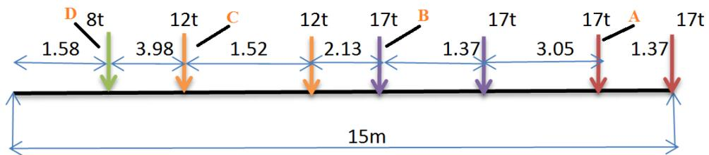
Figure 4.7: Loading for max. shear force
