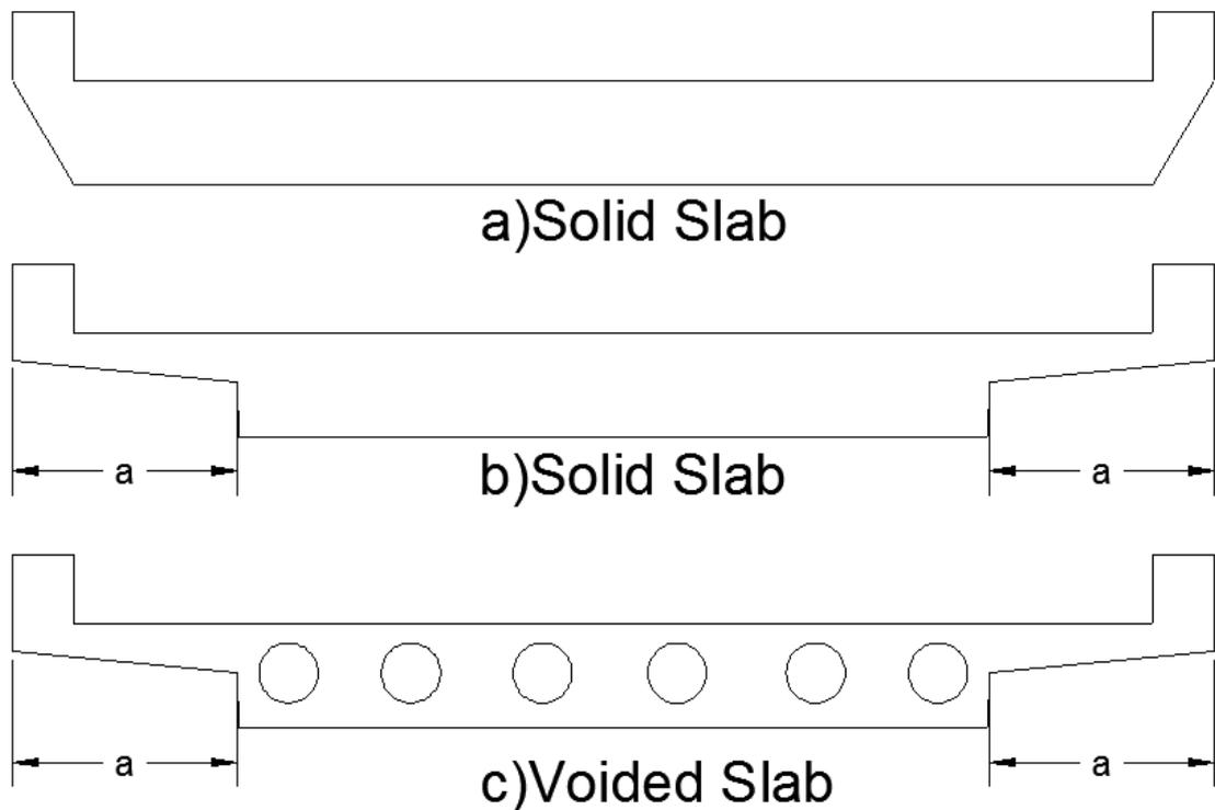
Figure 4.1: Slab Bridges
