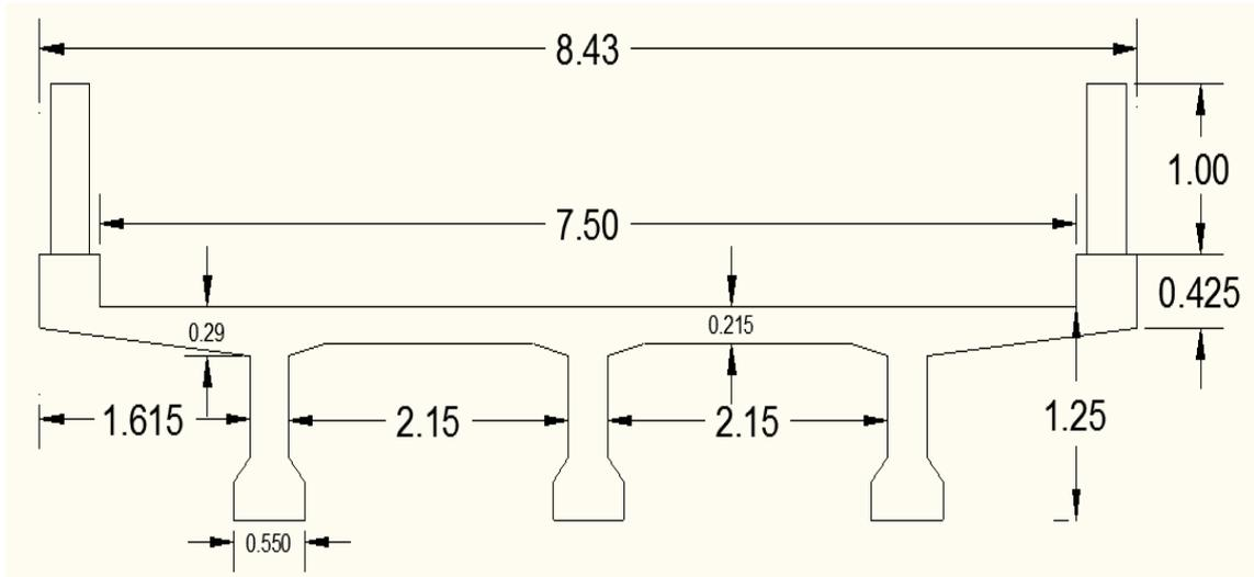
Figure 5.5: Cross Section for 20m Span
