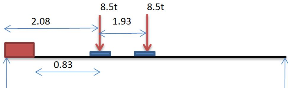
Figure 4.9: Transverse placement of 17t(A) Axles
