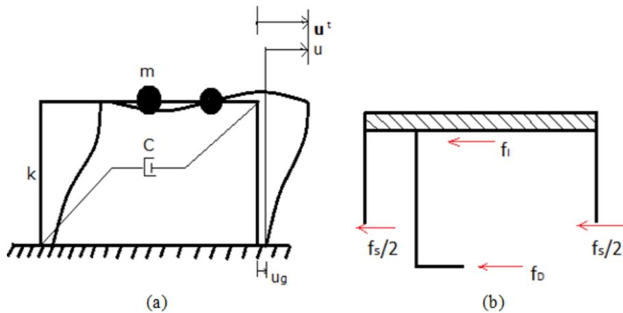
Figure 3.4: (a) SDOF system subjected to ground motion (b) Free Body Diagram
