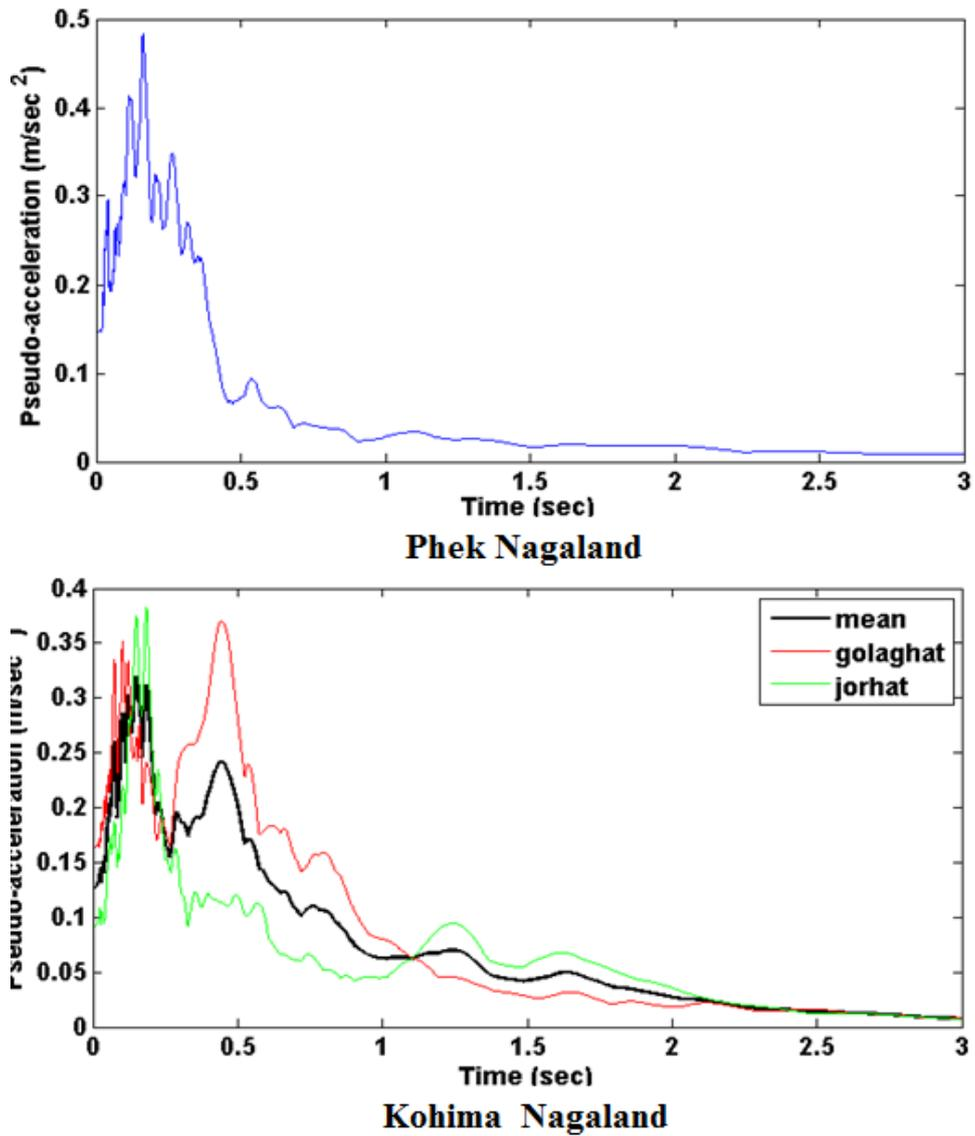
Figure 5.2: Mean response spectrum for 5% damping of horizontal ground motions
