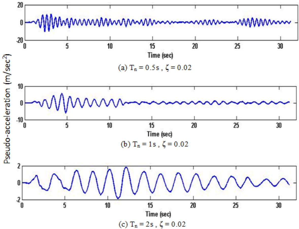
Figure 3.9: Pseudo-acceleration response of three SDOF systems with  $\zeta = 2\%$  and  $T_n = 0.5, 1$  and  $2$ sec. of El Centro ground motion
