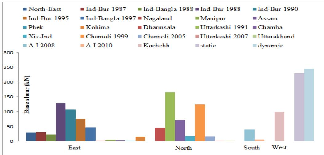
Figure 6.3: Base shear comparison for mean response spectrum (Dynamic analysis)
