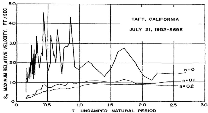
Figure 2.2: Typical earthquake response spectrum
