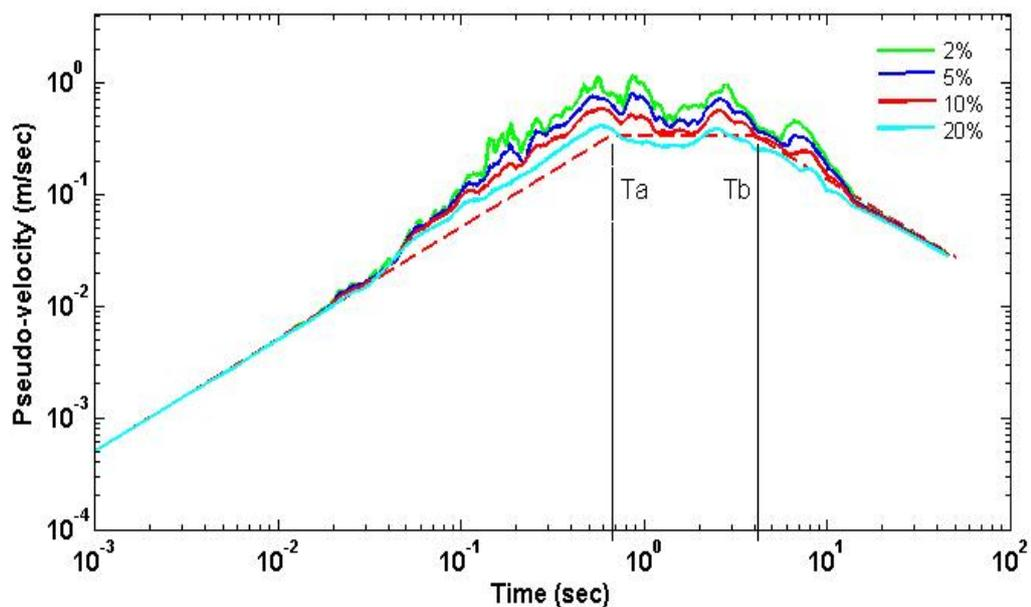
Figure 3.14: Combined D-V-A response spectrum for El Centro ground motion;  $\zeta = 2\%$ ,  $5\%$ ,  $10\%$  and  $20\%$
