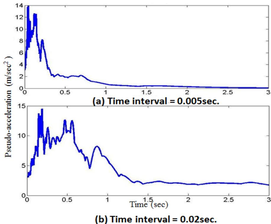
Figure 2.8: Response spectra with different interval in frequency range
