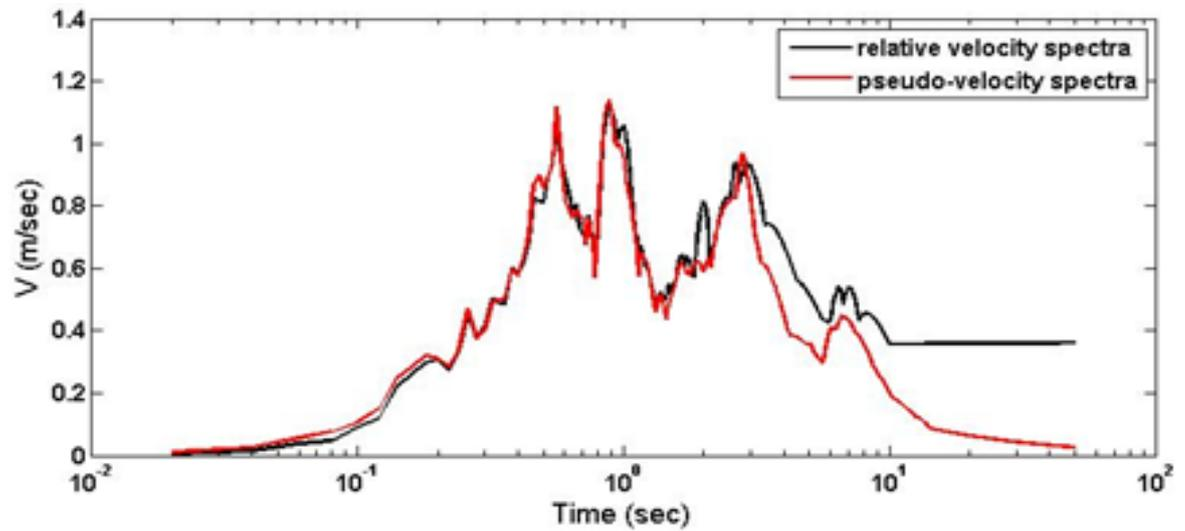
Figure 3.12: Comparison of pseudo-velocity and relative-velocity response spectra
