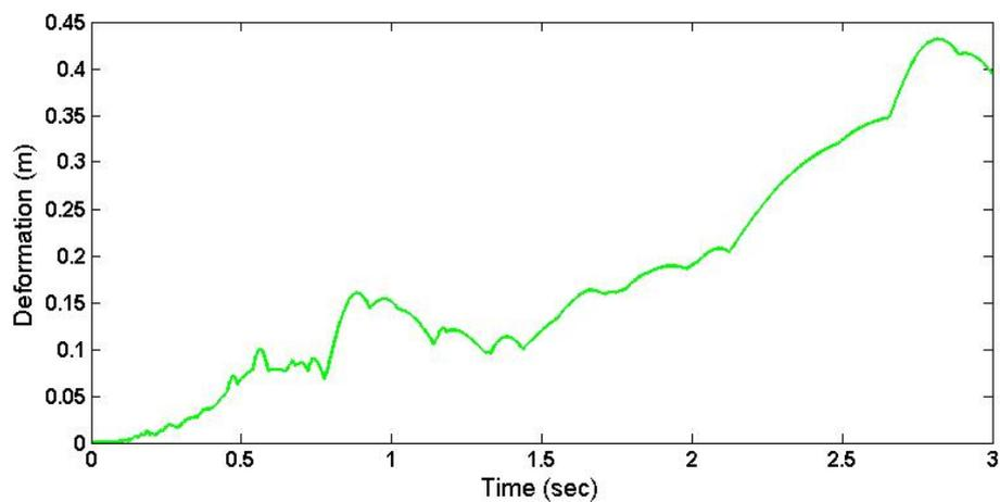
Figure 3.1: Deformation Response Spectrum for El Centro Ground Motion ( $\zeta = 0.02$ )
