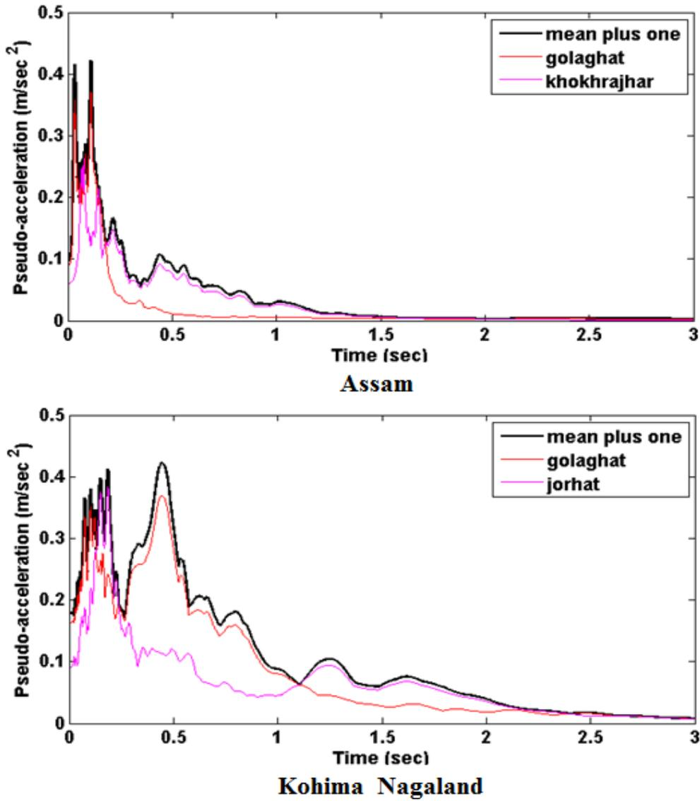
Figure 5.3: Mean +1  $\sigma$  response spectrum for 5% damping of horizontal ground motions
