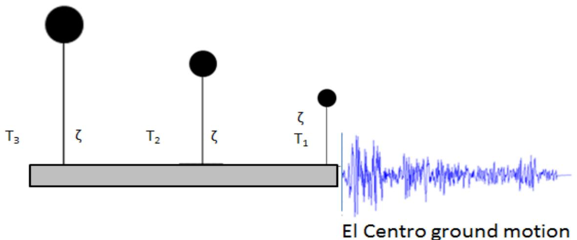
Figure 3.6: Different SDOF systems under earthquake ground excitation
