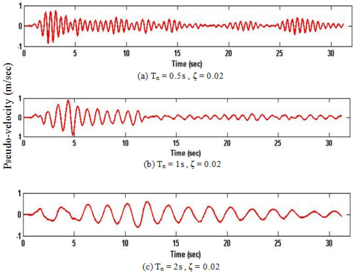
Figure 3.8: Pseudo-velocity response of three SDOF systems with  $\zeta = 2\%$  and  $T_n = 0.5, 1$  and  $2$  sec. of El Centro ground motion
