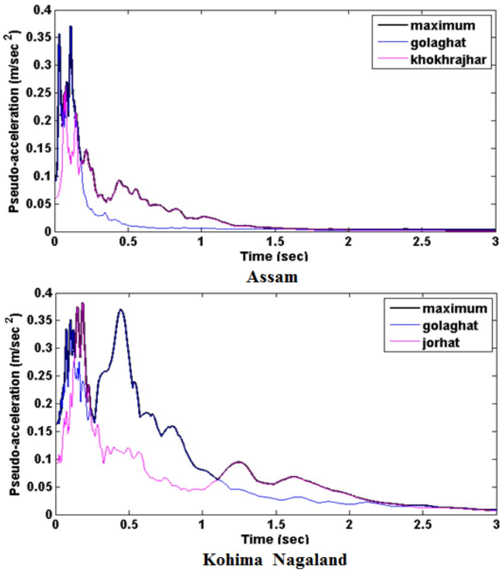
Figure 5.4: Maximum response spectrum for 5% damping of horizontal ground motions
