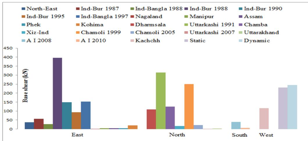
Figure 6.8: Base shear comparison for maximum response spectrum (Static analysis)
