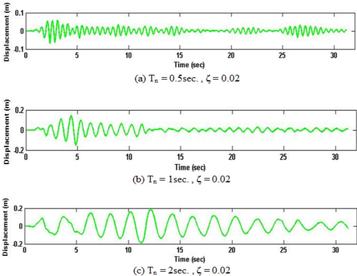
Figure 3.7: Deformation response of three SDOF systems with  $\zeta = 2\%$  and  $T_n = 0.5, 1$  and  $2 \text{ sec.}$  of El Centro ground motion
