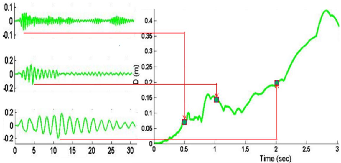
Figure 3.10: Deformation response spectrum of El Centro ground motion
