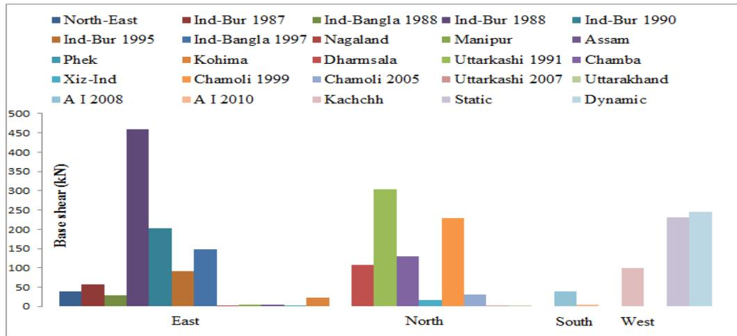
Figure 6.7: Base shear comparison for maximum response spectrum (Dynamic analysis)
