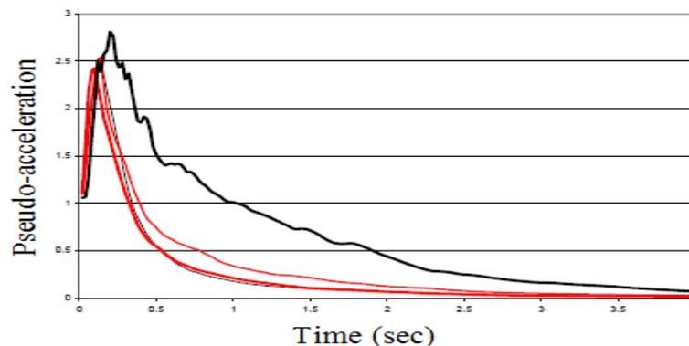
Figure 2.6: Average Pseudo-Acceleration Response Spectrum (Damping 5%)
