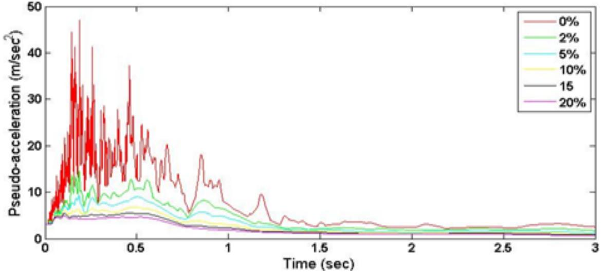
Figure 3.11: Normalized pseudo-acceleration response spectrum for El Centro ground motion for different damping ( $\zeta = 0\%$ ,  $2\%$ ,  $5\%$ ,  $10\%$ ,  $15\%$ ,  $20\%$ )
