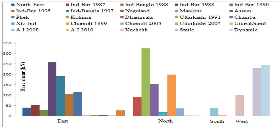
Figure 6.5: Base shear comparison for mean  $+1 \sigma$  response spectrum (Dynamic analysis)
