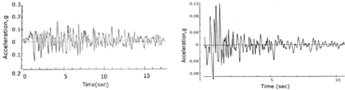
Figure 2.4: Accelerogram for Taft and Vernon, California, earthquake
