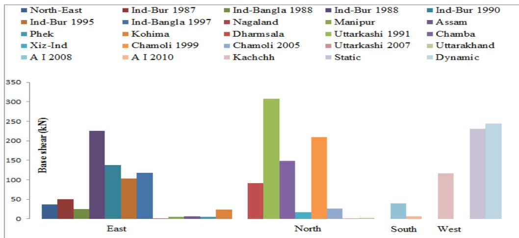
Figure 6.6: Base shear comparison for mean  $+1 \sigma$  response spectrum (Static analysis)
