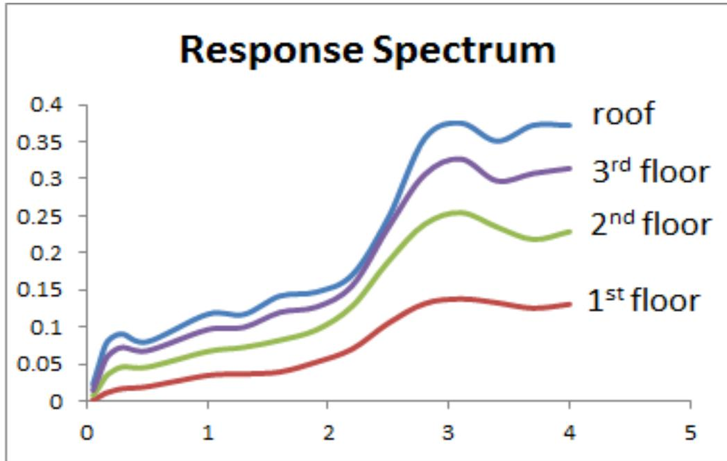
Figure 7.1: Response spectrum subjected to El Centro ground motion for all storey
