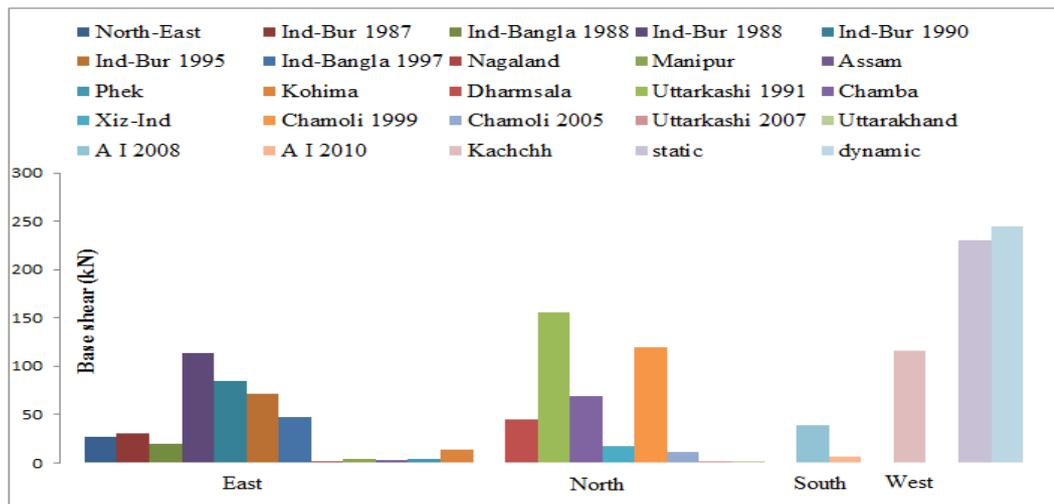
Figure 6.4: Base shear comparison for mean response spectrum (Static analysis)
