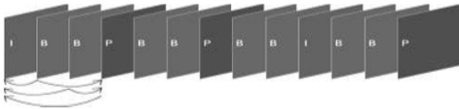
Figure 2.5: I, P and B frames [1]
