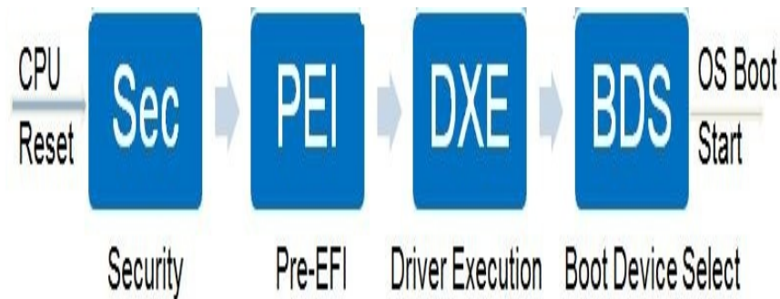
Figure 2.2: EFI BIOS boot phases
