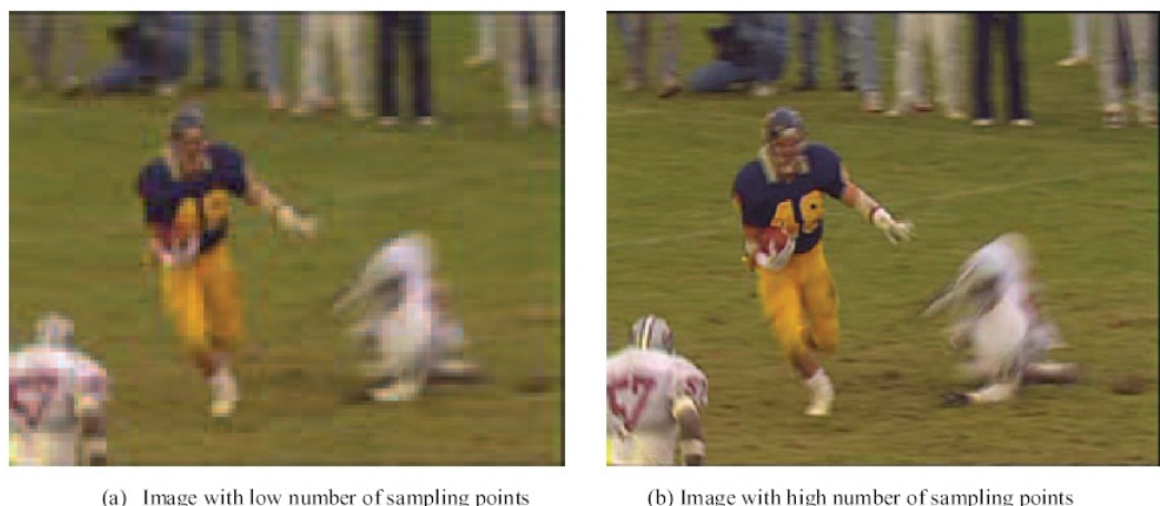
Figure 1.5: Image with different number of sampling points(a.176x144, b.352x288) [7]
