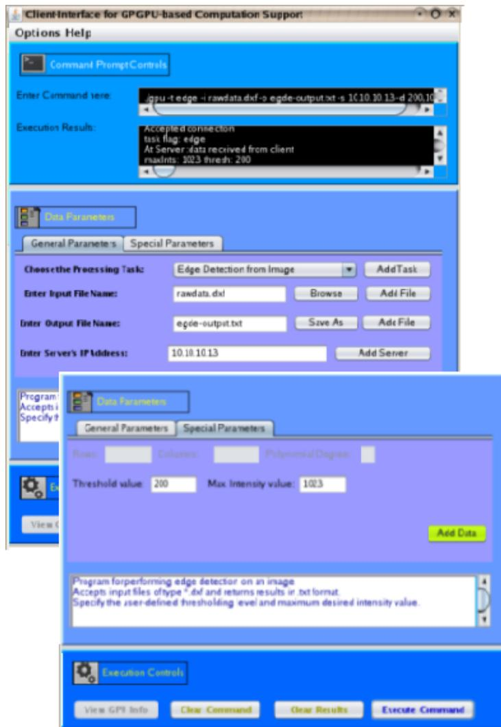
Figure 7.5: GUI configuration for Edge Detection and Ranking
