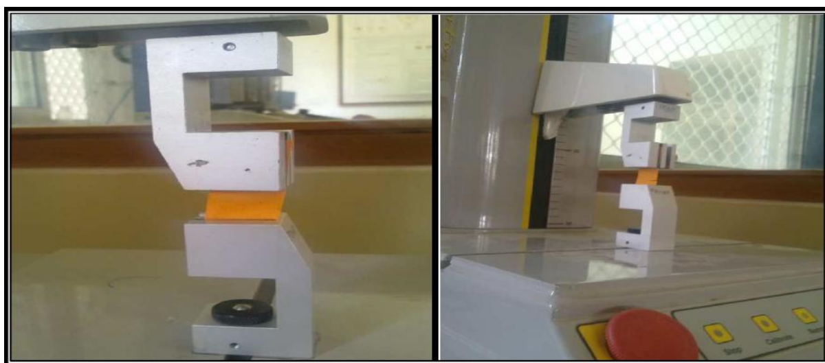
FIGURE 2.5 ASSEMBLY OF TEXTURE ANALYSER
