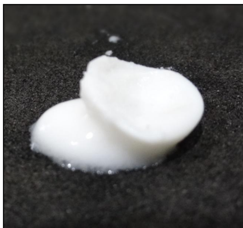
Figure 4.20: Collapsed tablet after dissolution
