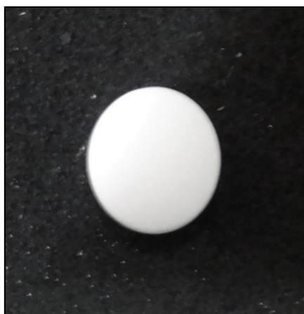
Figure 4.18: Tablet before dissolution (Intact tablet)
