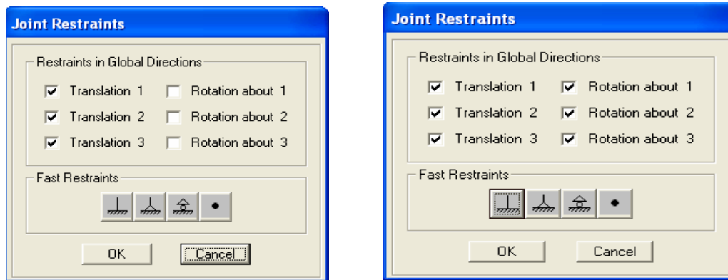
Fig. 4.14: Joint Restraints Dialogue Box
