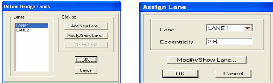
Fig. 4.20: Define and Assign Bridge Lanes
