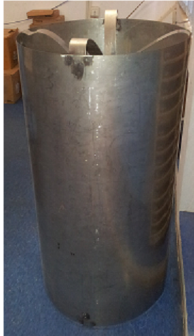
Figure 5.3: Cylinder representing inner current carrying conduit [Courtesy: Ongoing experimental work at ITER India]
