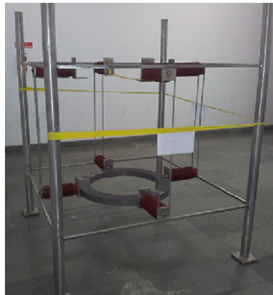
Figure 5.7: Prototype transmission model with two snubber core [Courtesy: Ongoing experimental work at ITER India]
