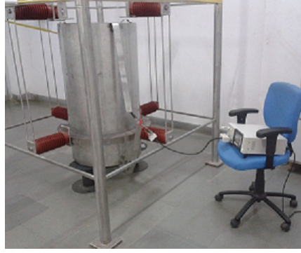
Figure 5.8: Inductance measurement of the Snubber [Courtesy: Ongoing experimental work at ITER India]
