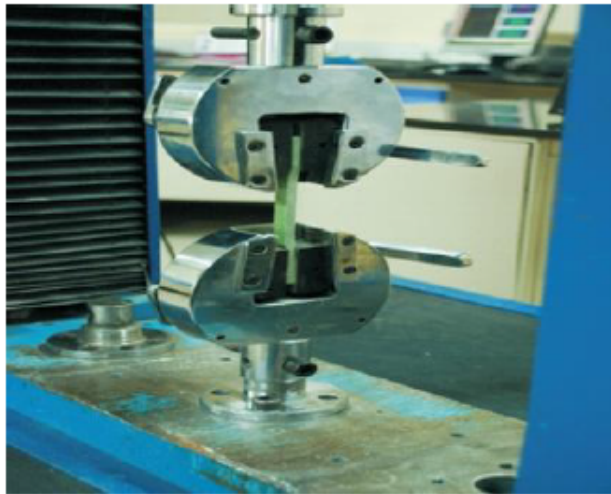
Figure 5.2: Axial Tensile Test set up
