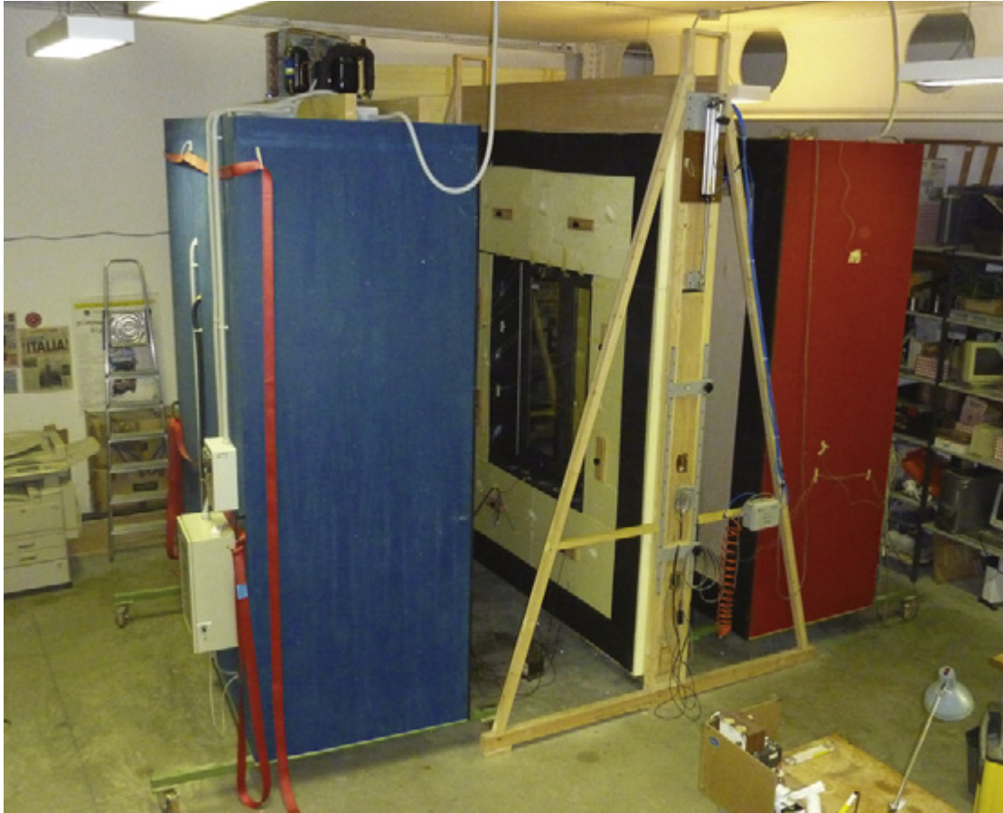
Figure 1.2: Photograph of guarded hot box apparatus[1]
