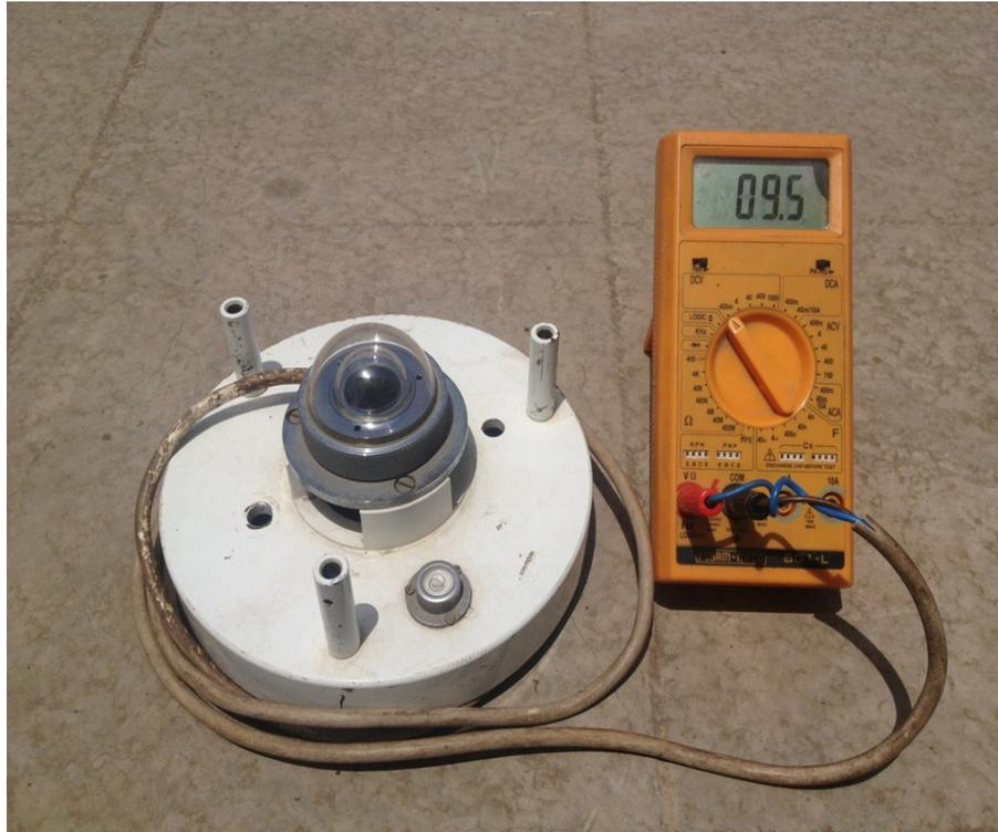
Figure 4.10: Solar pyranometer
