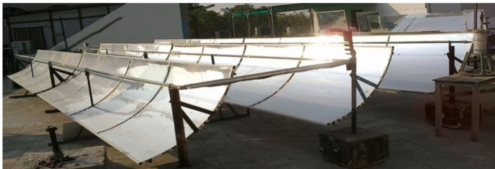
Figure 4.1: parabolic trough collector
