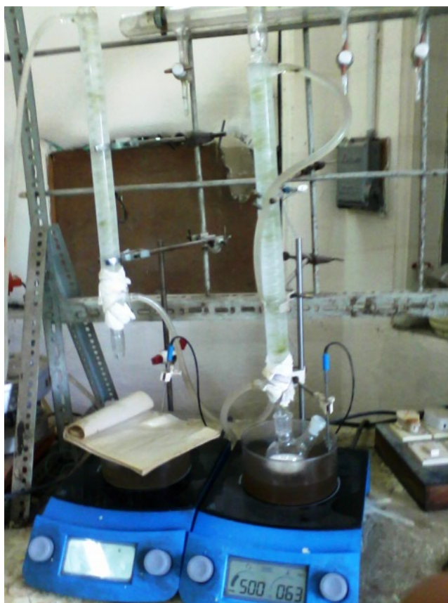
Figure 3.2: Batch Reactor (RBF) Reaction Arrangement
