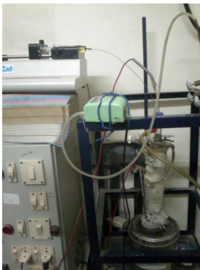
Figure 3.3: Fixed Bed Reactor Arrangement
