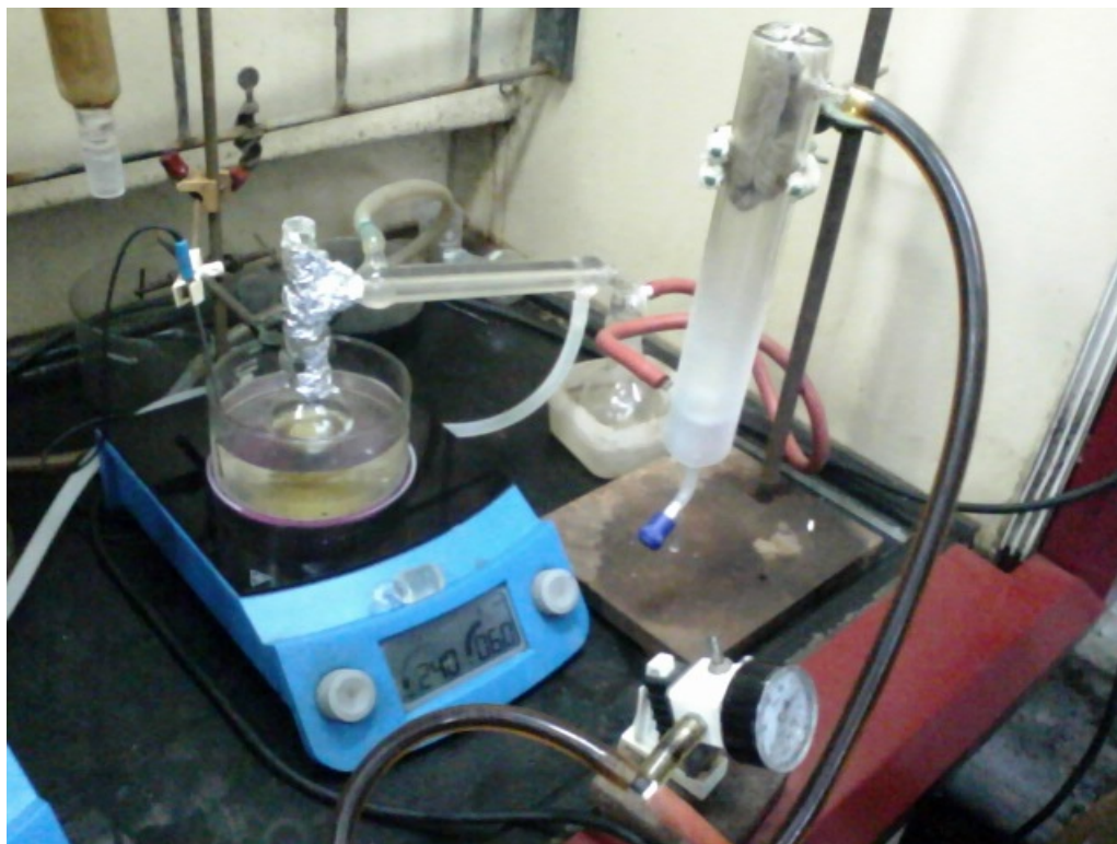
Figure 3.1: Distillation Arrangement Of Longifolene
