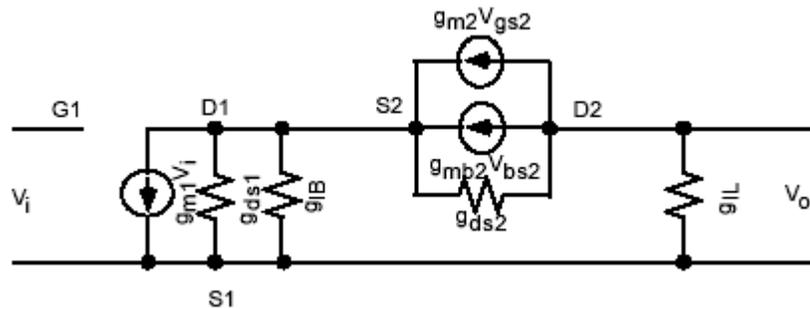
Fig: 4.4 Equivalent circuit of Folded Cascode
