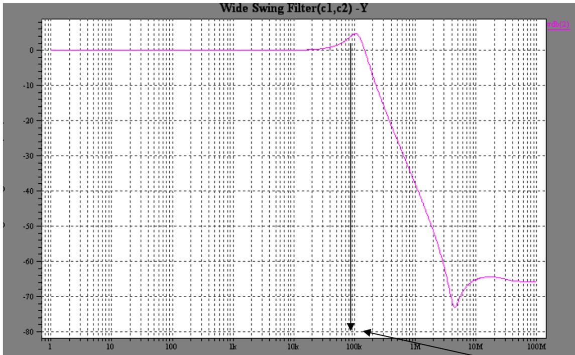
Fig:6.15 Low Pass Filter ( $V_{in} = V_1$ , with  $V_2$  and  $V_3$  grounded)
