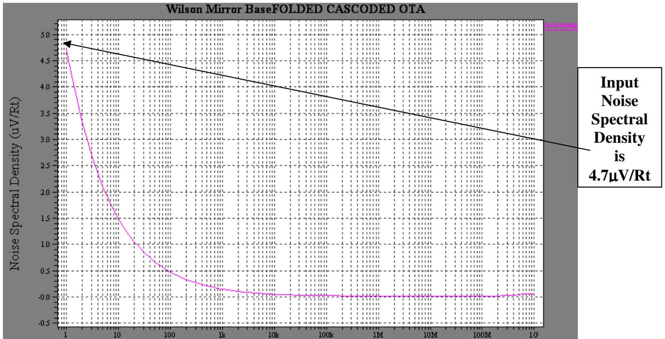
Fig: 4.17 Input Noise Spectral Density for Folded Cascode OTA
