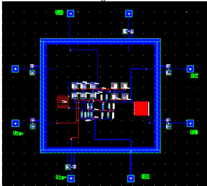
Fig:4.25 Physical Design of Biassing Circuit and Wide Swing OTA(-CMR)
