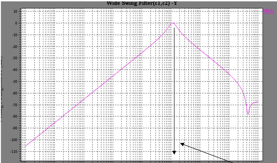
**Fig: 6.17 Band Pass Filter ( $V_{in} = V_2$ , with  $V_3$  and  $V_1$  grounded)**
