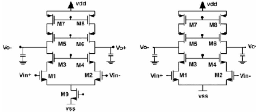
**Fig 2.3 (a) Telescopic amplifier      Fig 2.3 (b) No-tail telescopic amplifier**
