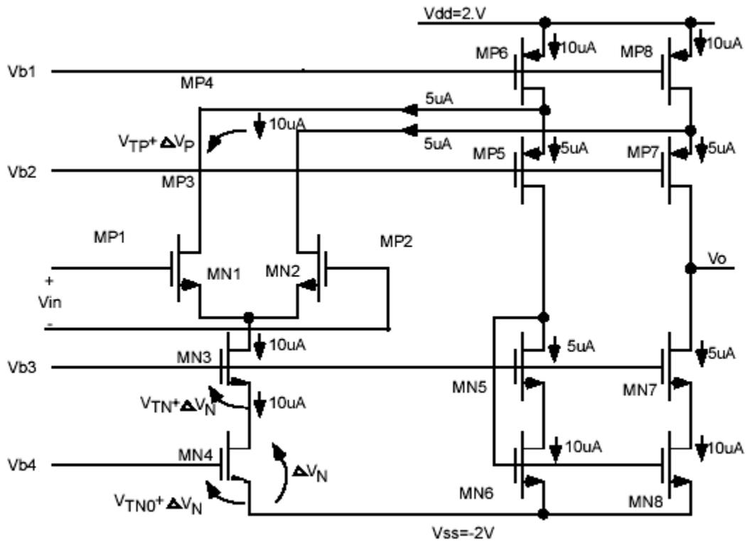
Fig: 4.23 Wide Swing OTA (NMOS Differential Pair-Poor Negative CMR) Circuit
