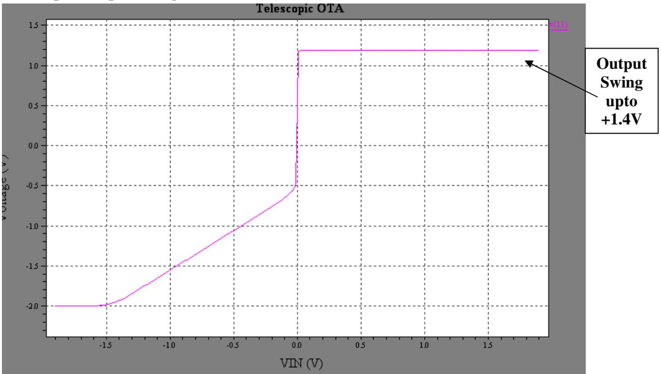
**Fig: 3.6 Input/Output Swing and Offset Measurement of Telescopic OTA**
