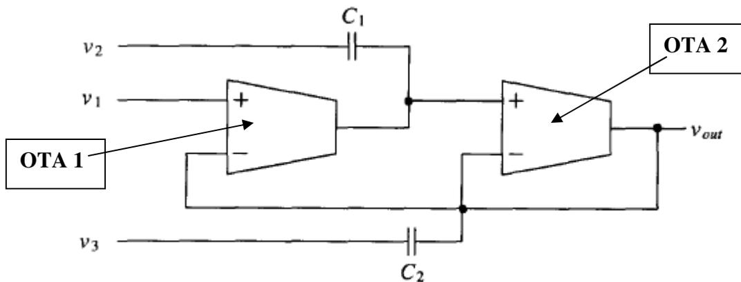
**Fig: 6.14 Biquad Filter (2<sup>nd</sup> Order) Implementation using OTAs Schematic**
