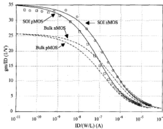
Fig. 4.9.  $g_m / I_D$  versus  $I_D / (W / L)$  curve
