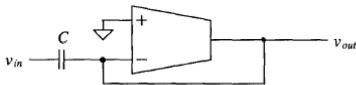
**Fig: 6.11 High Pass Filter using OTA**
