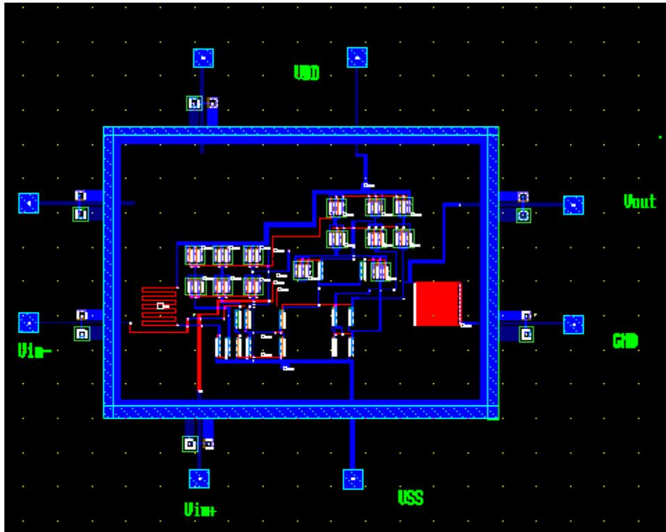
Fig:4.33 Physical Design of Wide Swing Folded Cascode OTA
