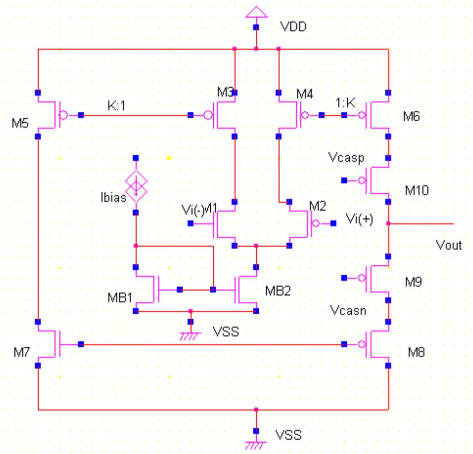
Fig: 1.2 CONVENTIONAL ONE-STAGE TRANSCONDUCTANCE AMPLIFIER
