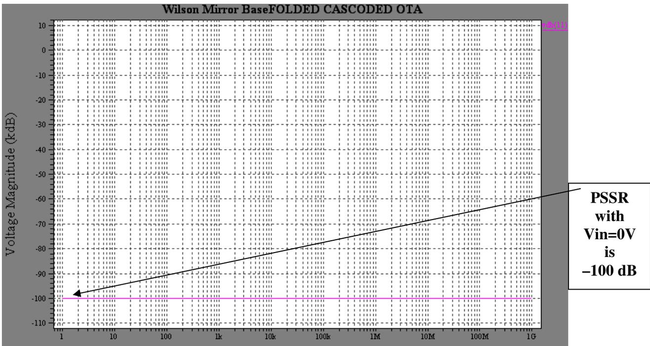
**Fig: 4.16 PSSR Measurement with  $V_{in}=0V$  for folded Cascode OTA**
