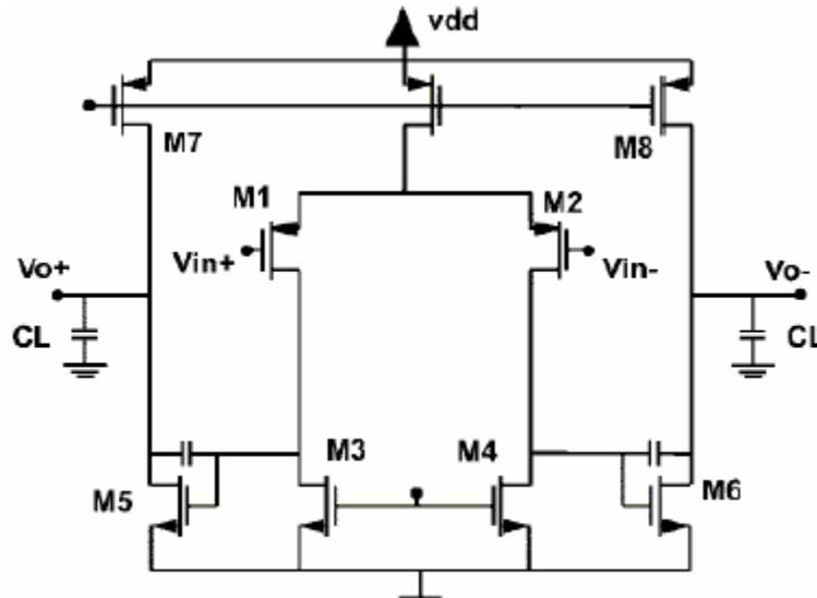
**Fig 2.1 Two – Stage amplifier**
