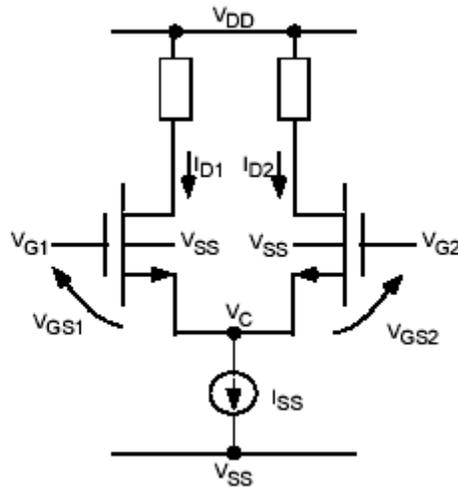
**Fig: 3.2 Differential Input pair**
