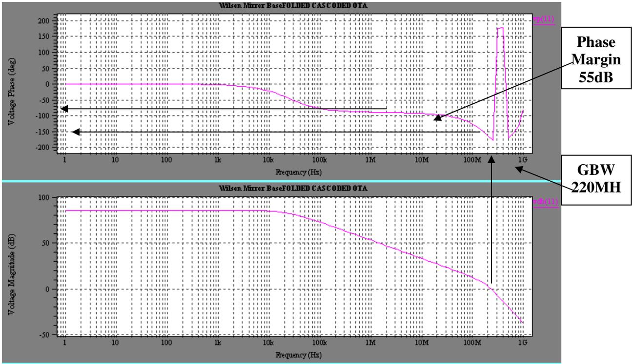
**Fig: 4.11 Gain Bandwidth and Phase Margin of Folded Cascode OTA**
