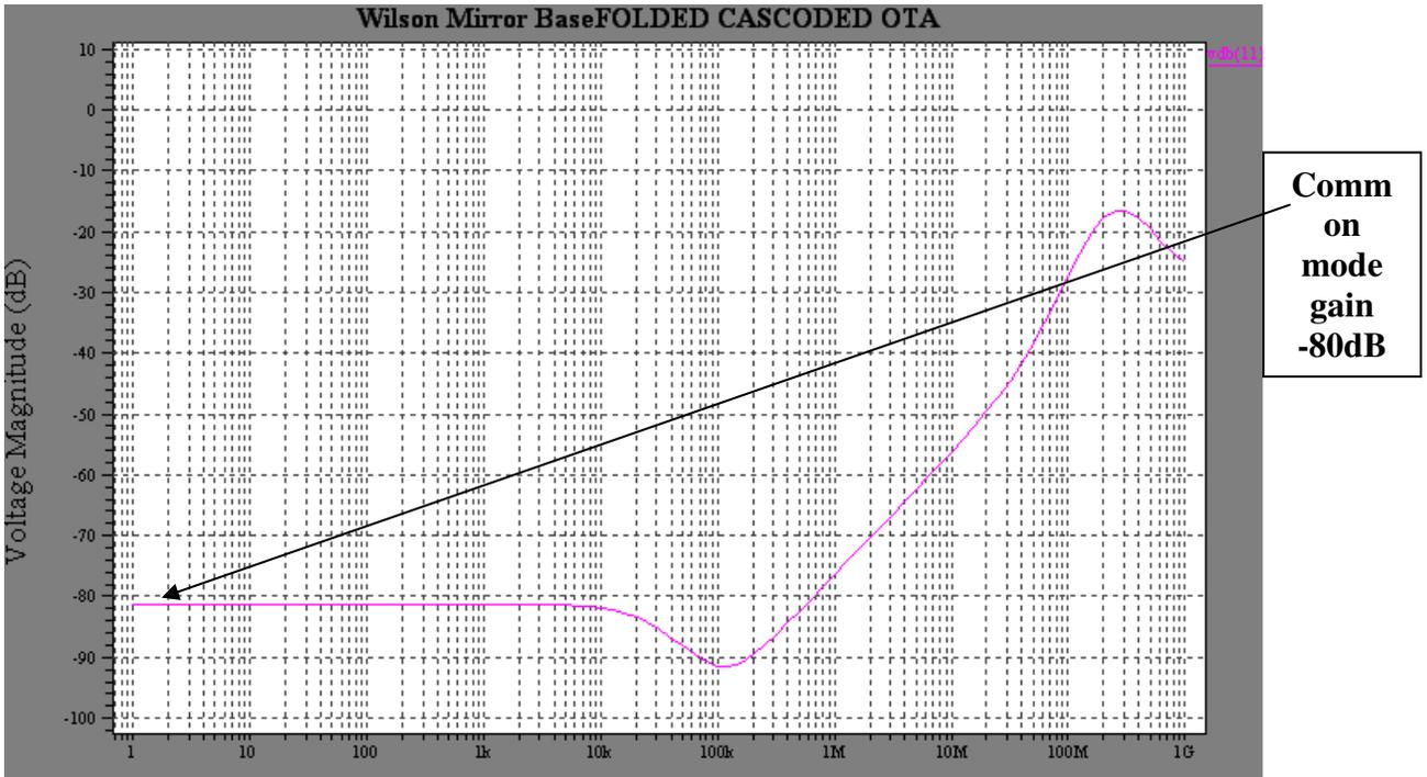
**Fig: 4.14 Common Mode Gain of Folded Cascode OTA**
