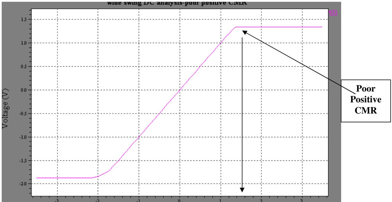
Fig: 4.27 Wide Swing OTA (PMOS Differential Pair-Poor Positive CMR) Result
