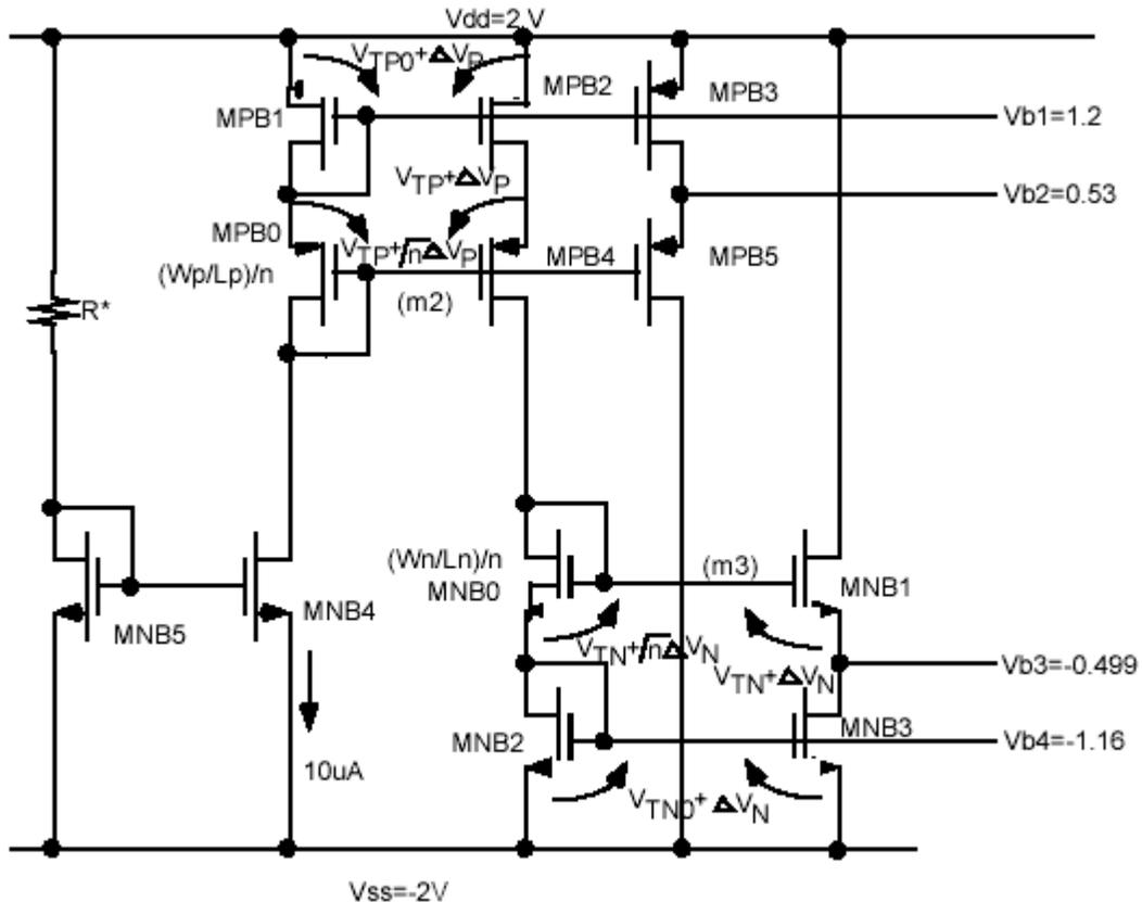
Fig: 4.22 Modified Bias Circuit
