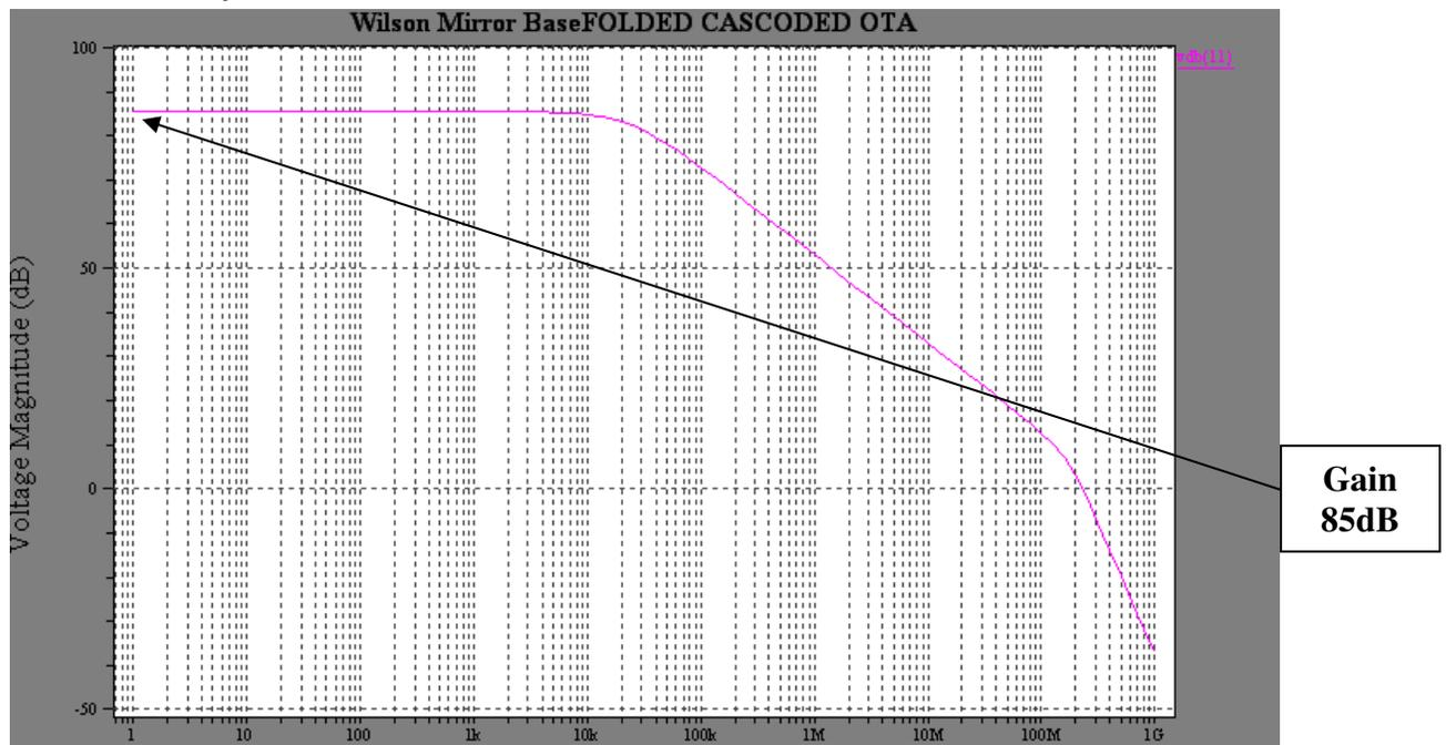
Fig: 4.10 AC Analysis of Folded Cascode OTA
