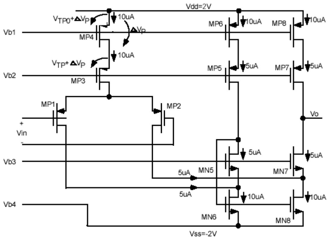
**Fig: 4.26 Biasing and Wide Swing OTA (PMOS Differential Pair-Poor Positive CMR) Circuit**
