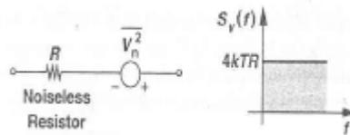
**Fig:5.2 Thermal noise of a resistor**
