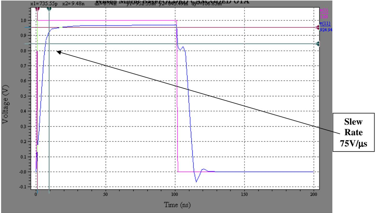
**Fig: 4. 13 Slew Rate of Folded Cascode OTA**
