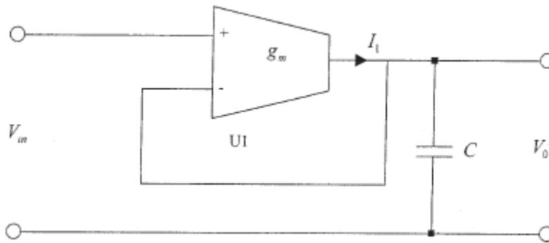
**Fig: 6.9 first order Low Pass Filter (Active Filter)**
