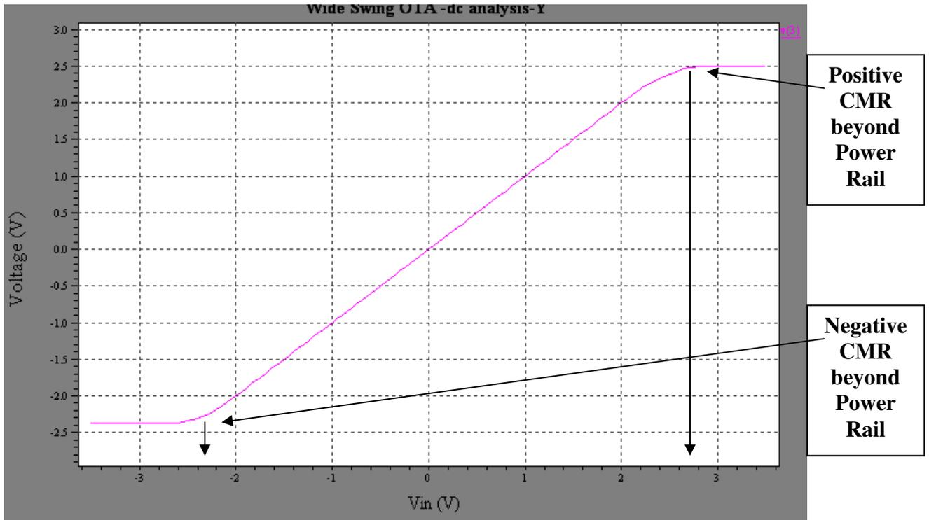
**Fig: 4.32 DC Analysis for Wide Swing Folded Cascode OTA**
