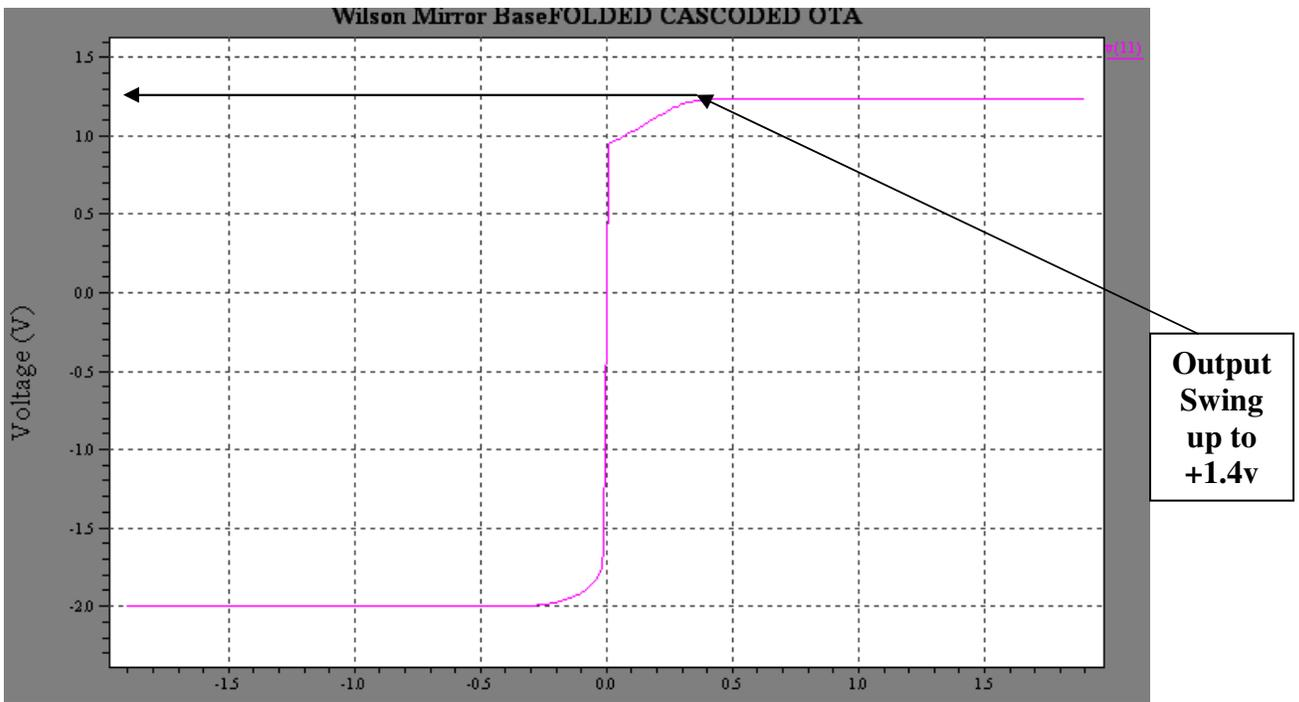
**Fig: 4.12 Input-Output Swing of Folded Cascode OTA**
