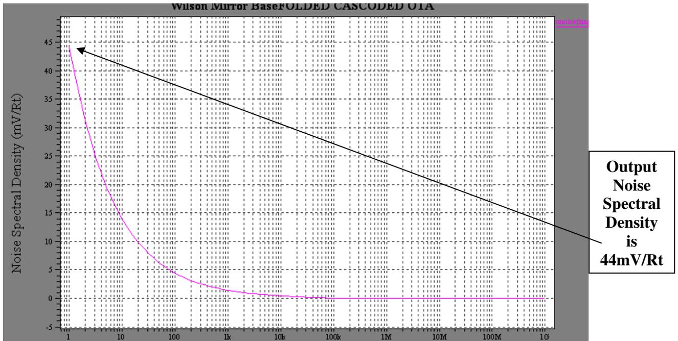
**Fig: 4.18 Output Noise Spectral Density for Folded Cascode OTA**
