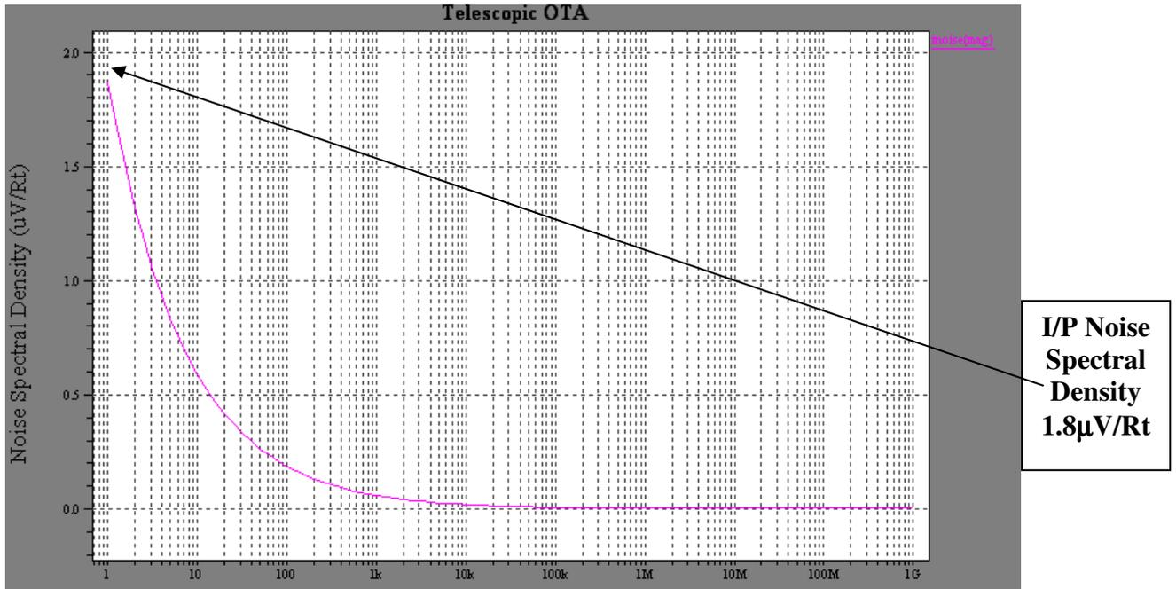
Fig: 3.9 Input Noise Spectral Density
