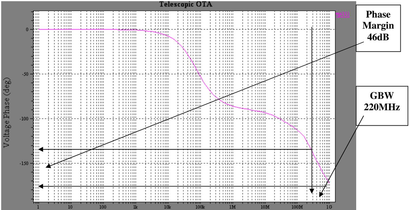
**FIG:3.5 PHASE MARGIN AND GAIN BANDWIDTH PRODUCT**
