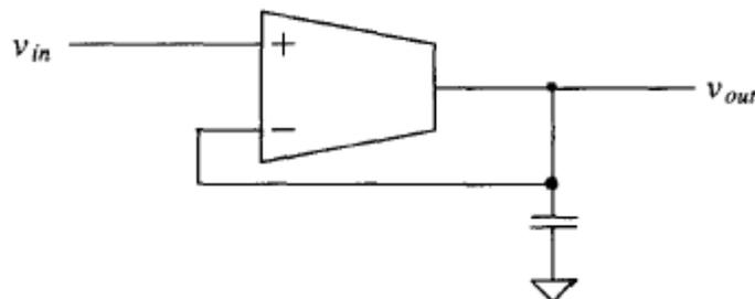
**Fig: 6.10 Low Pass Filter using OTA**
