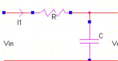
**Fig: 6.8 First Order Low Pass Filter (Passive Filter)**
