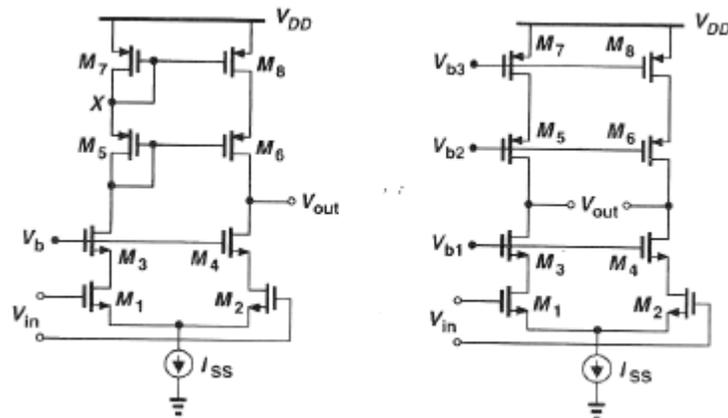
Fig:4.5 Single Ended and Double Ended Telescopic OTA
