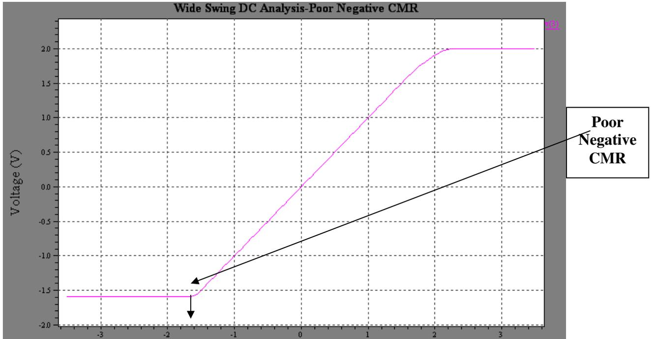
Fig: 4.24 Wide Swing OTA (NMOS Differential Pair-Poor Negative CMR) Result
