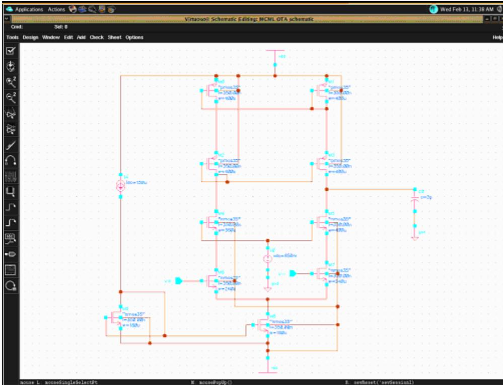
**Fig:3.11 Schematic of Telescopic OTA**
