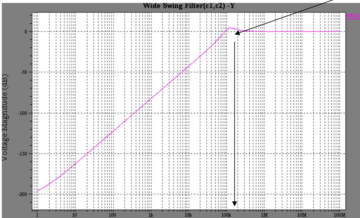
Fig: 6.16 High Pass Filter ( $V_{in} = V_3$ , with  $V_2$  and  $V_1$  grounded)
