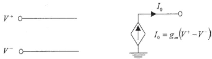
**Fig: 6.3 Small Signal Equivalent Circuit**
