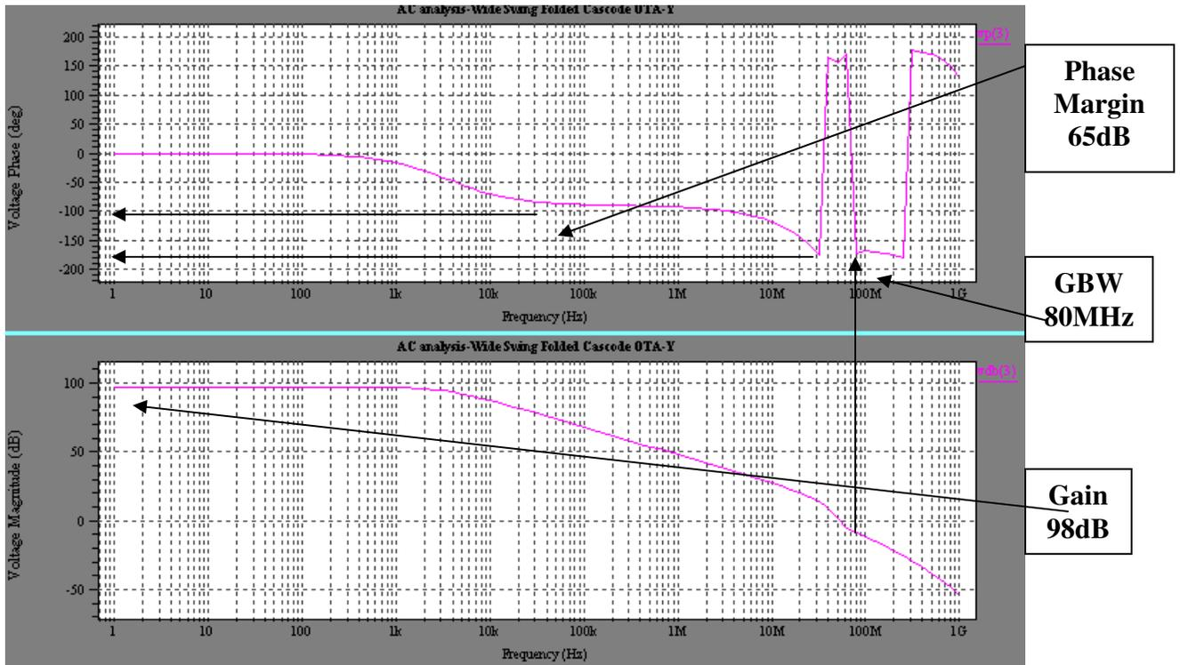
**Fig:4.31 Simulation Result for Wide Swing Folded Cascode OTA
