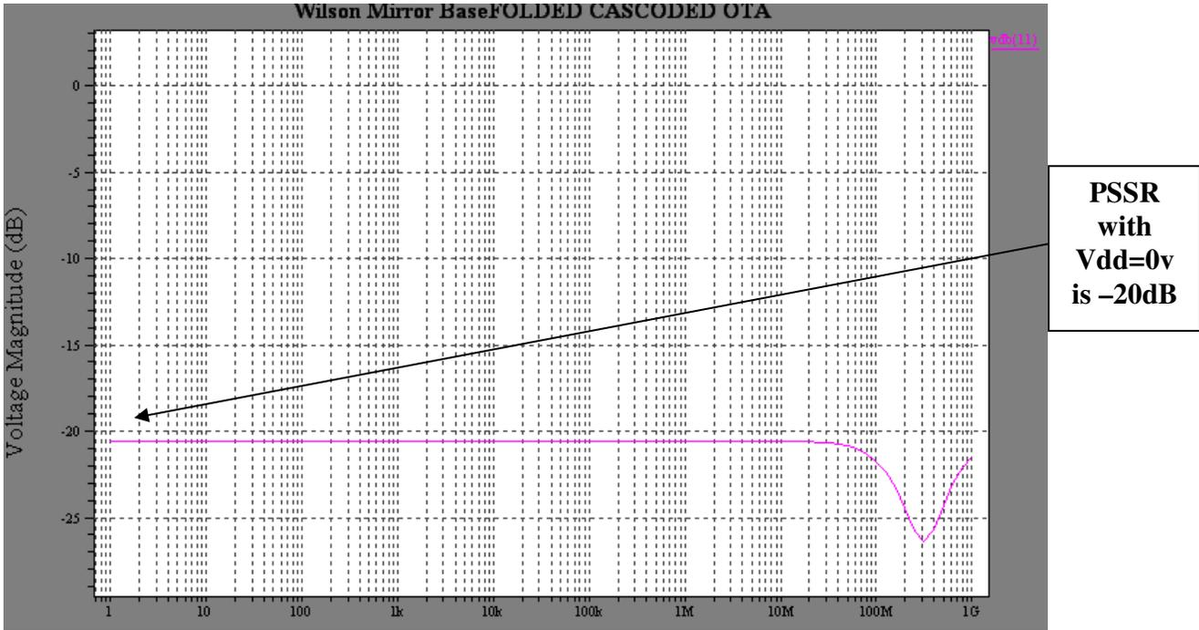
**Fig: 4.15 PSSR Measurement with  $V_{dd}=0V$  for Folded Cascode OTA**
