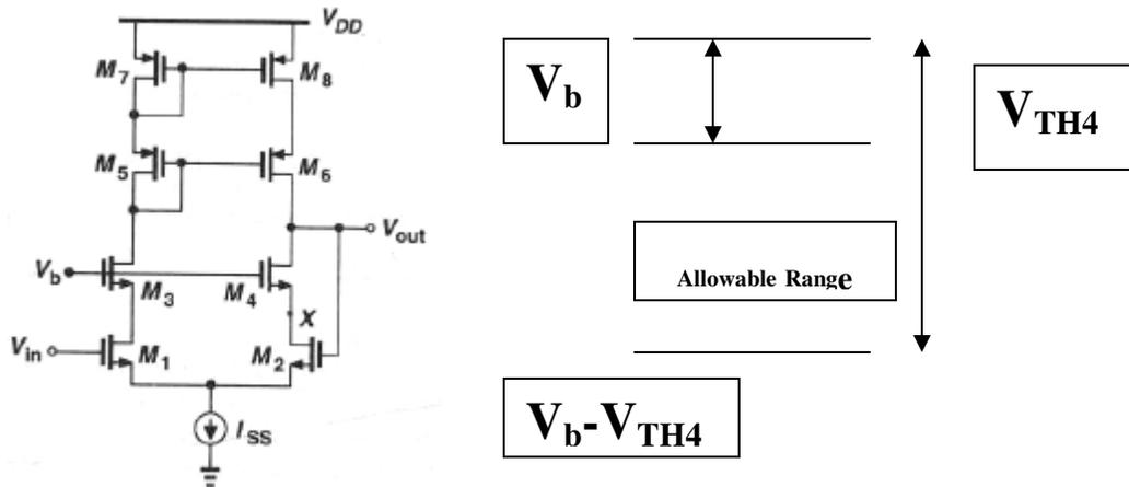
Fig: 4.6 Telescopic OTA with input and output shorted
