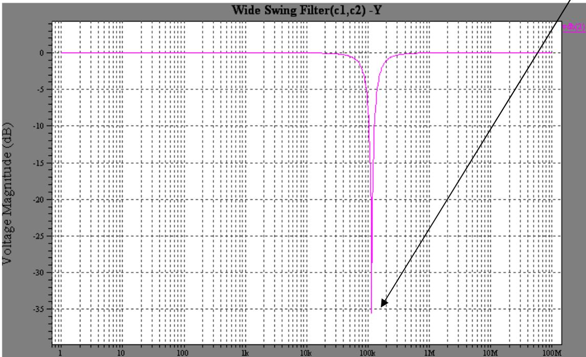
**Fig: 6.18 Band Pass Filter ( $V_{in} = V_3 = V_1$  with  $V_2$  grounded)**
