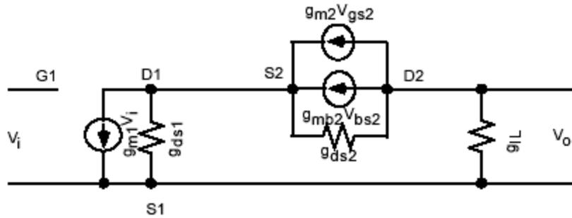
Fig: 4.3 Equivalent circuit of Telescopic Cascode
