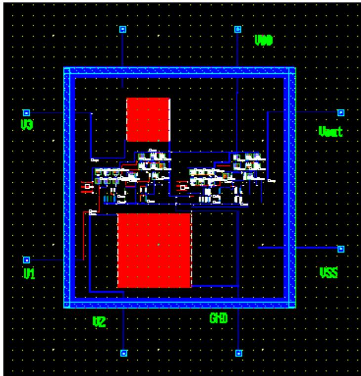
Fig:6.19 Physical Design of 2<sup>nd</sup> order Biquad Filter
