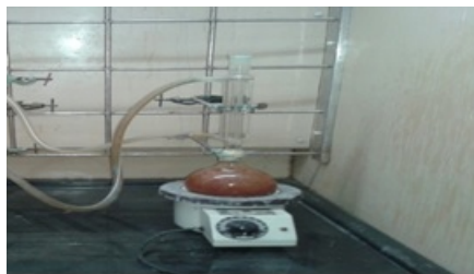
Figure 3.1: Synthesis experimental setup (Reflux method)
