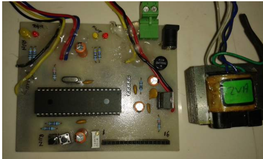
Figure 5.2: PIC micro controller board circuit
