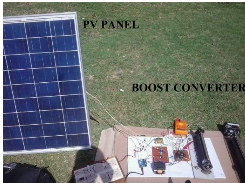
Figure 9: Integration of PV panel with boost converter
