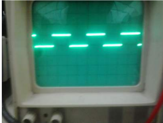
Figure 5.1: Input Pulse : X axis = 0.0005 sec/Div , Y axis = 5 V/Div
