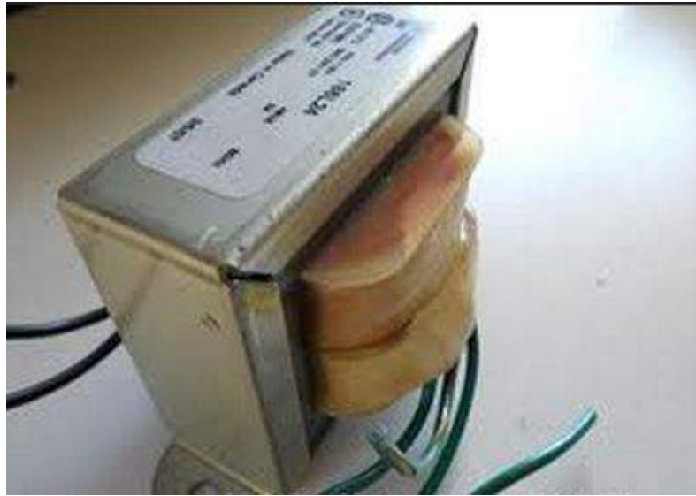
Figure 5.2: Transformer for Power Supply
