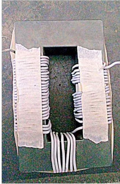
Figure 4.1: Designed Inductor 15mH
