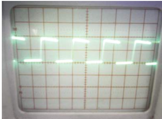
Figure 7.5: Output of inverter for upper two switches [Scale:X-axis:10 ms, Y-axis:5 V/div]
