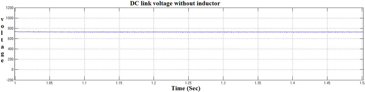
Figure 7.10: X-axis=Time(sec),Y-axis=Voltage,DC link voltage without inductor.
