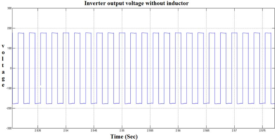
Figure 7.11: X-axis=Time(sec),Y-axis=Voltage,inverter output voltage without inductor.
