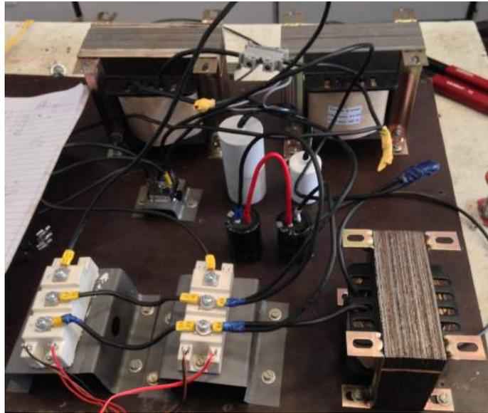
Figure 10.2: Sectional view of the Rectifier and LCL tank circuit.
