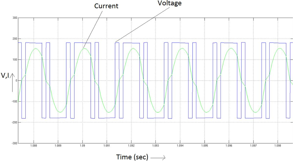
Figure 7.6: X-axis=Time(sec),Y-axis=Voltage and Current,Inverter output voltage and current at 70 percent load.
