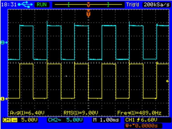
Figure 10.5: gate driver output for IGBT AH and BL
