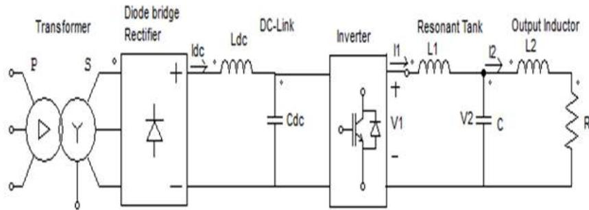
Figure 5.2: IGBT based LCL resonance inverter.
