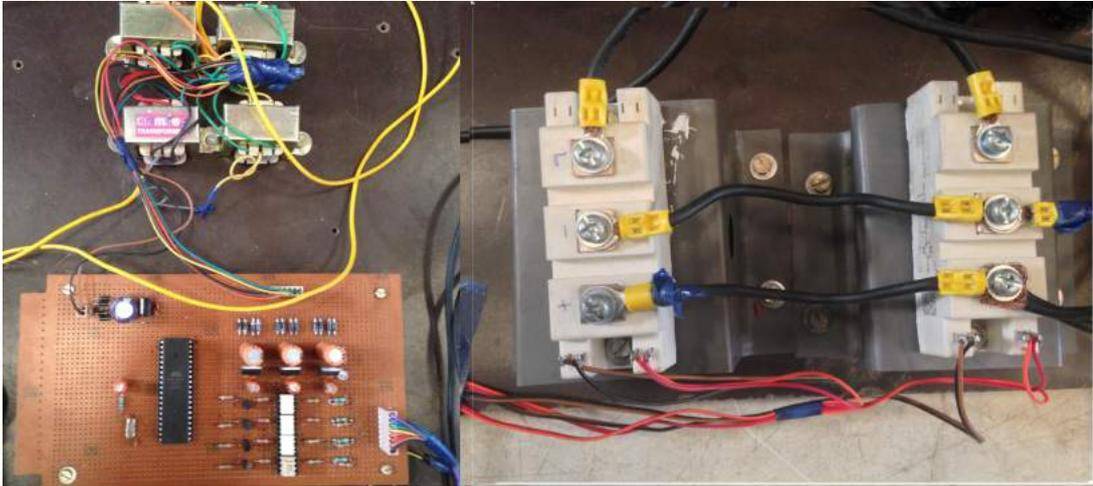
Figure 10.4: shows the hardware circuit of single phase inverter
