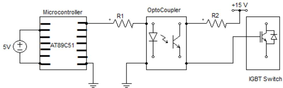
Figure 9.2: basic block diagram of gate driver circuit
