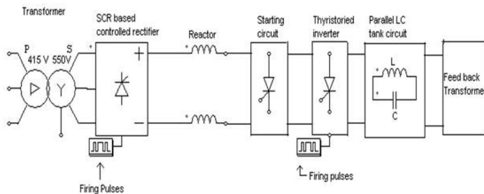
Figure 5.1: Power schematic of thyristorised based parallel resonance circuit configuration
