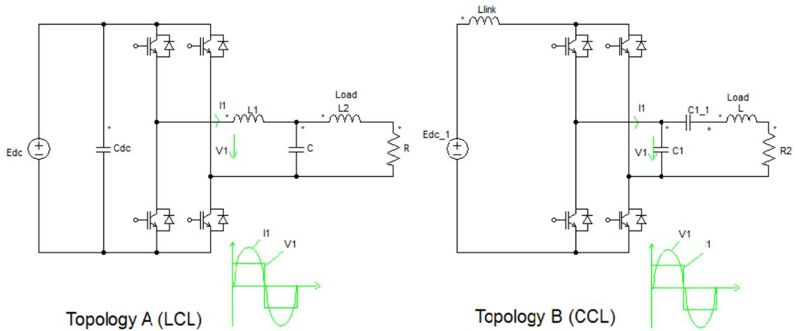
Figure 2.1: VSI with Inductive Coupling (topology A) and CSI with capacitive coupling (topology B) of the load
