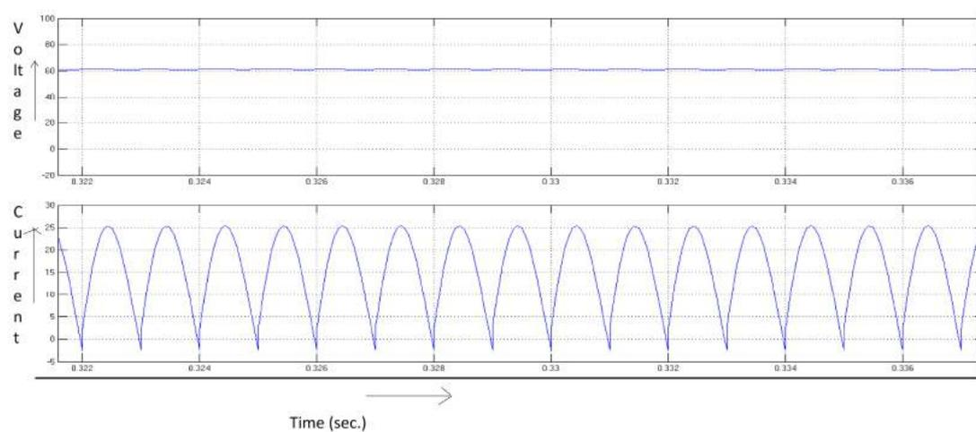
Figure 8.2: X-axis=Time(sec),Y-axis=1-Voltage,2-Current,DC link voltage and current
