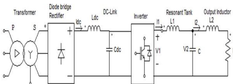
Figure 6.1: - shows the logical power schematic of IGBT based LCL resonant inverter with uncontrolled rectifier
