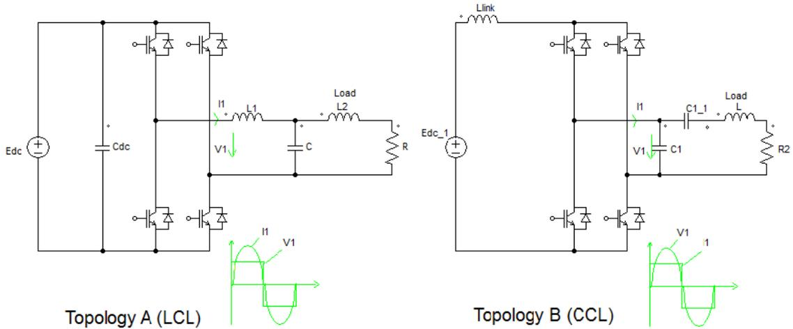
Figure 4.1: VSI with Inductive Coupling (topology A) and CSI with capacitive coupling (topology B) of the load
