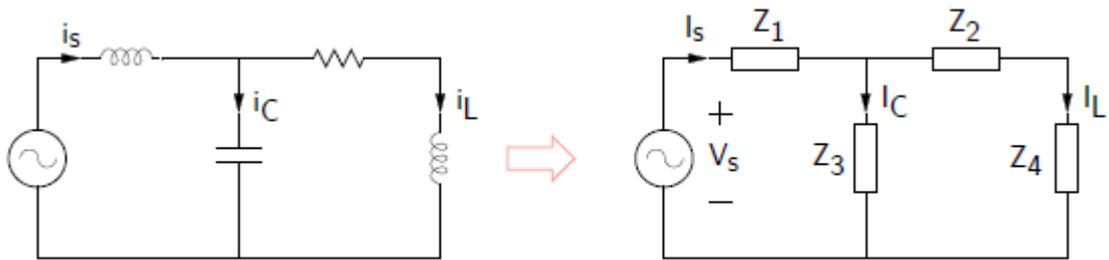
Figure 4.2: equivalent resonant-tank circuit
