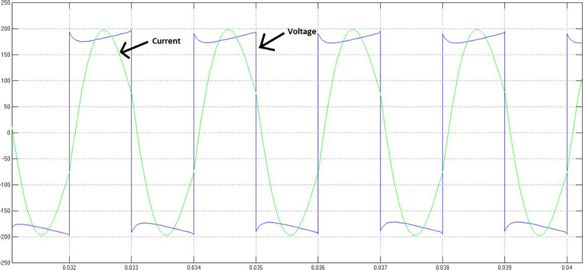
Figure 6.3: X-axis= Time (sec.), Y-axis= voltage, output voltage and current of the inverter
