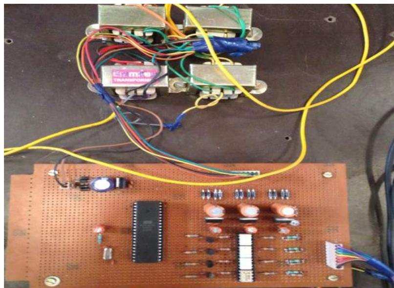
Figure 10.3: Gate driver hardware circuitry
