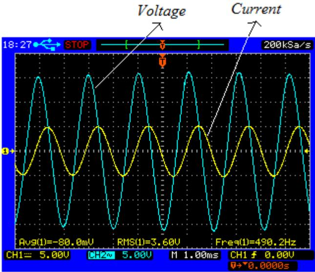
Figure 10.10: final output voltage and current at tank coil side when supplied voltage at Primary=83V, Sec.=10V and i/p current=0.7Amp and output voltage is 19V and Current is 1.5 amp.
