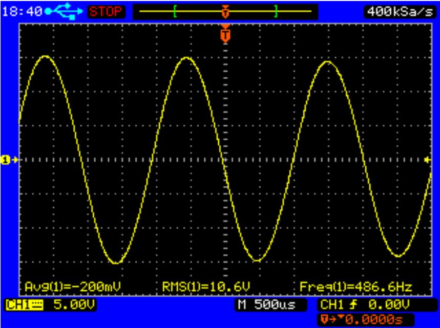
Figure 10.11: final output voltage at tank coil side when supplied voltage is 50V and i/p current=3.3 Amp and output voltage is 106V rms and Current is 8.7 Amp.
