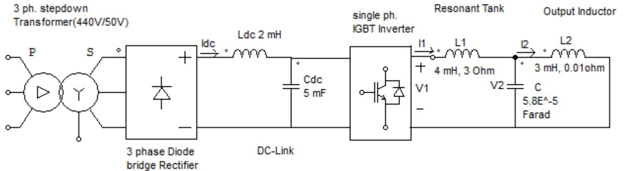
Figure 9.1: Power schematic of prototype design of LCL induction furnace
