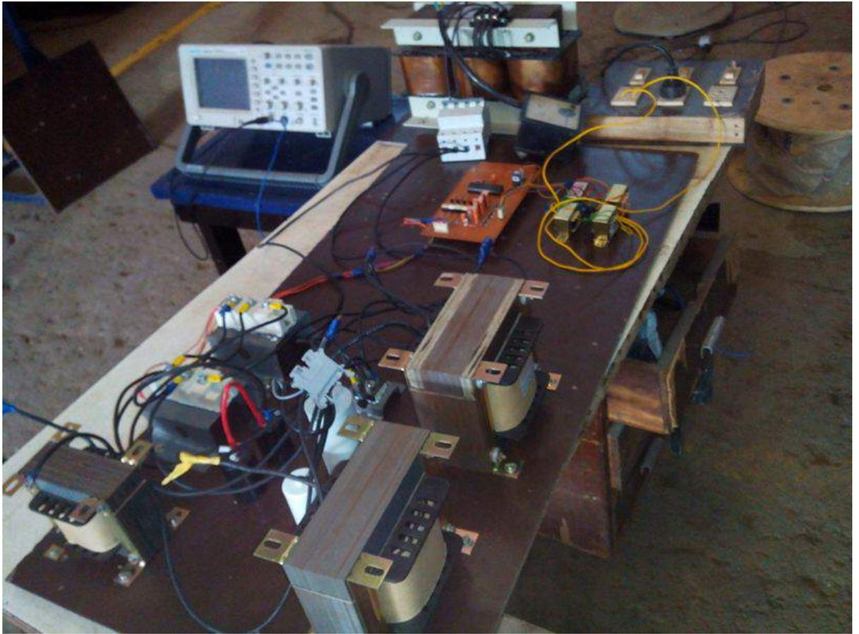
Figure 10.1: hardware setup of the LCL resonant converter
