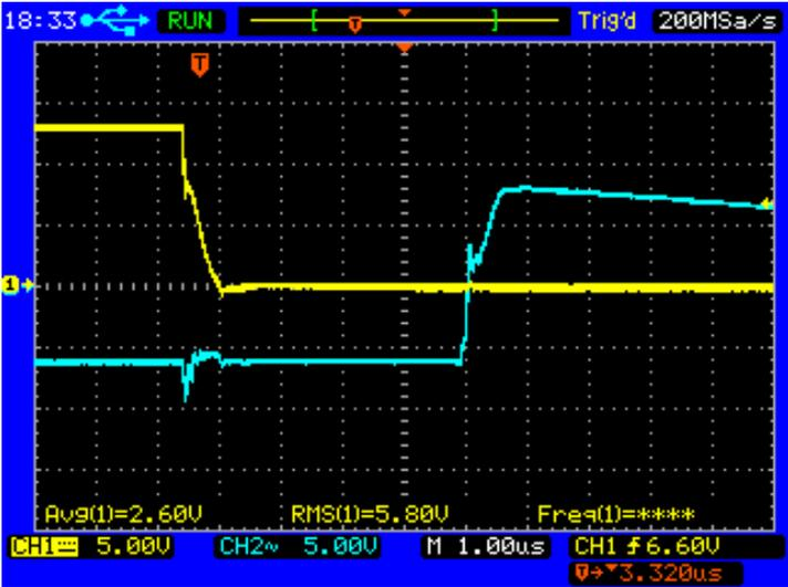
Figure 10.7: Dead band of 4 microsecond between two complimentary gating signal
