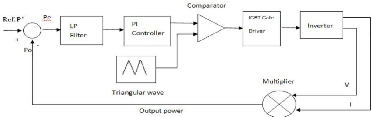
Figure 7.1: Block diagram for close loop control of inverter
