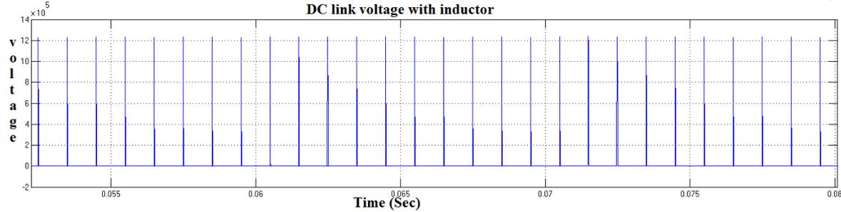
Figure 7.8: X-axis=Time(sec),Y-axis=Voltage,DC link voltage with inductor.
