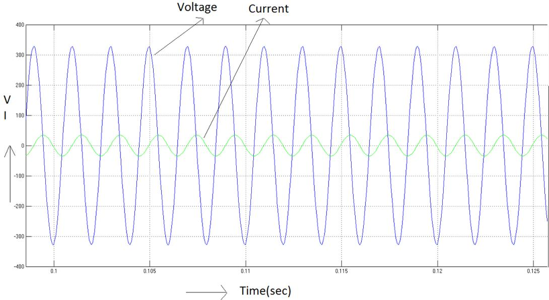
Figure 8.4: X-axis=Time(sec),Y-axis=Voltage and Current,output voltage and current at load 1kw load
