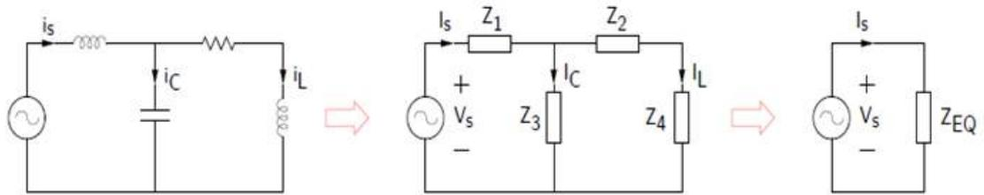
Figure 4.3: total system equivalent impedance.
