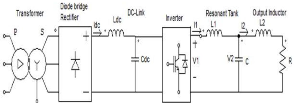
Figure 2.2: Power schematic of the IGBT based resonant inverter with LCL configuration
