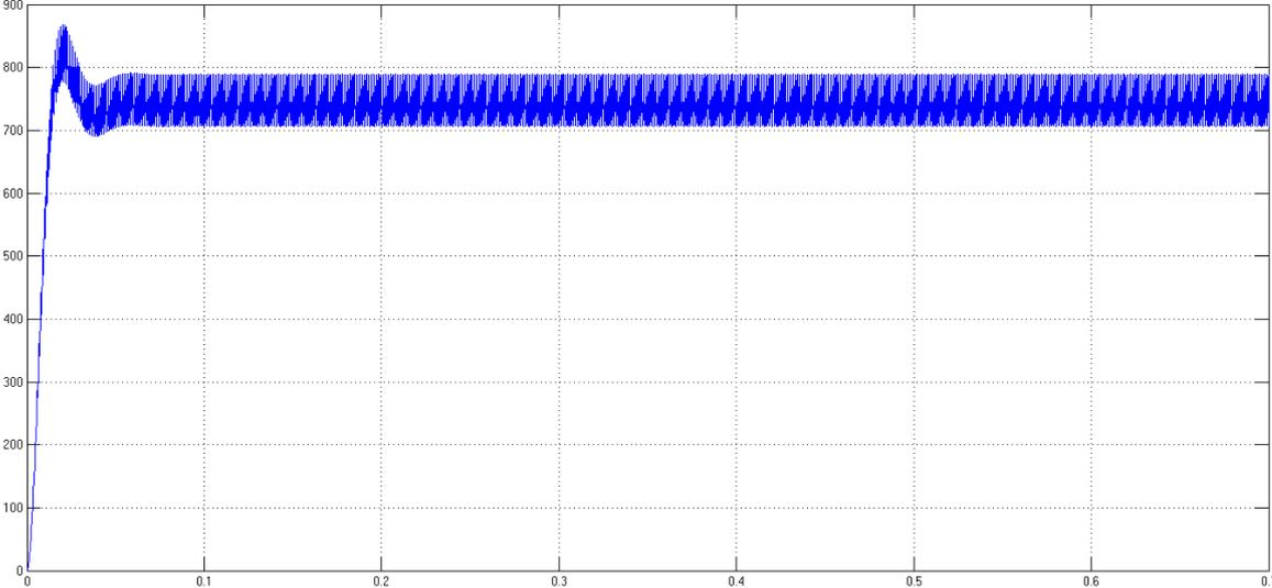
Figure 6.2: X-axis=Time(sec.),Y-axis= Voltage, Output voltage of DC link filter
