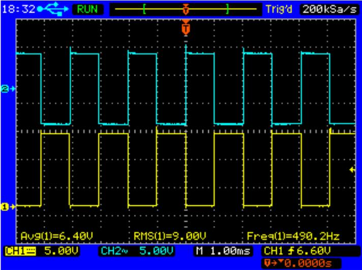
Figure 10.6: gate driver output for IGBT AH and AL
