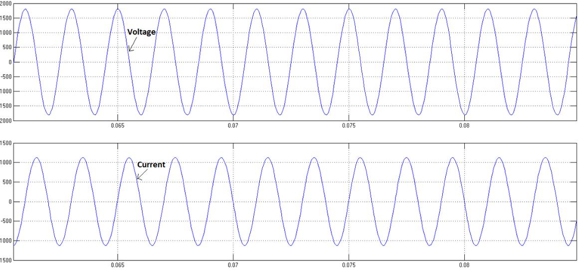
Figure 6.5: X-axis=Time(sec),Y-axis=1-Voltage,2-Current, shows the total output voltage current across the tank coil
