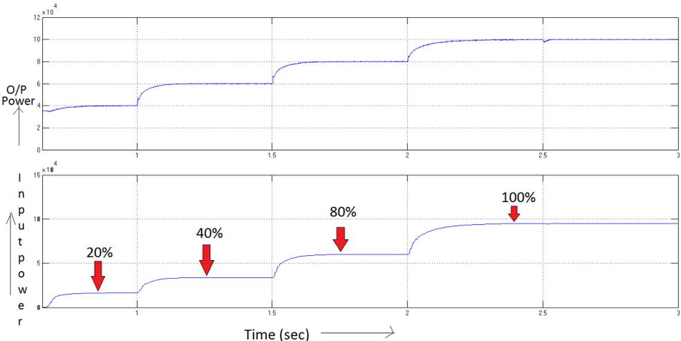
Figure 7.5: X-axis=Time(sec),Y-axis=1-output power,2-input power,variation in power w.r.t. to change in load.
