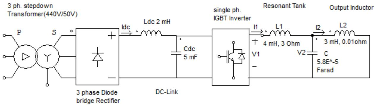
Figure 8.1: shows the power schematic of 1kW system with components rating
