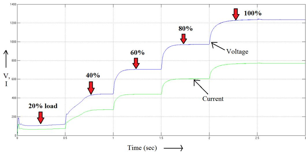
Figure 7.4: X-axis=Time(sec),Y-axis=Voltage and current,total system output w.r.t variation in load
