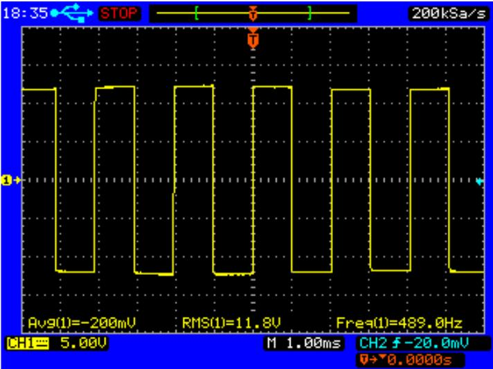
Figure 10.8: inverter output voltage with R load.
