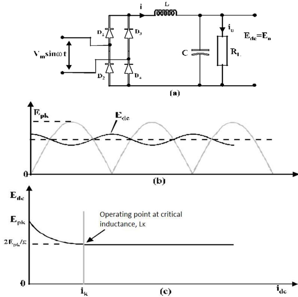
Figure 3.1: Full wave rectifier with inductor input filter (a) rectifier-LC filter circuit, output voltage waveform,(c) output voltage versus load.
