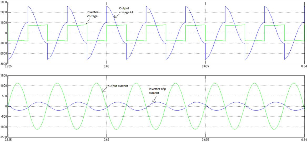
Figure 6.4: X-axis=Time(sec),Y-axis=1 voltage,2-current, output voltage and current across the inductor L1
