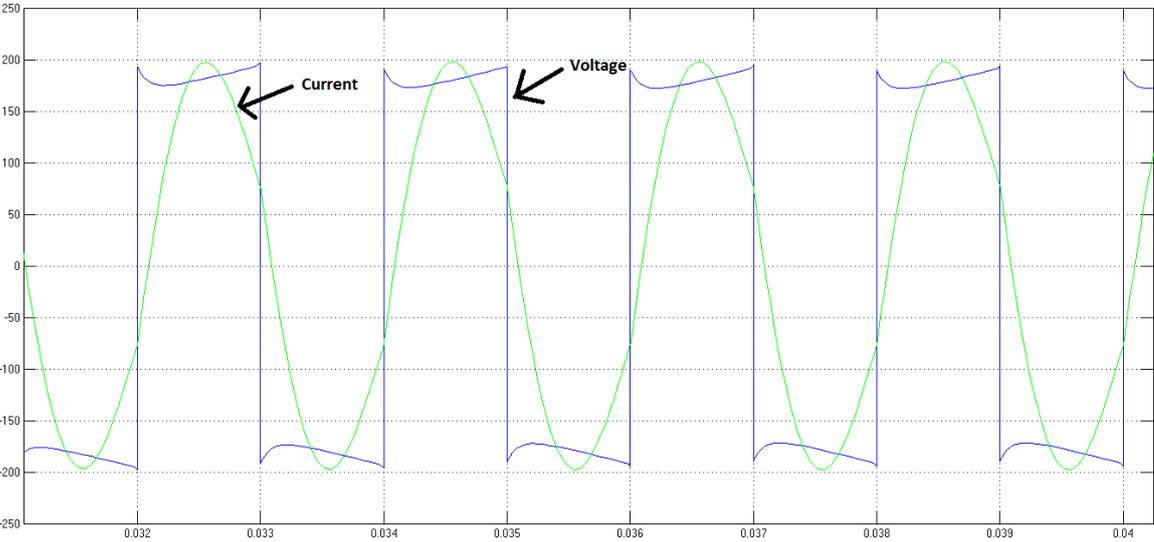
Figure 7.7: X-axis=Time(sec),Y-axis=Voltage and Current,Desired output of inverter waveform shape at each load irrespective of load variation.
