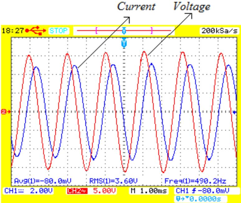
Figure 10.9: final output voltage and current at tank coil side when supplied voltage at Primary=83V, Sec.=10V and i/p current=0.7Amp and output voltage is 19V and Current is 1.5 amp.
