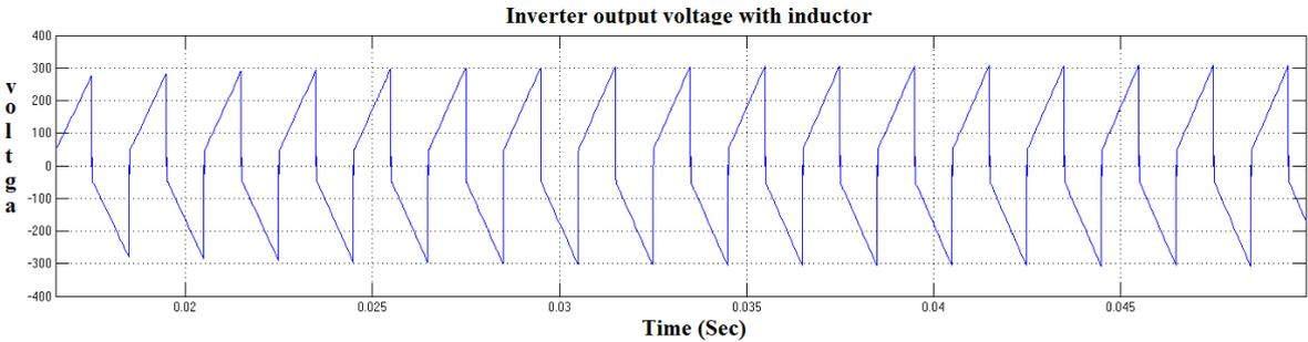
Figure 7.9: X-axis=Time(sec),Y-axis=Voltage,inverter output voltage with inductor.
