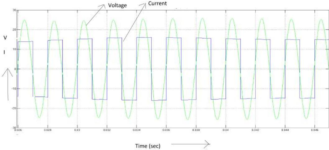
Figure 8.3: X-axis=Time(sec),Y-axis=Voltage and Current,inverter output voltage and current at 1kW
