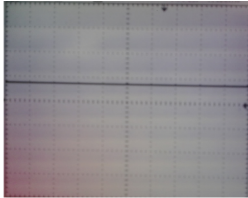
Figure 6.14: Constant Dc output scale x axis:1 cm = 5 millisecond, y axis:1 cm = 5 Volt.
