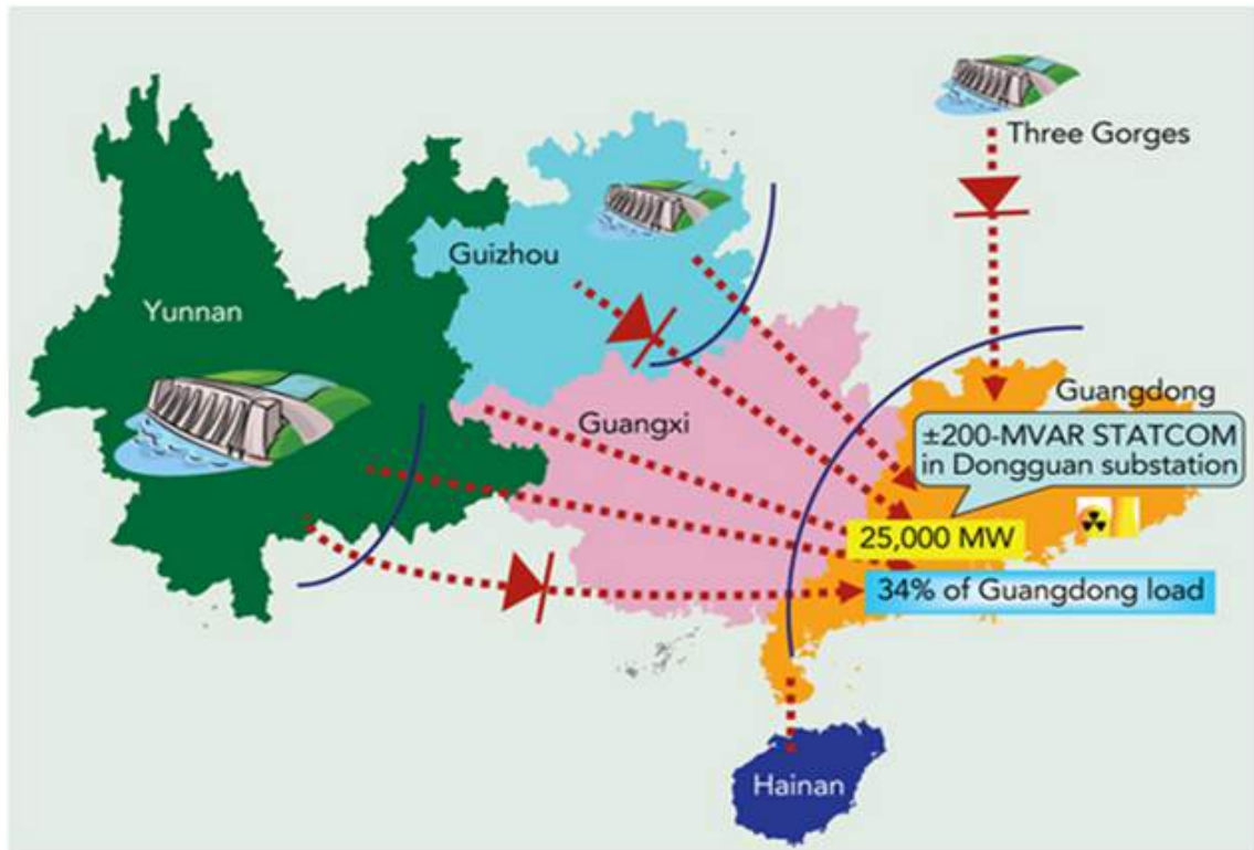
Figure 3.10: China Southern Power Grid service area and STATCOM location
