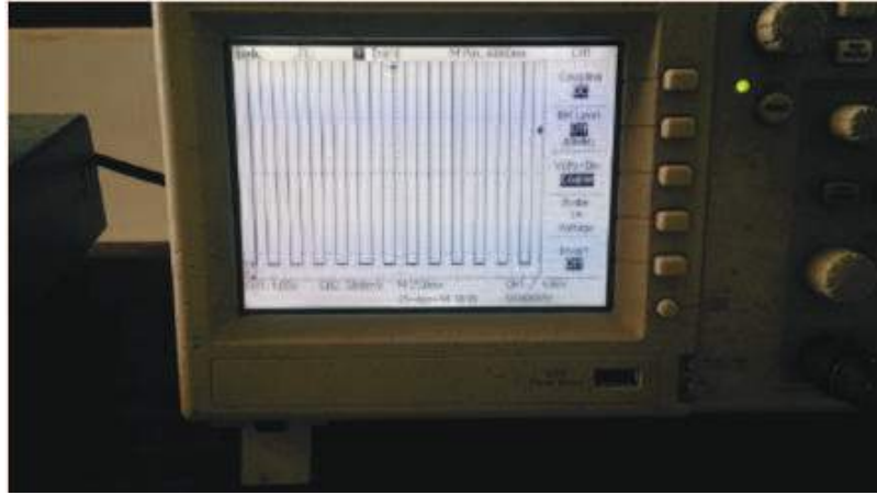
Figure 9.9: MOSFET Triggering Pulses[Scale:X-axis:10ms,Y-axis:5 V/div]
