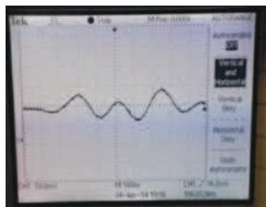
Figure 9.15: Output Voltage Waveforms Of Thyristor[Scale:X-axis:10ms,Y-axis:5 V/div]
