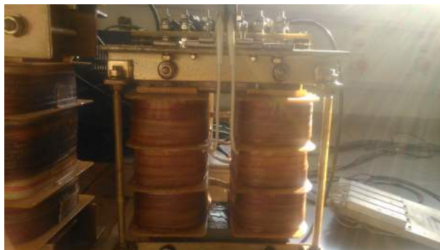
Figure 8.3: 9 kVA Active Interphase Transformer
