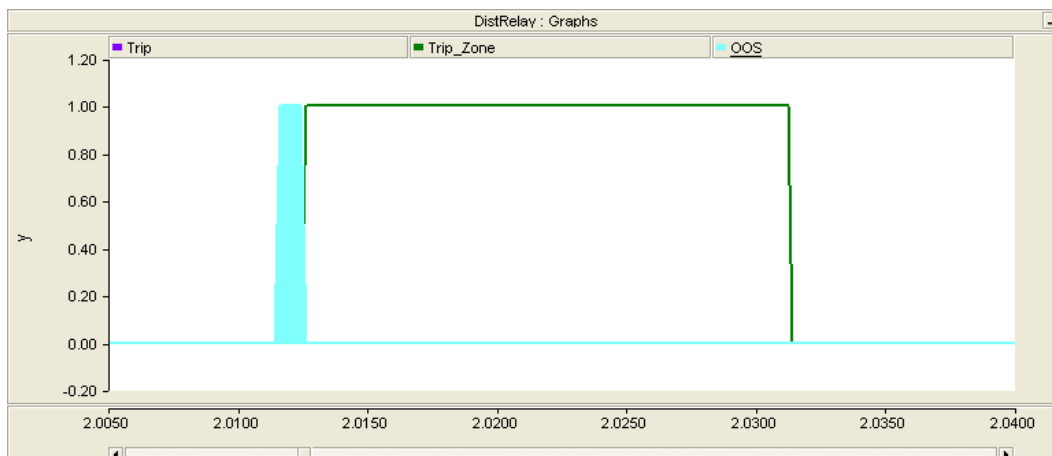
Figure 5.8: Tripping Logic when fault is created at 100 kms
