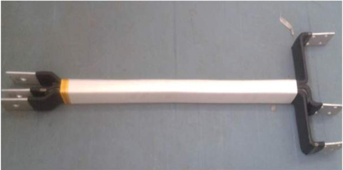
Figure 5.8: Bus bar with glass mica epoxy along with conducting tape before curing
