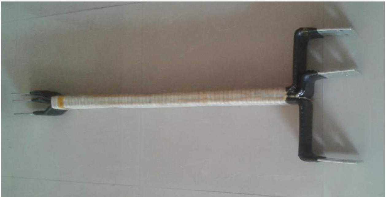
Figure 5.9: Bus bar with insulation material after curing
