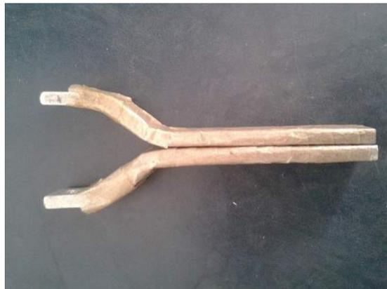
Figure 5.3: Glass mica epoxy tape model
