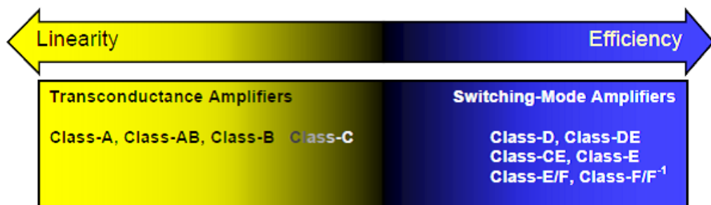
Figure 3.3: Transconductance and switching-mode amplifiers
