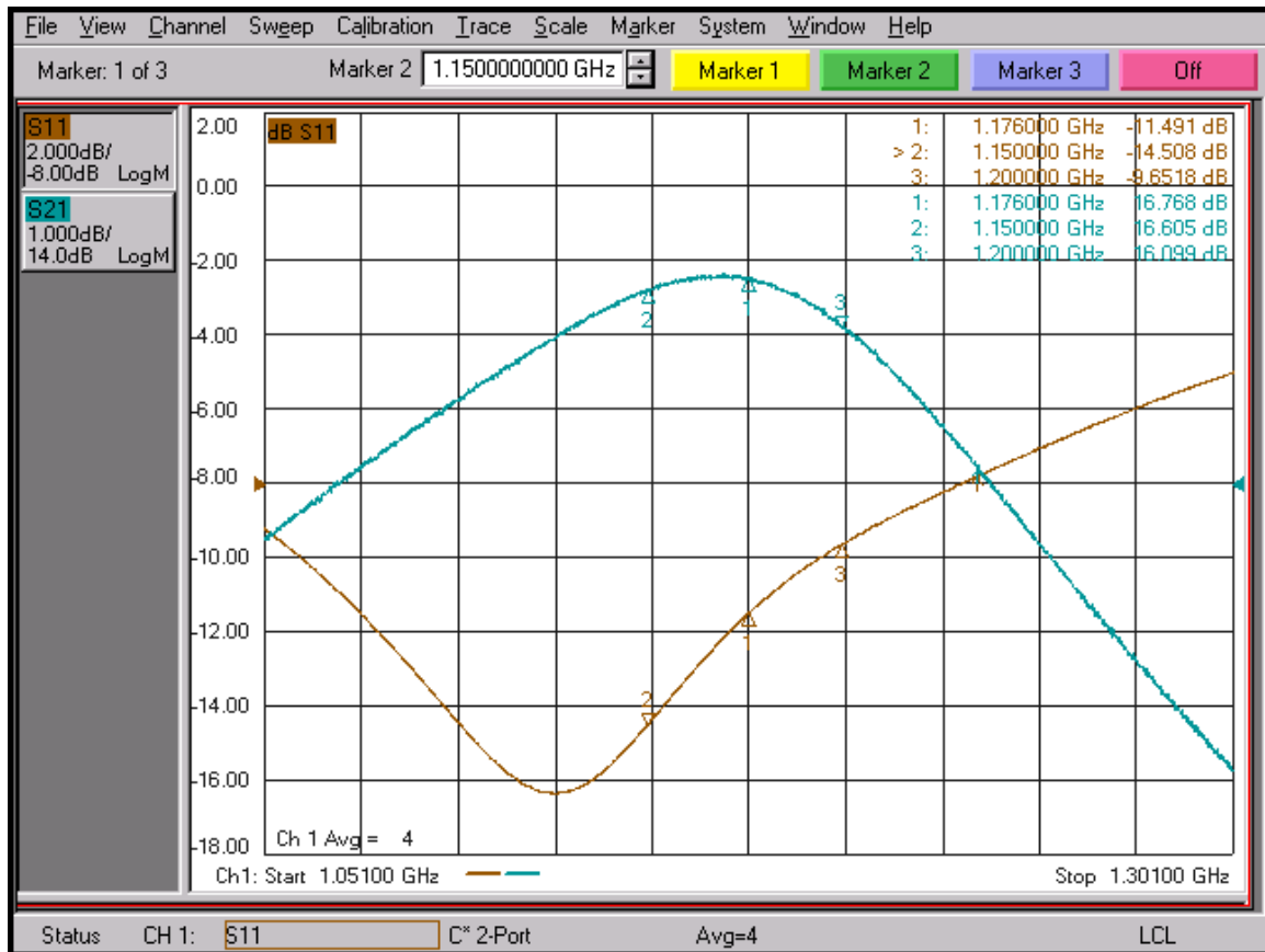
Figure 5.8: S(2,1) from Network Analyzer
