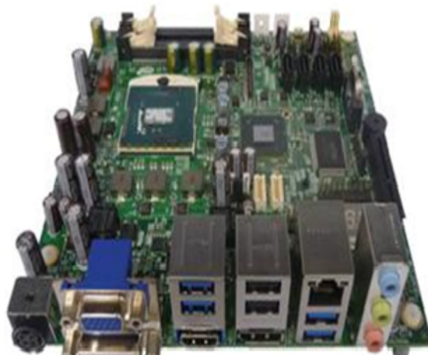
Figure 1.3: Example of RVP/CRB Board-Intel ® Core ™ i5-3610ME processor (PGA) and mobile Intel ® QM77 Express Chipset development kit
