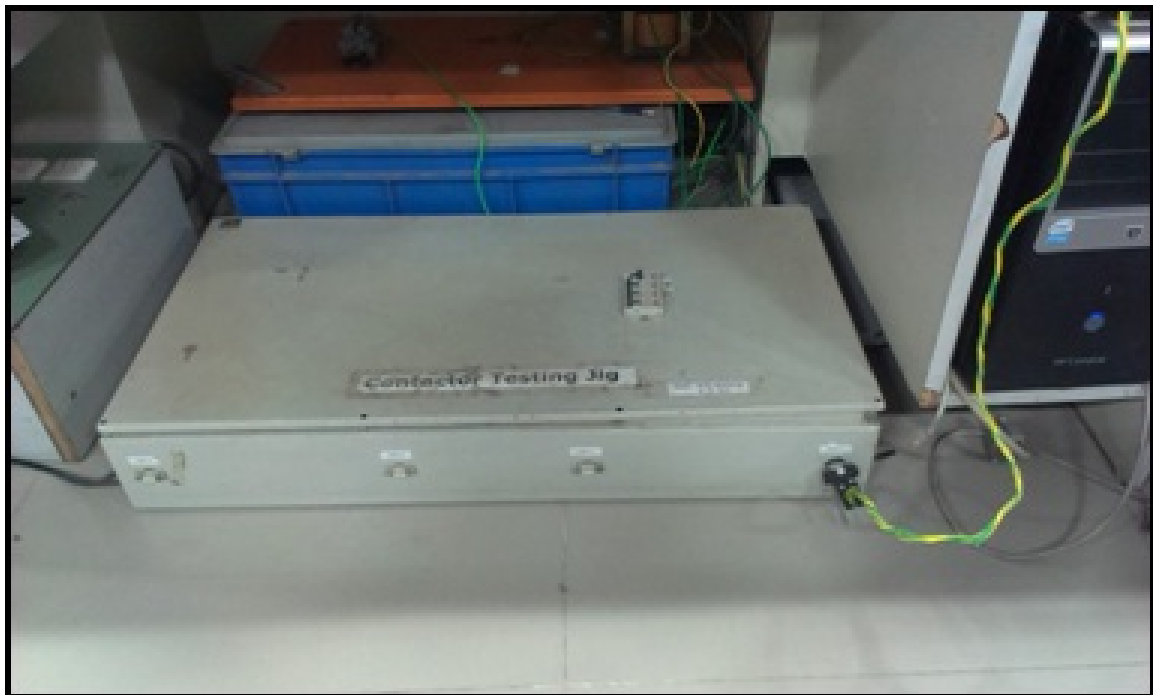
Figure 3.13: Snapshot of contactor testing jig consist of heater for Industrial Process test
