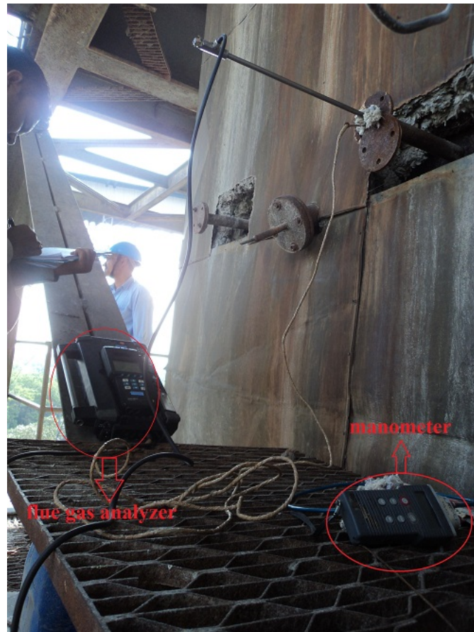
Figure 4.6: Set up of APH Audit
