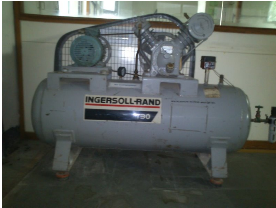
Figure 3.3: Two stage v-type compressor with inter cooler
