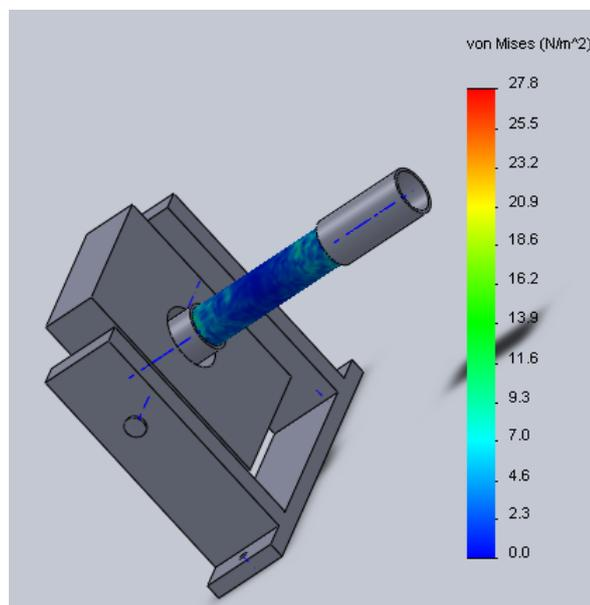
Figure 5.11: Von-mises stress of shaft
