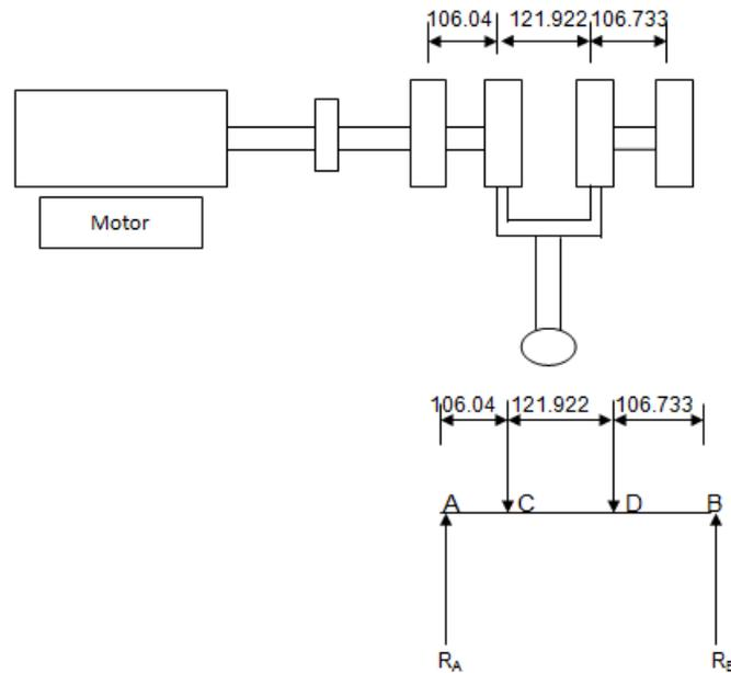
Figure 4.1: Beam analysis of machine set up
