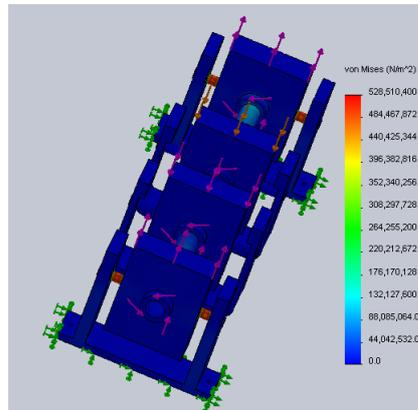
Figure 5.15: Von mises stress
