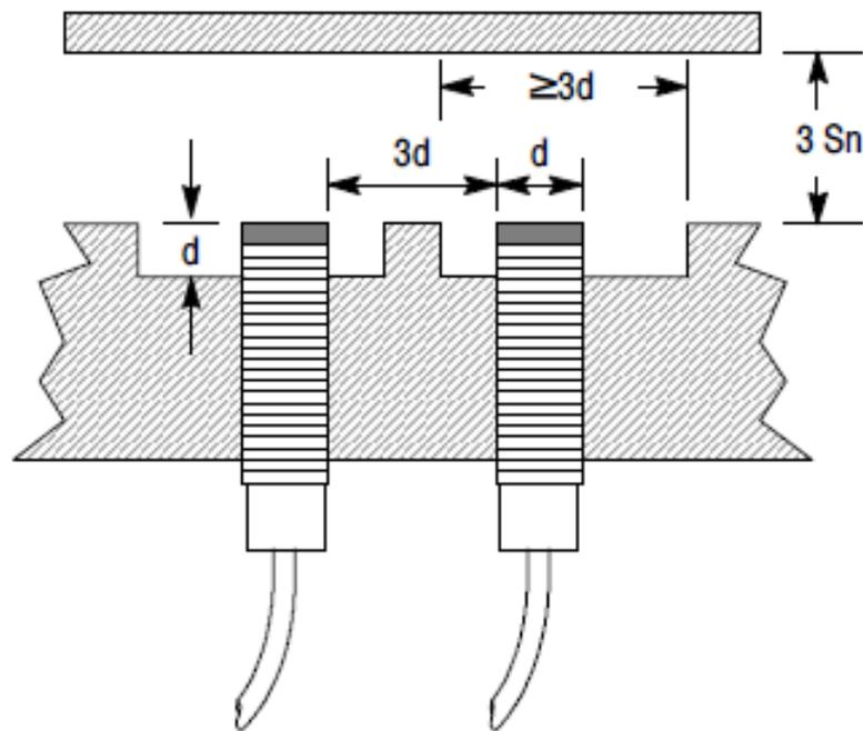
Figure 4.3: Two inductive proximity sensor for long specimen
