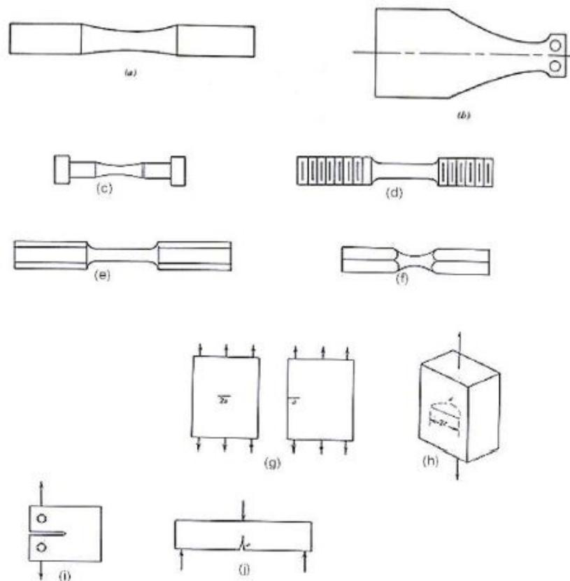
Figure 1.5: Test Specimens: (a) Rotating bending, (b) Cantilever Flat Sheet (c) Buttoned axial dog-bone, (d) Threaded axial dog-bone, (e) torsion, (f) Combined stress, (g) Axial Cracked sheet, (h) Part-through crack, (i) Compact tension and (j) Three point bend specimen
