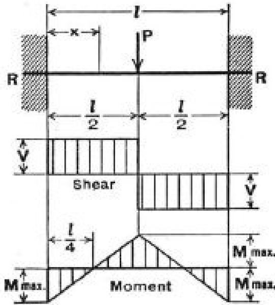
Figure 3.1: Bending Moment diagram of simply supported beam
