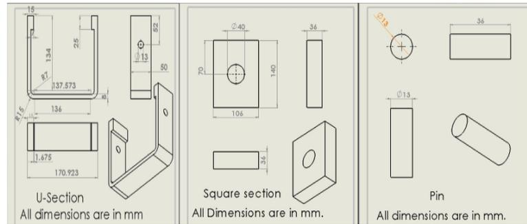
Figure 5.7: Detailed drawing of U-Section, Square Section and Pin
