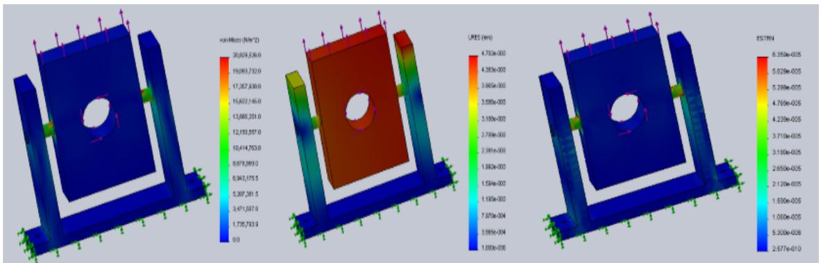
Figure 5.6: Von-mises stress, Displacement and Strain of C-Section and square section
