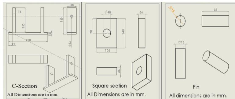
Figure 5.3: Detailed drawing of C-Section, Square Section and Pin
