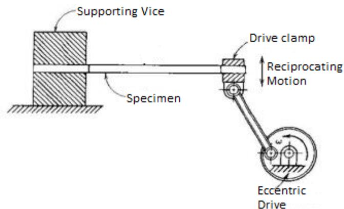
Figure 1.2: Reciprocating Type Bending Testing Machine
