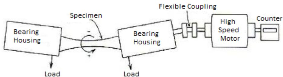
Figure 1.1: Rotating Type Bending Testing Machine
