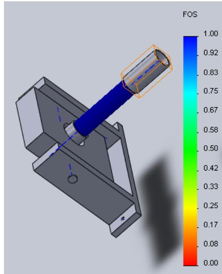
Figure 5.12: Factor of safety of whole machine set-up
