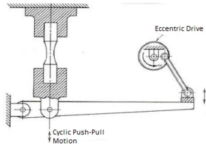
Figure 1.3: Direct-Force Fatigue Testing Machine [1]
