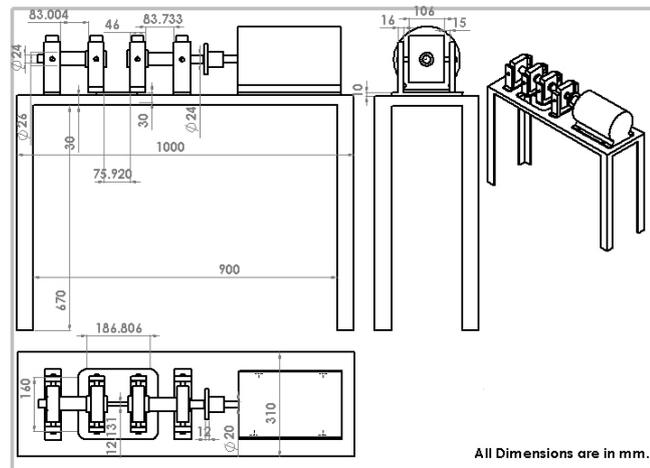
Figure 5.2: Detail drawing of machine set-up
