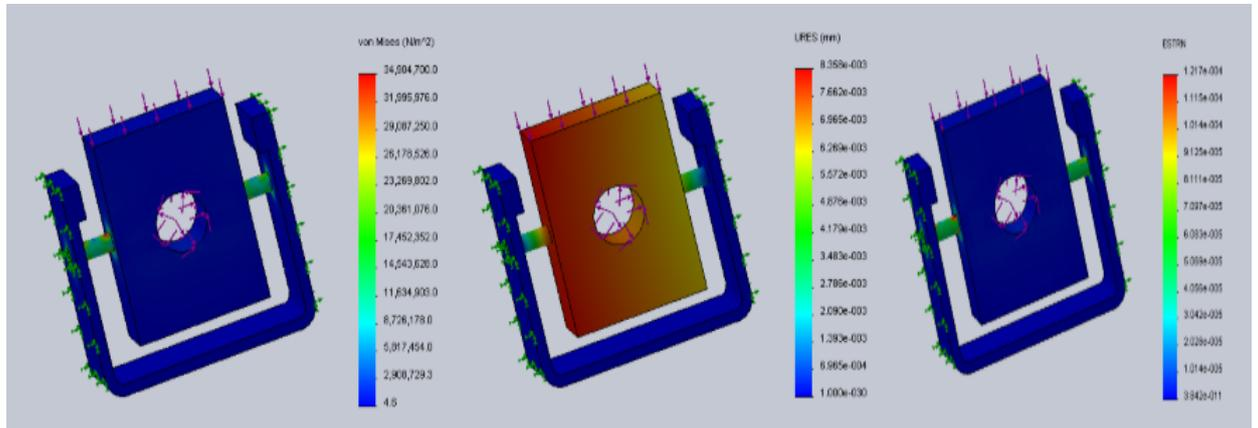
Figure 5.10: Von-mises stress, Displacement and Strain of U-Section and square section
