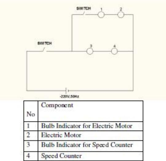
Figure 4.6: Electric circuit diagram
