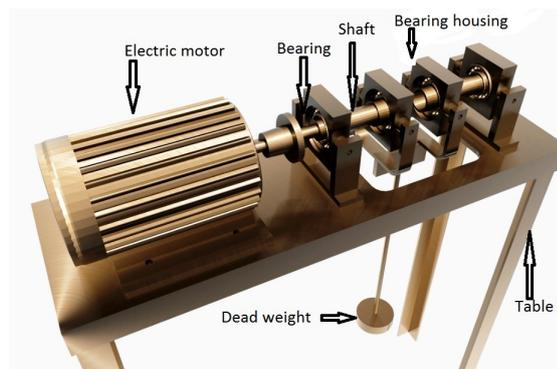
Figure 5.1: CAD model of machine set-up
