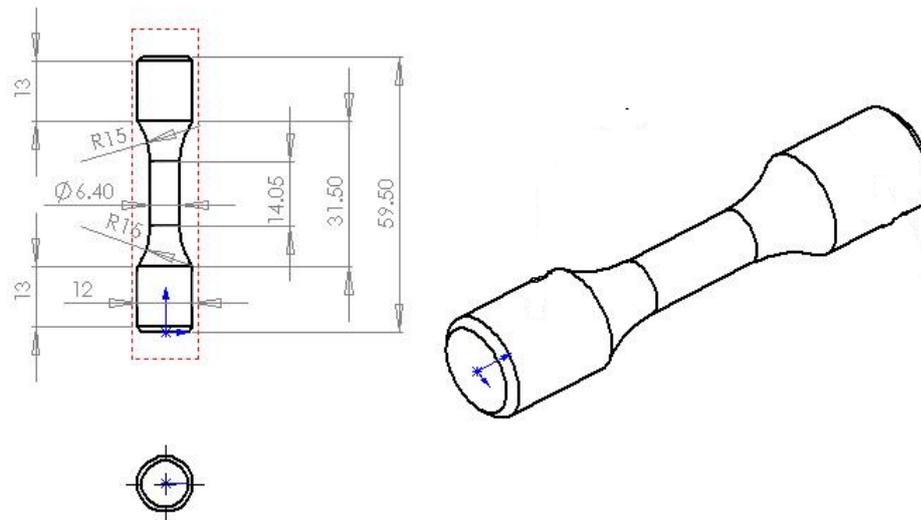
Figure 1.6: Test Specimens
