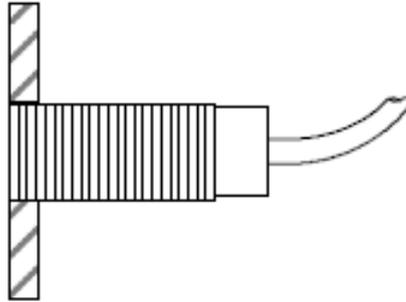
Figure 4.2: Side view of Proximity sensor
