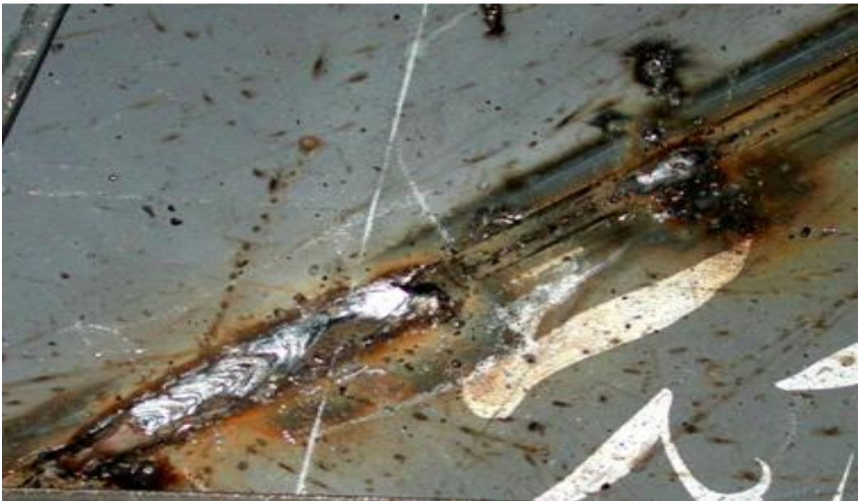
Fig.11 Defect in continuous welding in overhead position.
