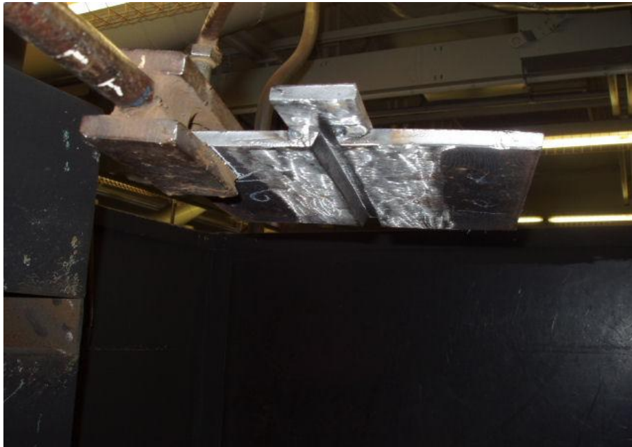
Fig.8 setup for overhead welding.
