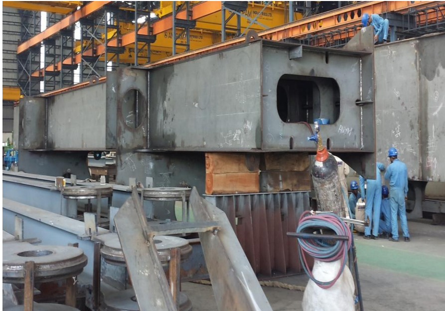
Fig.4 (box section of overhead crane)
