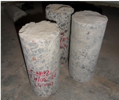
Figure 4.14: Extracted core specimen
