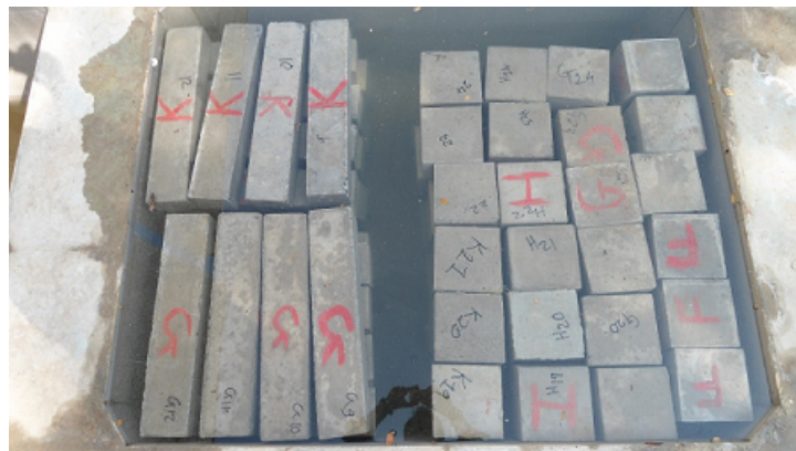
Figure 4.10: Concrete specimens in water tank for water permeability test
