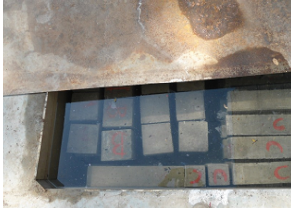
Figure 4.8: Tank of chloride solution with concrete specimens
