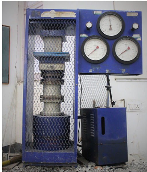
Figure 4.5: Plain concrete cube in compression testing machine
