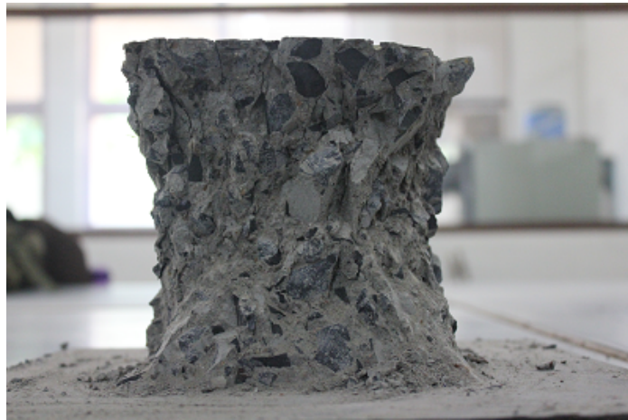
Figure 5.1: Failure of Plain Concrete Cube After Compression Test
