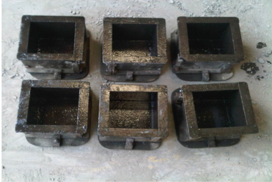
Figure 4.1: Moulds for concrete specimens
