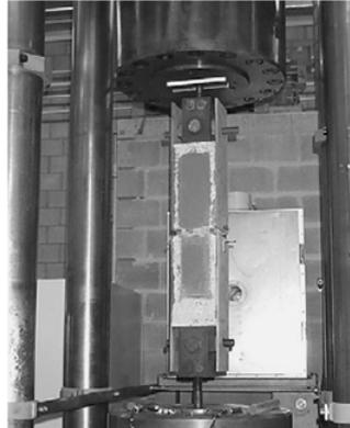
Figure 2.1: Test Setup for Direct Tension
