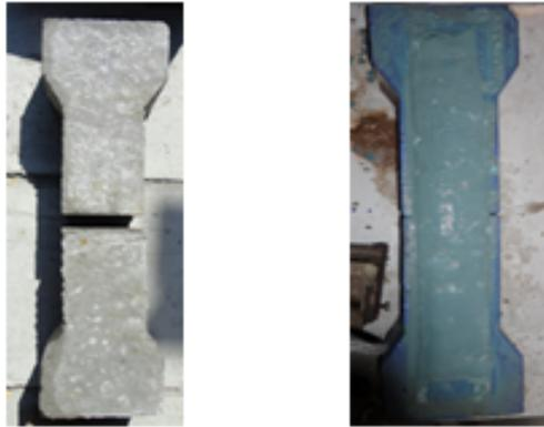
Figure 3.7: Casted Concrete Specimen (Left) and SFRG Coated Specimen (Right)
