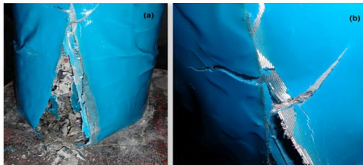
Figure 4.21: (a) and (b) Failure of Circular R.C.C Epoxy SSWM Layer 2
