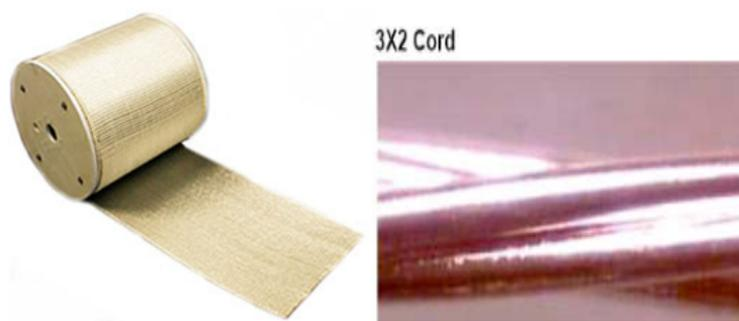
Figure 1.2: (a) SFRP Material of Hardwire (b) Steel Cord of SFRP
