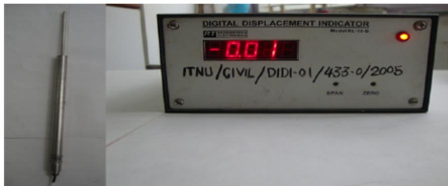
Figure 3.30: LVDT Rod and Digital Indicator
