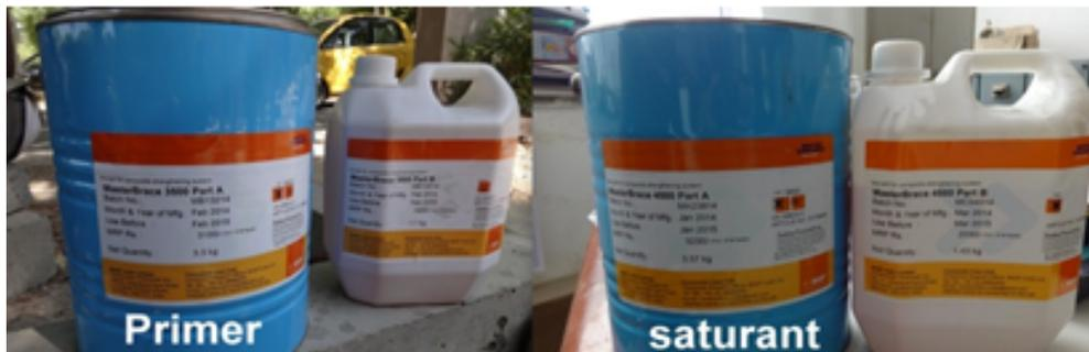
Figure 3.21: Primer (Part 1 and 2) and Saturant (Part 1 and 2)
