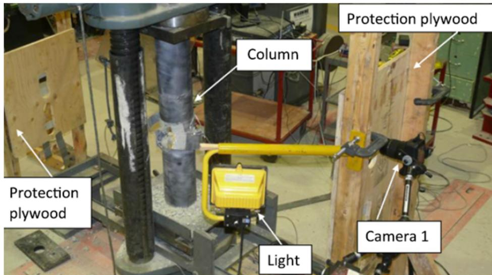
Figure 2.6: Test Setup for Concrete Specimens
