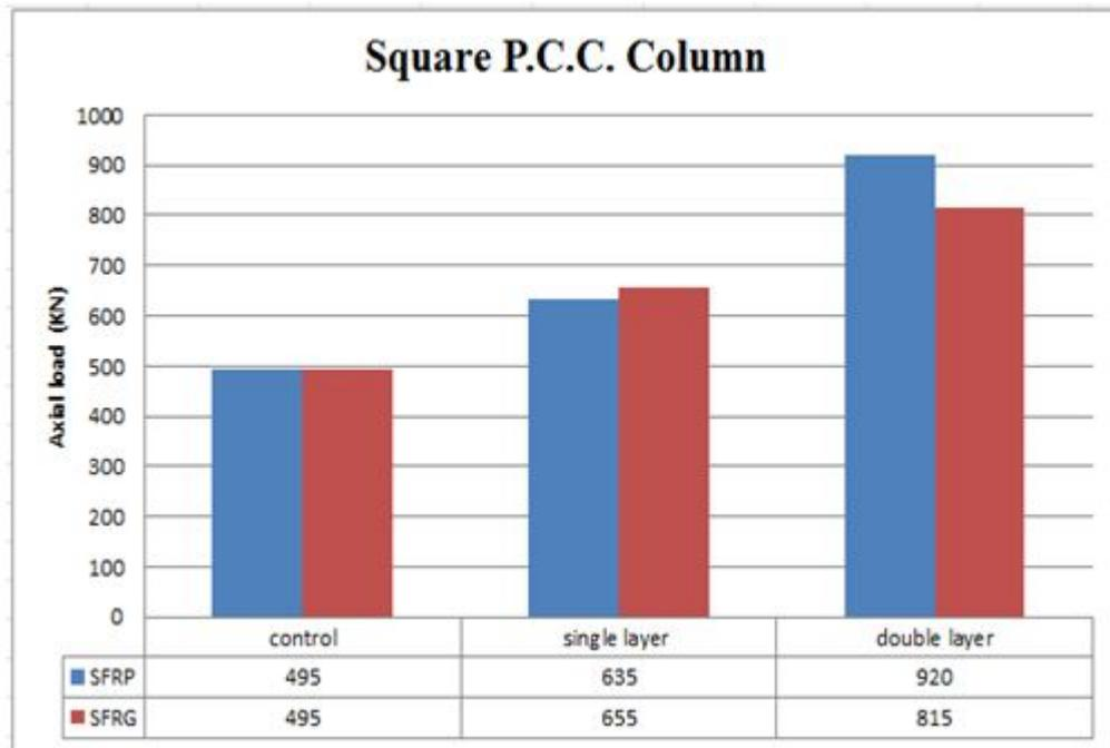
Figure 4.3: Comparison of Axial Load of Square Column
