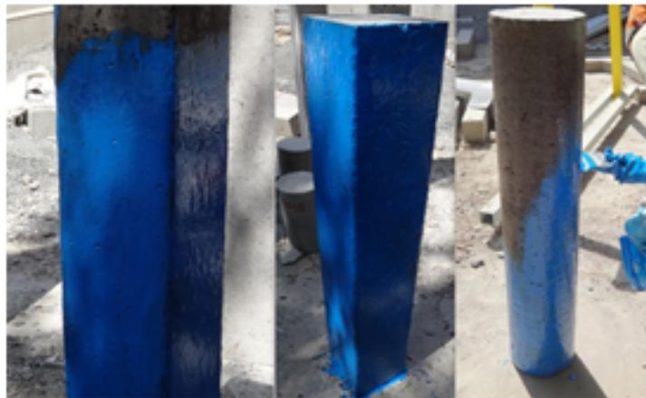
Figure 3.24: Applying First Coat of Epoxy
