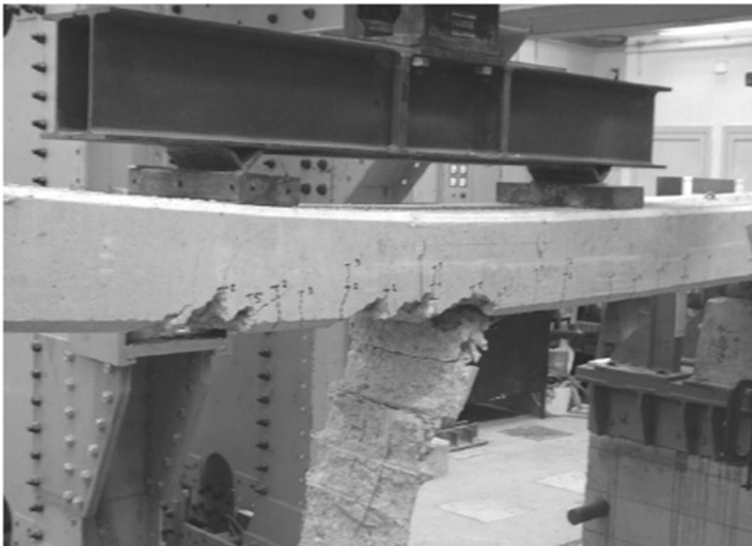
Figure 2.9: Lateral View of Failure of Beam
