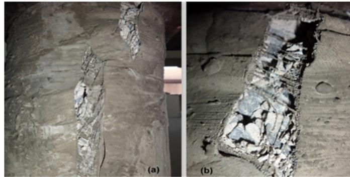
Figure 4.26: (a) and (b) Failure of Circular P.C.C Polymer SSWM Layer 2
