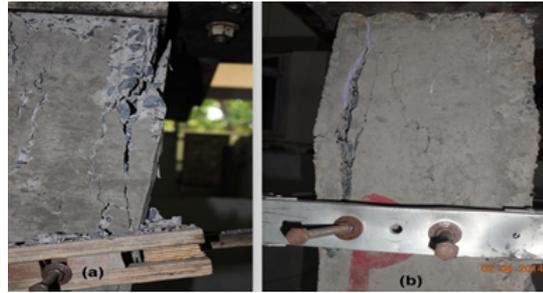
Figure 4.18: (a) and (b) Failure of Control Square P.C.C.
