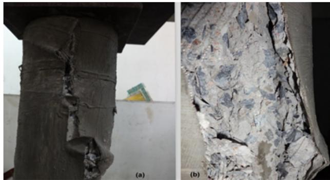
Figure 4.27: (a) and (b) Failure of Circular R.C.C Polymer SSWM Layer 2
