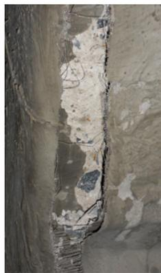
Figure 4.29: Failure of Square P.C.C. Polymer SSWM Layer 2
