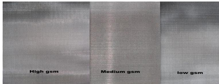
Figure 1.3: Three Types of Steel Wire Mesh
