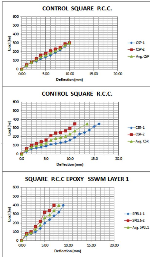
Figure 4.8: Load vs. Deflection of CSP, CSR and SPEL1 Columns
