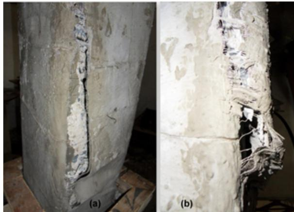
Figure 4.30: (a) and (b) Failure of Square R.C.C. Polymer SSWM Layer 2
