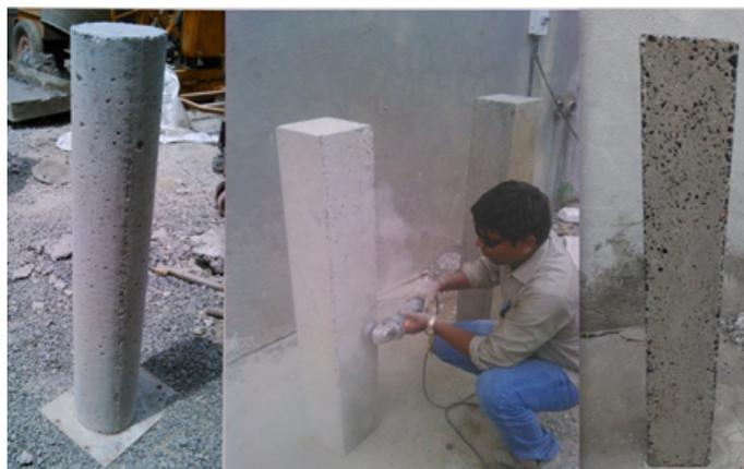
Figure 3.14: Grinding of Specimens
