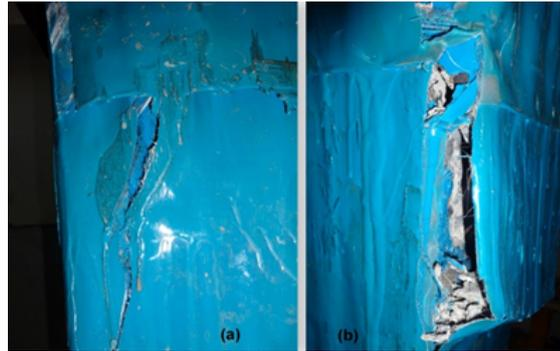
Figure 4.24: (a) and (b) Failure of Square R.C.C. Epoxy SSWM Layer 2
