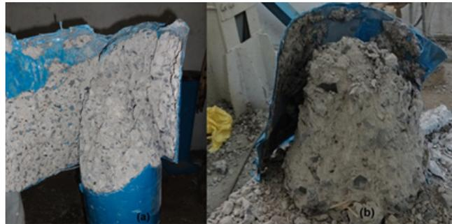
Figure 4.20: (a) and (b) Failure of Circular P.C.C Epoxy SSWM Layer 2
