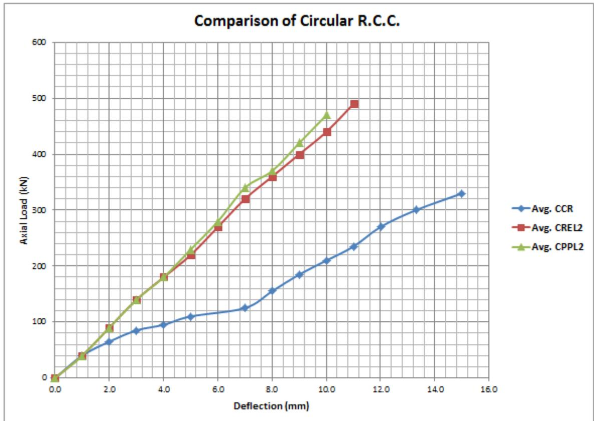
Figure 4.12: Load vs. Deflection of Circular R.C.C. Columns
