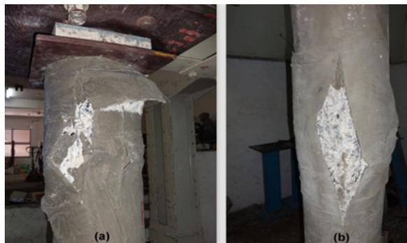
Figure 4.25: (a) and (b) Failure of Circular P.C.C Polymer SSWM Layer 1
