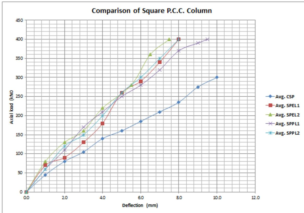
Figure 4.13: Load vs. Deflection of Square P.C.C. Columns
