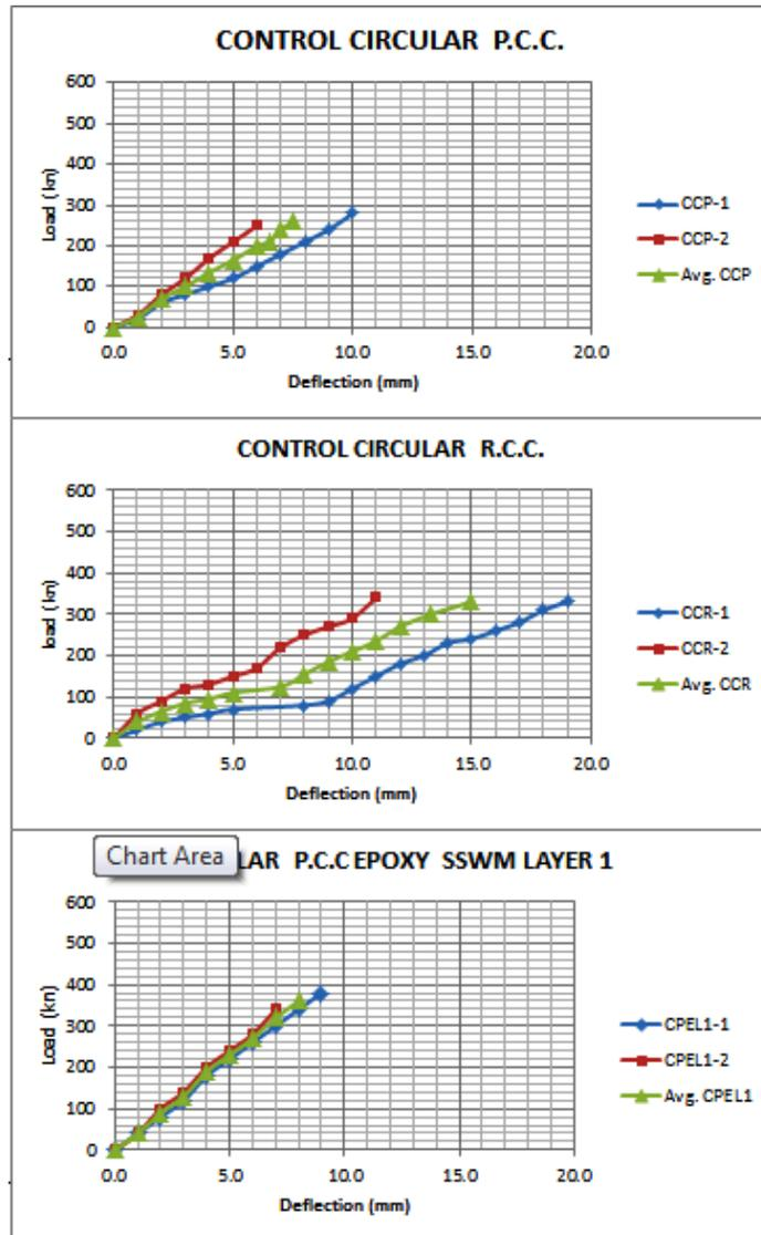
Figure 4.5: Load vs. Deflection of CCP, CCR and CPEL1 Columns
