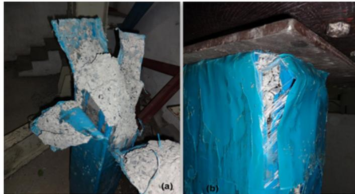
Figure 4.22: (a) and (b) Failure of Square P.C.C. Epoxy SSWM Layer 1
