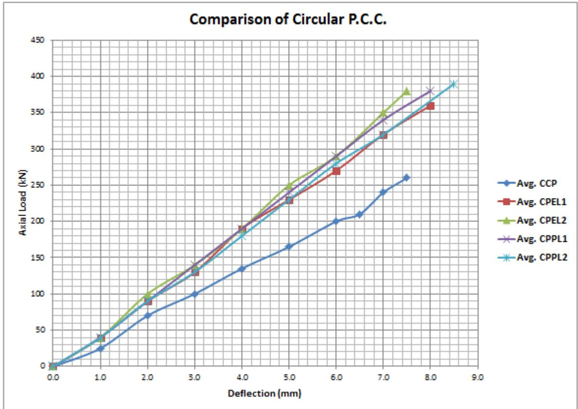
Figure 4.11: Load vs. Deflection of Circular P.C.C. Columns
