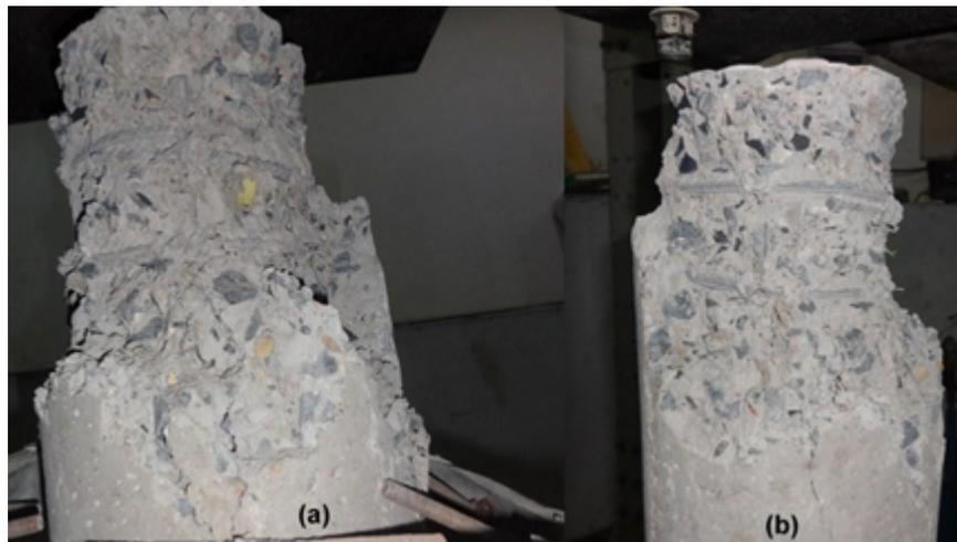
Figure 4.15: (a) and (b) Failure of Circular Column R.C.C.
