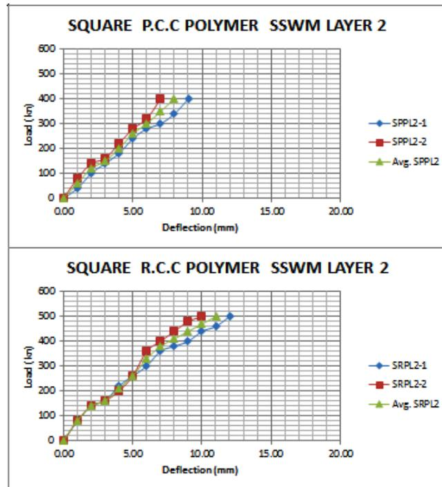
Figure 4.10: Load vs. Deflection of SPPL2 and SRPL2 Columns
