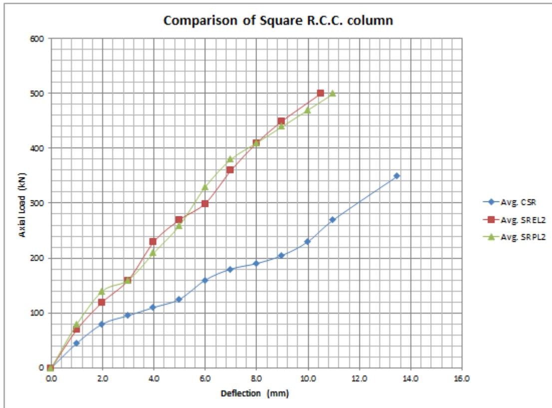
Figure 4.14: Load vs. Deflection of Square R.C.C. Columns
