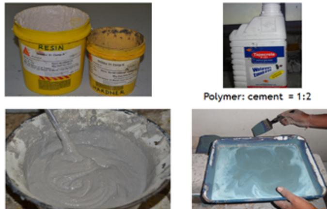
Figure 3.5: Epoxy Resin (Sikadur-31)(Left) and Cementitious Polymer Grout (Tapecreate P-151)(Right)
