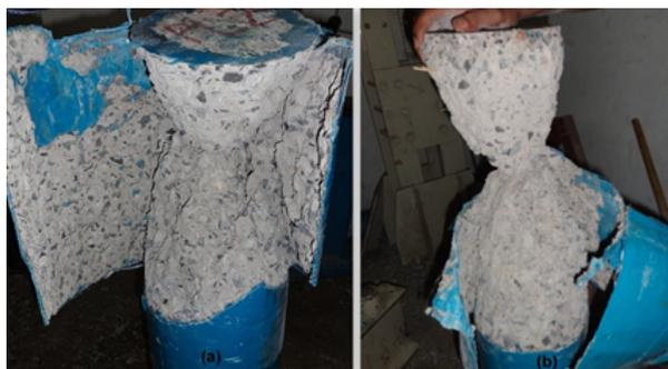
Figure 4.19: (a) and (b) Failure of Circular P.C.C Epoxy SSWM Layer 1
