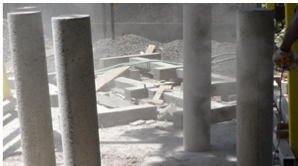
Figure 3.20: Grinding of Columns
