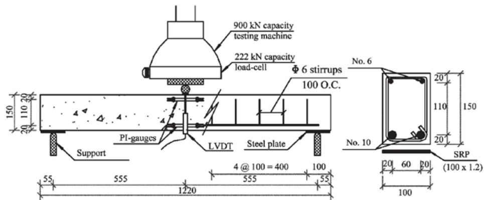
Figure 2.8: Experimental Test Setup and Beam Detail
