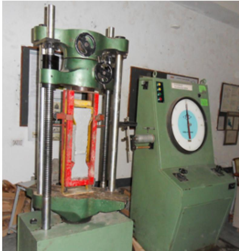
Figure 3.9: Test Setup of Bond Test
