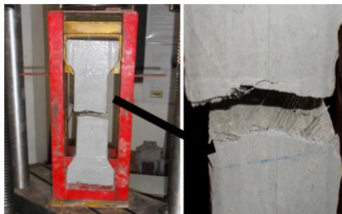
Figure 3.10: Failure of Bond Specimen
