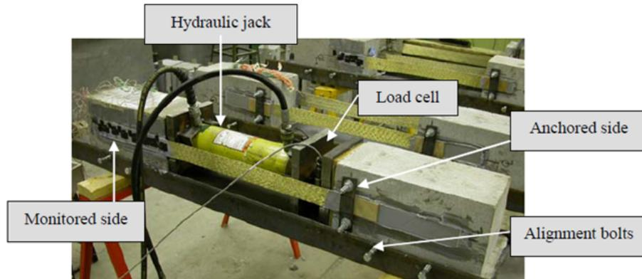
Figure 2.3: Test Setup for Direct Shear Test
