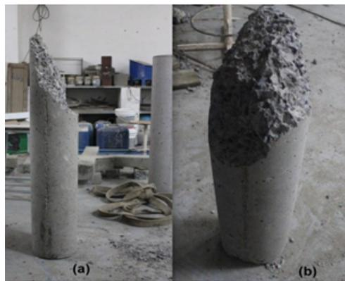
Figure 4.16: (a) and (b) Failure of Circular Column P.C.C.
