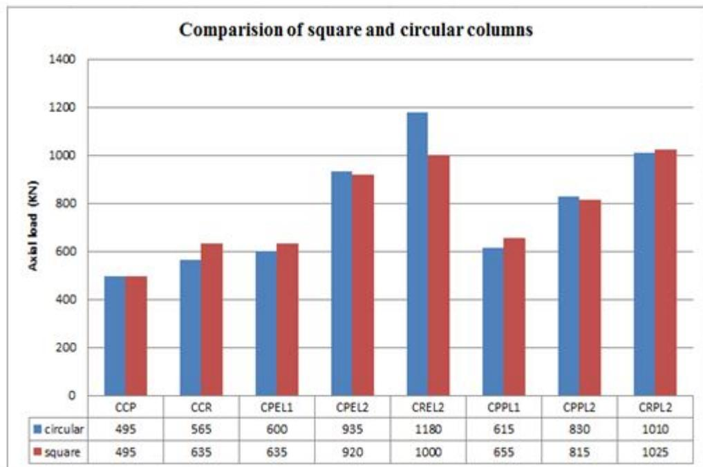
Figure 4.4: Comparison of Axial Load of Square and Circular Columns
