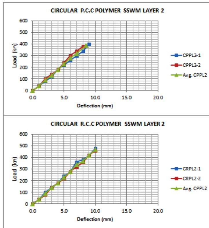
Figure 4.7: Load vs. Deflection of CPPL2 and CRPL2 columns
