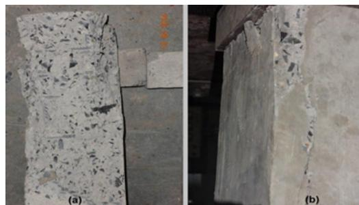
Figure 4.17: (a) and (b) Failure of Control Square R.C.C.
