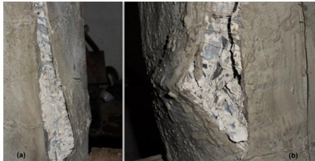
Figure 4.28: (a) and (b) Failure of Square P.C.C. Polymer SSWM Layer 1
