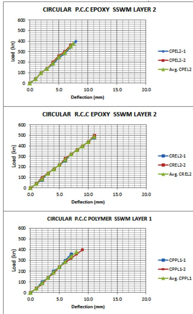
Figure 4.6: Load vs. Deflection of CPEL2, CREL2 and CPPL1 Columns
