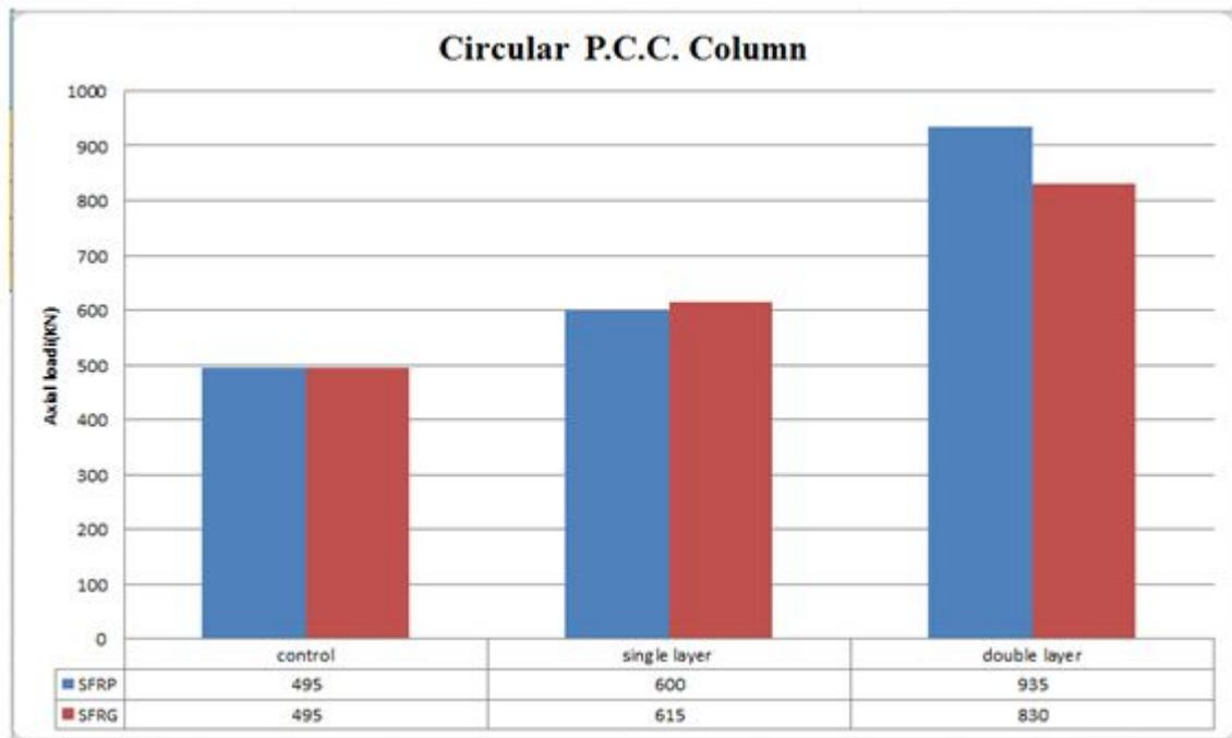
Figure 4.2: Comparison of Axial Load of Circular Column
