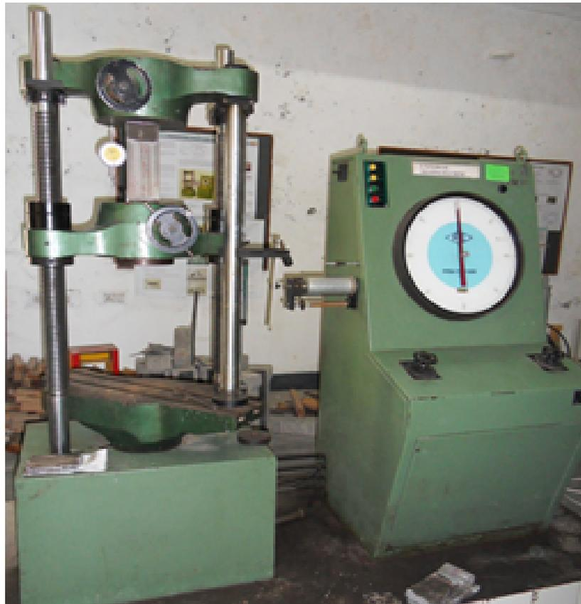
Figure 3.3: Test Setup for Tensile Test
