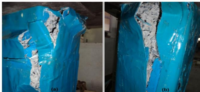
Figure 4.23: (a) and (b) Failure of Square P.C.C. Epoxy SSWM Layer 2
