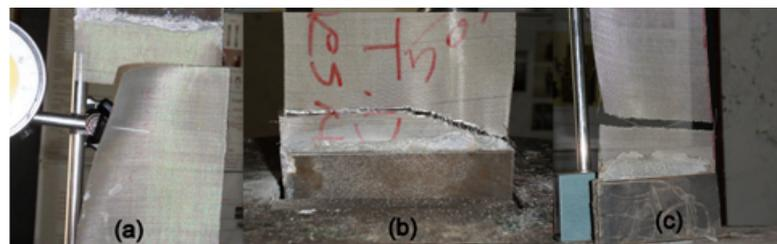
Figure 3.4: (a) Failure of SSWM-1 (b) Failure of SSWM-2 (c) Failure of SSWM-3
