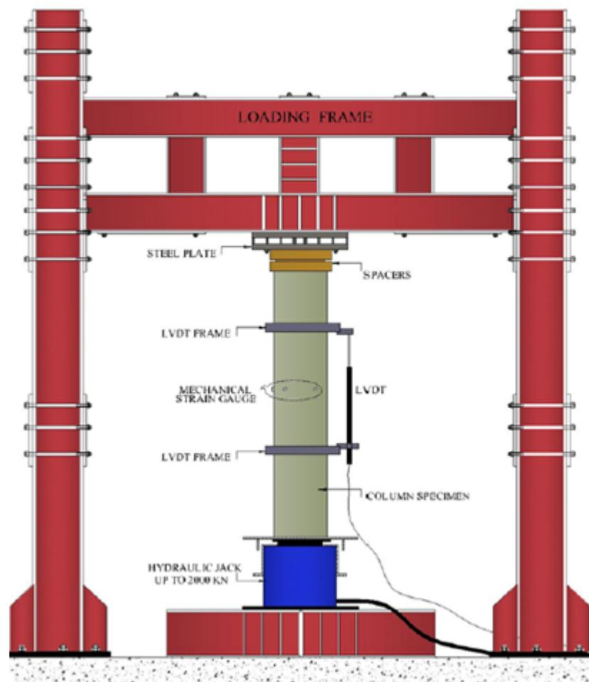
Figure 3.29: Test Setup for Column Specimen
