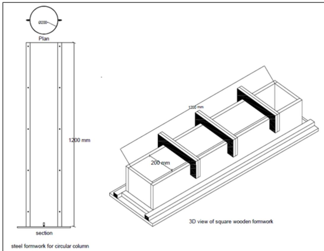
Figure 3.11: Drawing of Formwork
