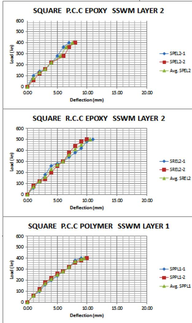
Figure 4.9: Load vs. Deflection of SPEL2, SREL2 and SPPL1 Columns
